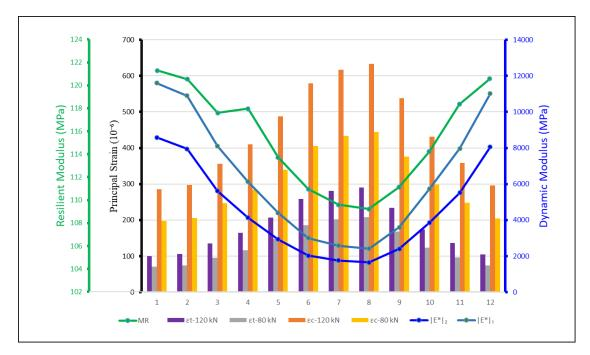
Figure 4.2 Principal strains and material properties
