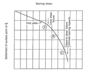
Figure 5.1 Load-Settlement curve (Modified from Whitman and Hoeg, 1966)
