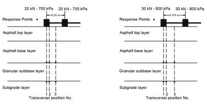
Figure 4.1 Evaluated response points and two reference axles
