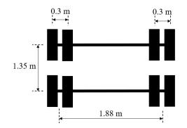
Figure 7.3 The heaviest axle configuration in solar farm
