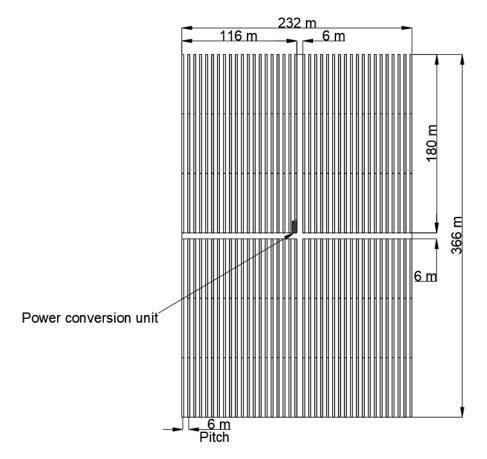
Figure 6.11 10 5MW array block showing location of PCU and access track
