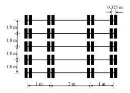
Figure 7.4 The heaviest axle load configuration in wind farm
