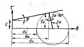
Figure 5.6 Shear and normal stresses in a plane stress state (ODN 218.046-01, 2001)
