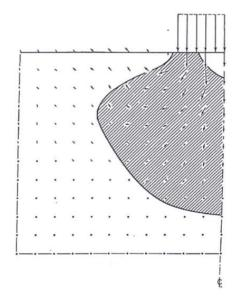
Figure 5.4 Plastic zone reaching the foundation surface (Whitman and Hoeg, 1966)
