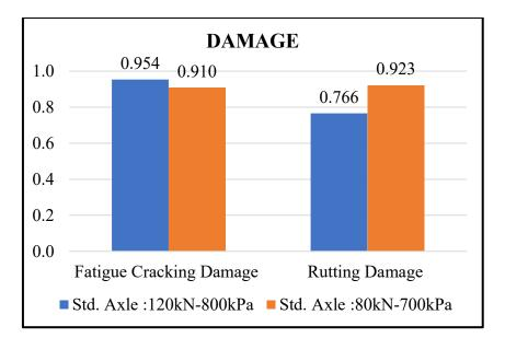
Figure 4.3 Comparison of damages
