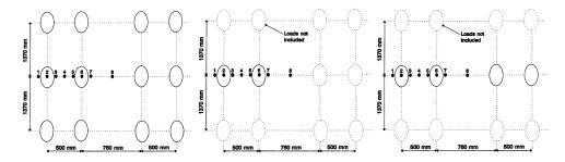
Figure 2.8 Triple, single axle load and dual wheel load (From left to right) (Jooste and Fernando, 1995)
