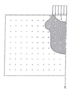
Figure 5.3 Propagation of the plastic zone (Whitman and Hoeg, 1966)
