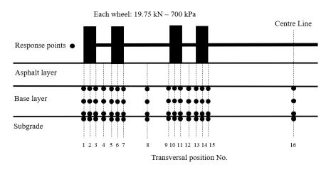
Figure 7.9 Evaluated response points within pavement - Wind farm
