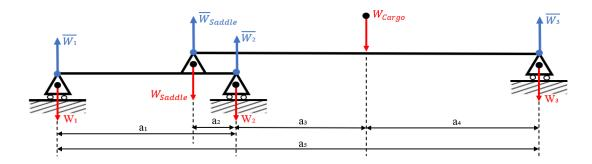
Figure 6.21 Computational static model of flatbed trailer
