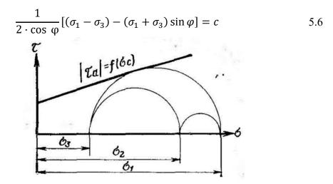
Figure 5.7 Mohr diagram under volumetric stress state (ODN 218.046-01, 2001)
