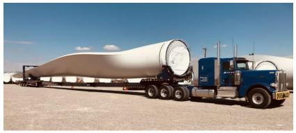
Source: Wind Energy Transport LLC Figure 1.5 Turbine blade transport in wind farm
