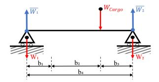
Figure 6.26 Computational model of dump truck
