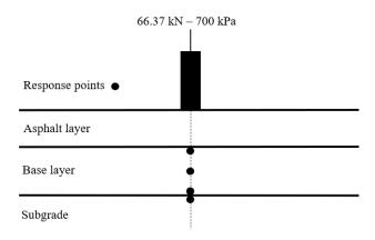
Figure 7.7 Evaluation points in the pavement under ESWL
