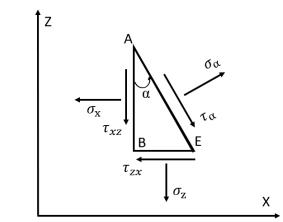
Figure 5.9 Stress components on segment ABE
