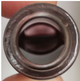
Figure 53. Resin sample of A/IB 60:40 charged with 5% in weight of WPL-CF after 4 hours
