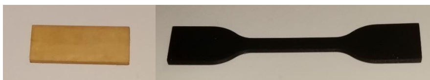
Figure 62. Rectangular specimen in A/TH 60:40 g5 an tensile test specimen in A/TH 60:40 w5
