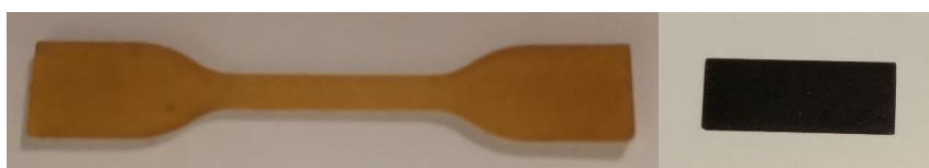
Figure 61. Tensile test specimen in A/IB 60:40 g5 and rectangular specimen in A/IB 60:40 w5
