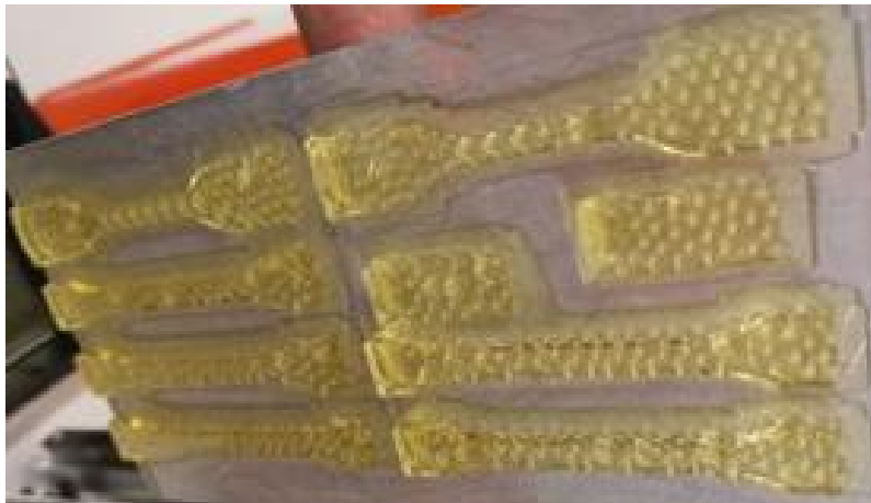
Figure 55. Specimens of A/IB 70:30 with their supports and the bases attached to the printing platform
