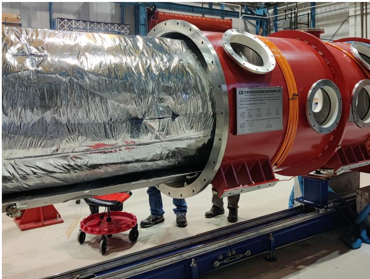
*Figure 5.2: Insertion of the coldmass assembly into the pHB650 vacuum vessel.*
