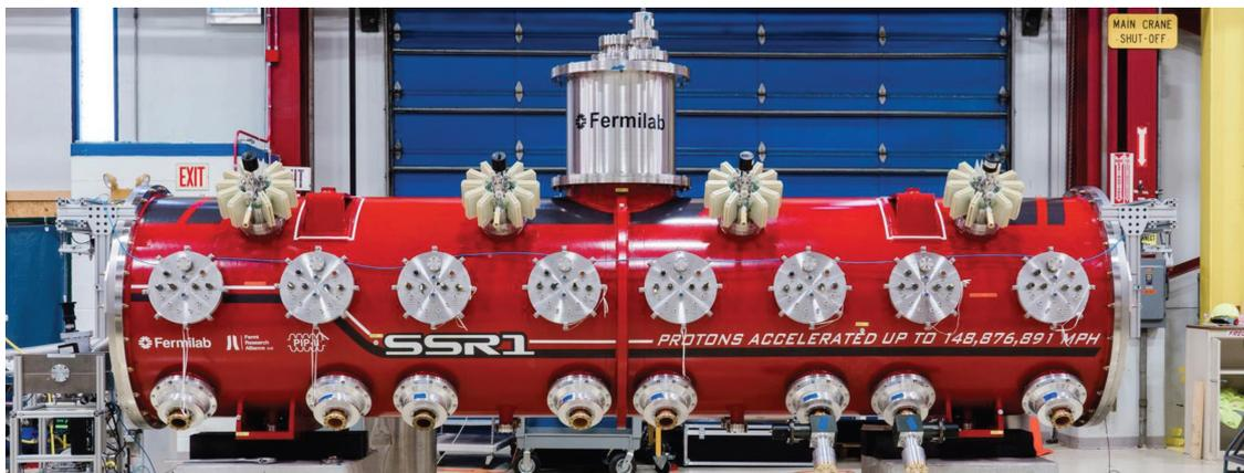
*Figure 1.3: Prototype SSR1 Cryomodule assembled and tested at Fermilab<sup>12</sup>.*
