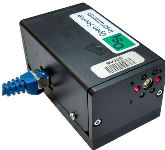
*Figure 2.1: H-BCAM. The front lens is visible, with two laser diodes on either sides. Above and below the lens are the four LED flashes<sup>13</sup>.*
