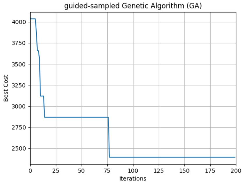
Figure 4.20: OF best solution for each iteration related to Scenario (b) - Symmetric Warren
