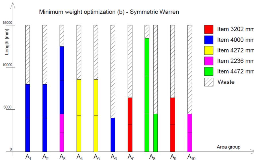
Figure 4.19: Optimal cutting pattern derived by traditional optimization scenario (b) - Symmetric Warren
