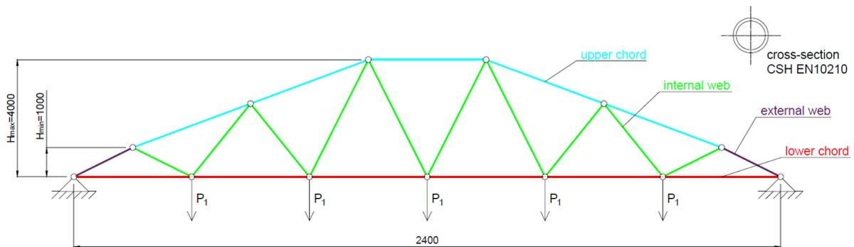
Figure 4.24: Configuration of the Warren truss under analysis, the members are divided into 4 cross-sectional areas which are the 4 design variables, measures are expressed in millimetres (mm)
