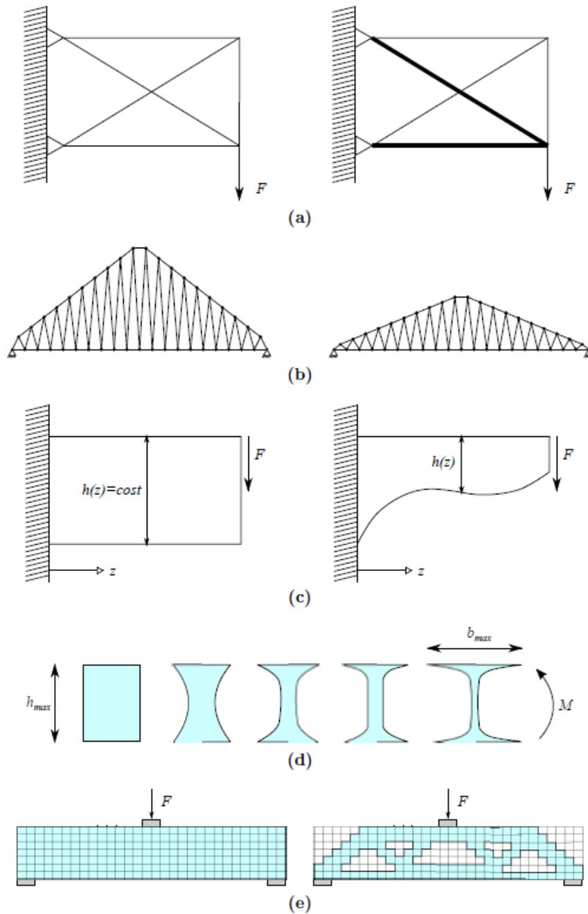
Figure 2.1: On the left column, starting design situations are presented; on the right column, optimized designs are depicted. (a) Size optimization; (b) Shape optimization of a Warren truss beam; (c) Shape optimization with a parametric function  $h(z)$ ; (d) Continuum Topology optimization of a rectangular cross section under a bending moment in the elastic stage; (e) Topology optimization on a discrete grid (image from [69]).
