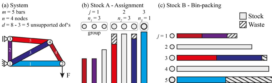
Figure 3.1: (a) Cantilever truss, (b) stock A and assignment, (c) stock B and cutting stock configuration (image taken from [13])
