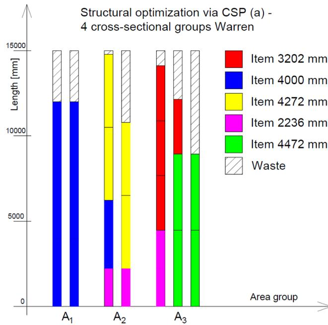
Figure 4.25: Optimal cutting pattern derived by optimization via CSP scenario (a) - 4 DV Warren
