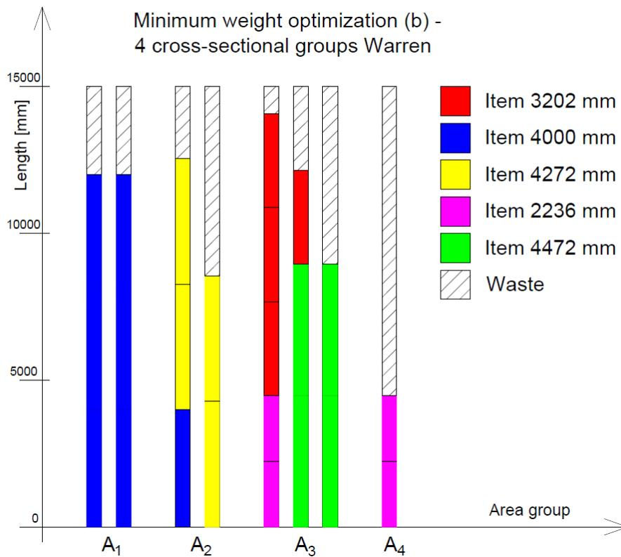
Figure 4.30: Optimal cutting pattern derived by traditional optimization scenario (b) - 4 DV Warren
