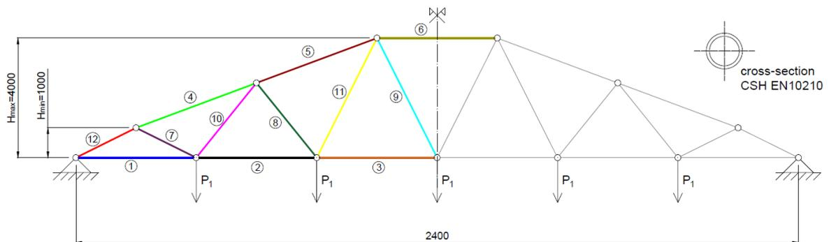
Figure 4.13: Configuration of the Warren truss under analysis, the numbers indicate the design variables which are 12 because the symmetry is considered, measures are expressed in millimetres (mm)
