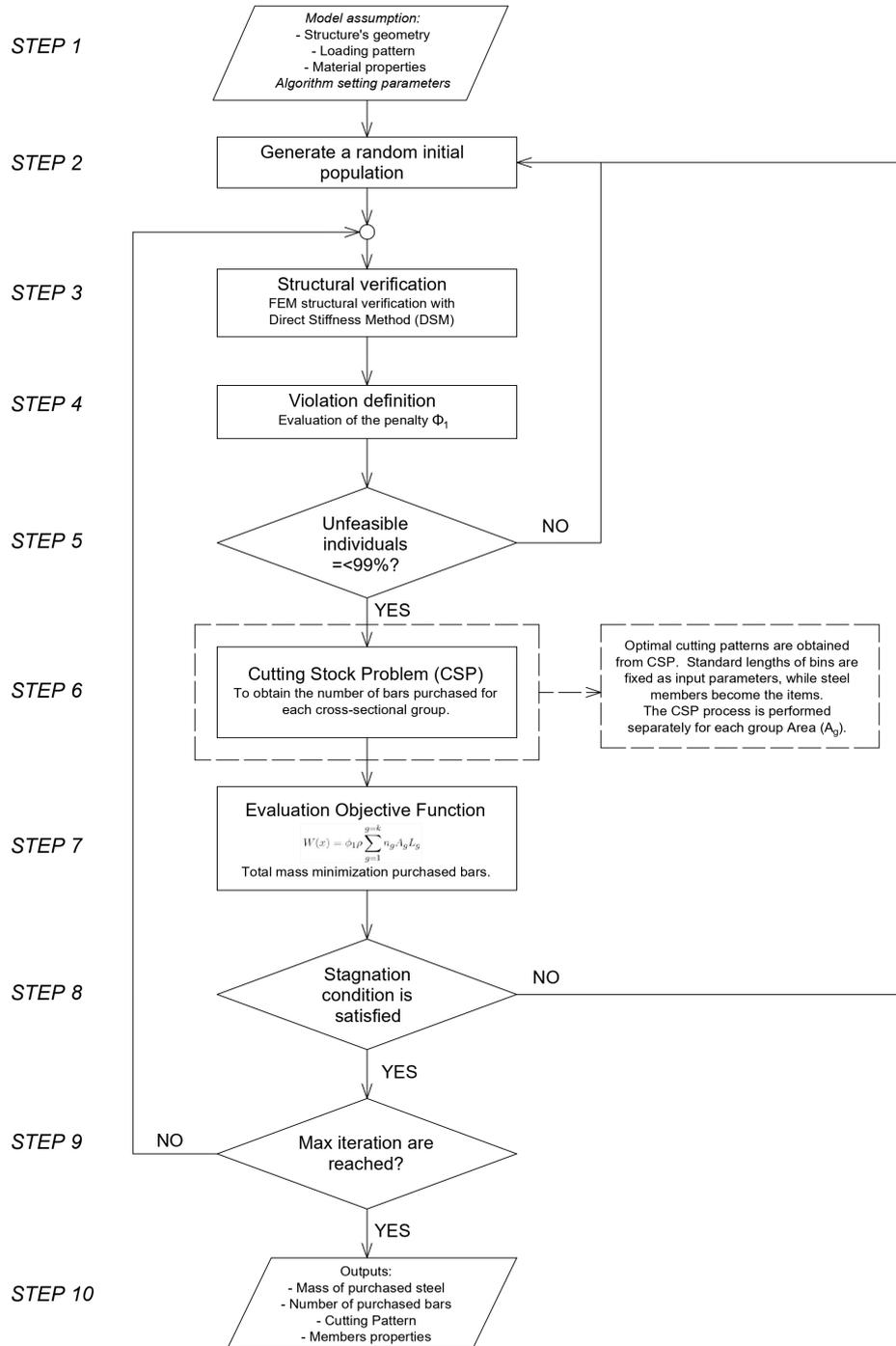
Figure 4.2: Structural Optimization via CSP problem algorithm
