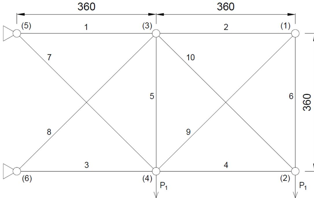
Figure 4.4: Configuration of the in-plane 10-bar truss, measures are expressed in inches (in.)
