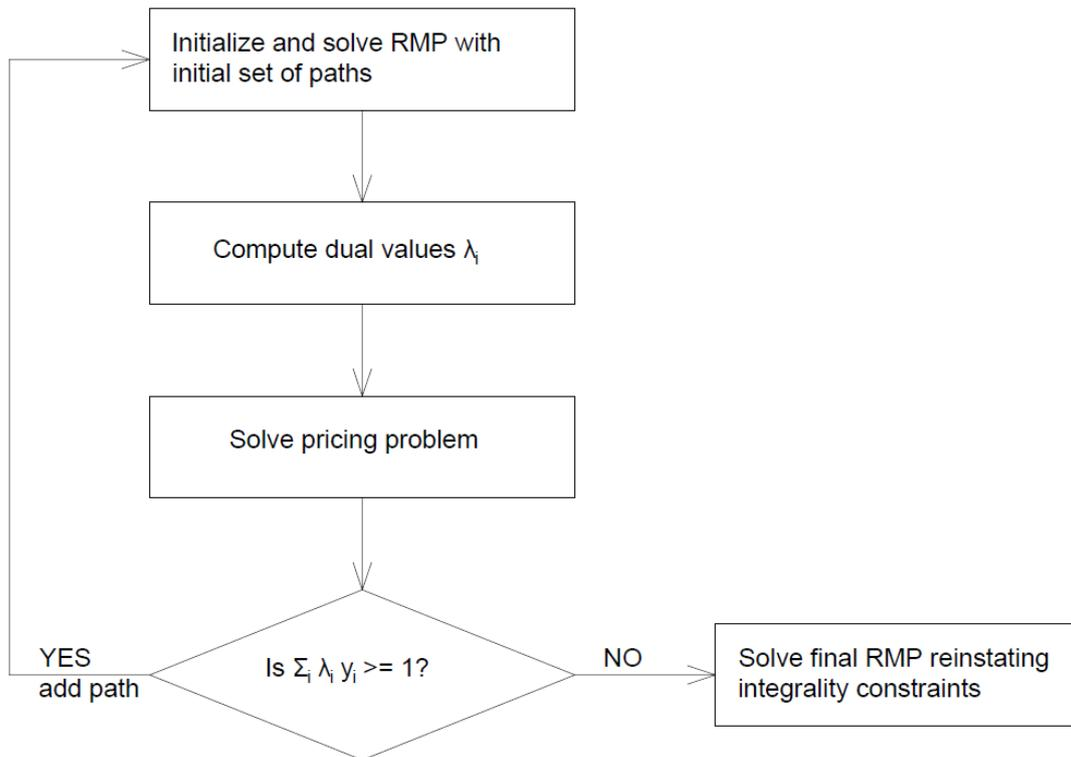
Figure 3.2: Column Generation algorithm for the solution of Cutting Stock Problem
