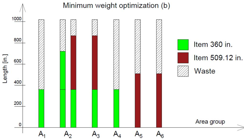
Figure 4.9: Optimal cutting pattern derived by optimization scenario (b)
