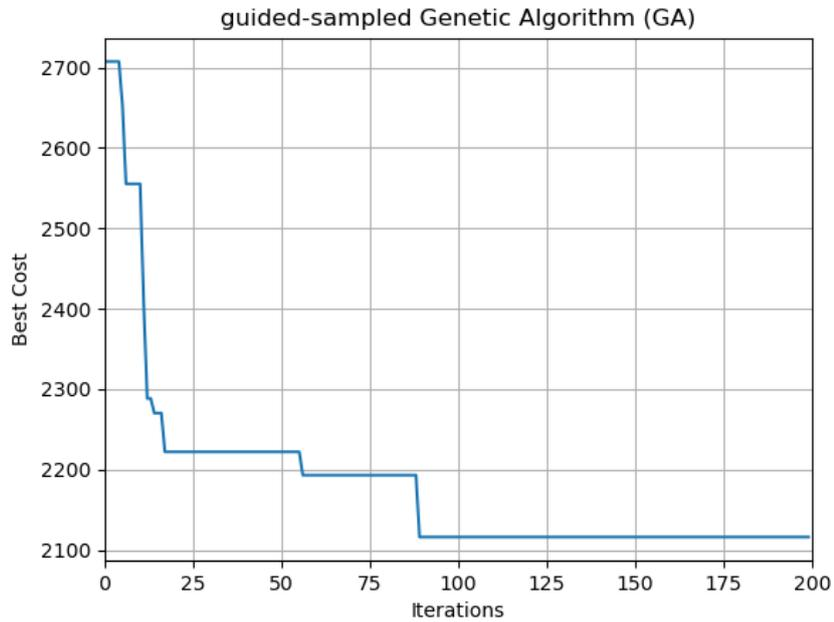
Figure 4.31: OF best solution for each iteration related to Scenario (b) - 4 DV Warren
