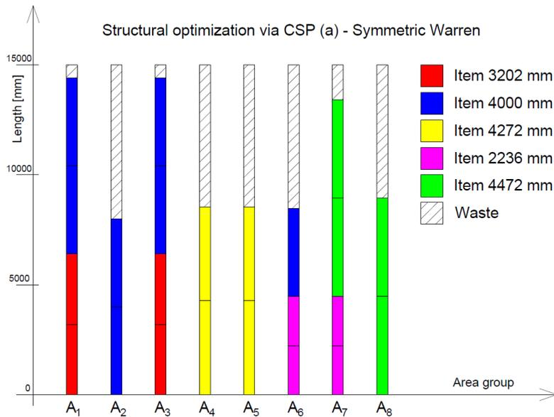
Figure 4.14: Optimal cutting pattern derived by optimization via CSP scenario (a) - Symmetric Warren
