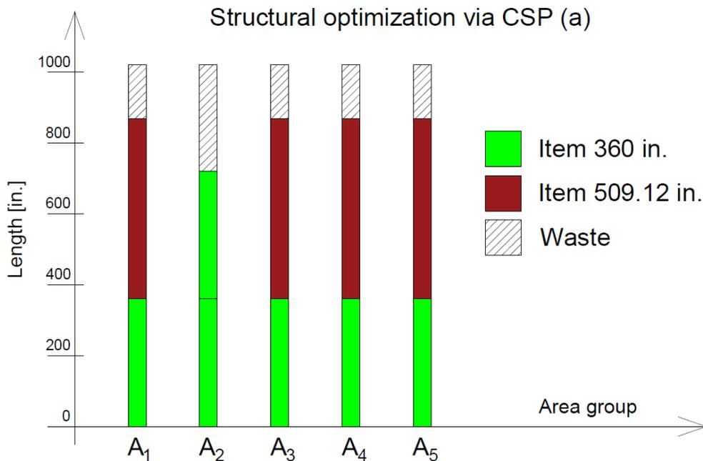
Figure 4.5: Optimal cutting pattern derived by optimization scenario (a)
