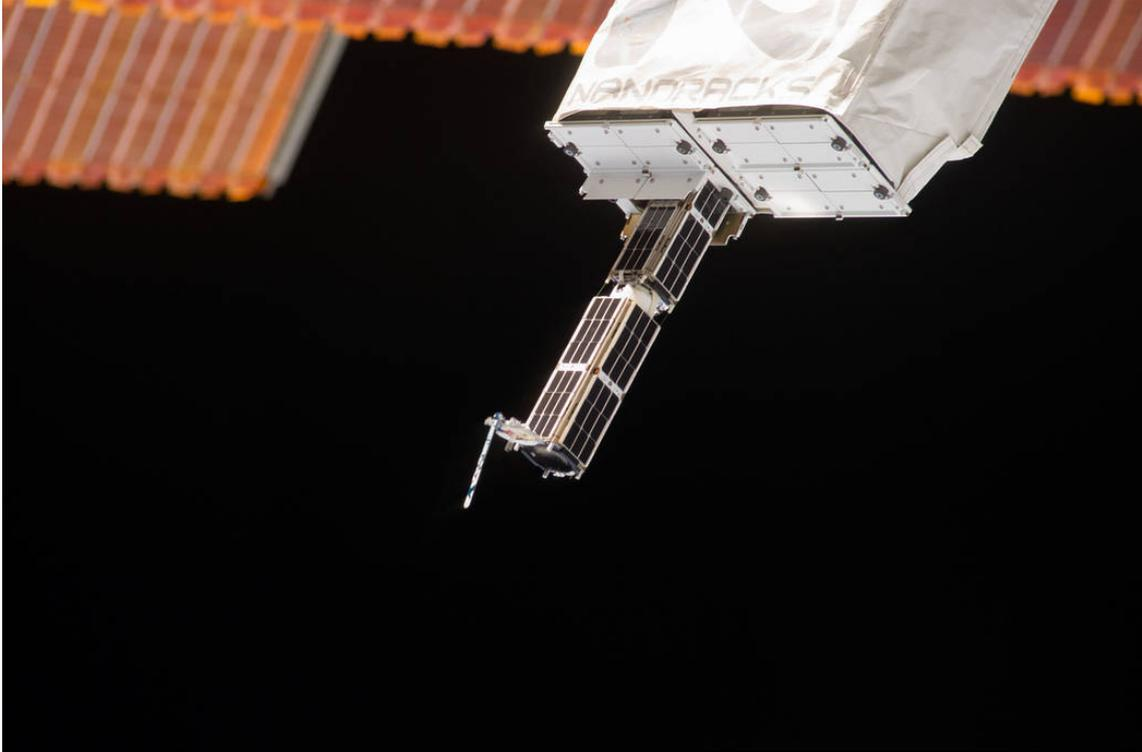
**Figure 1.1:** Nanoracks Cubesat Deployer (credit NASA [6])
