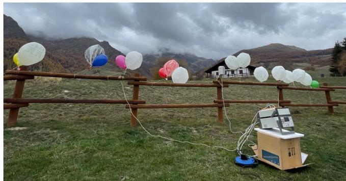
Figure 6.4: Calibration phase: temperature measurement by INRiM instrumentation and mounted probes.
