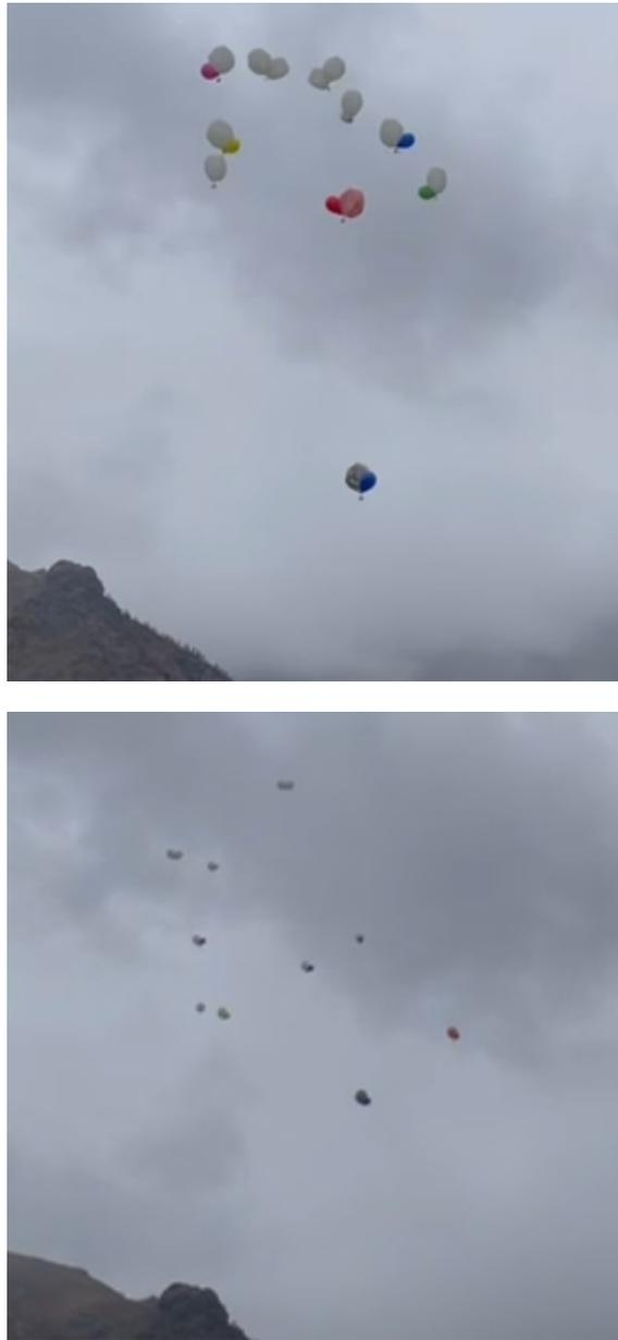
Figure 6.14: Images taken about 10 and 40 seconds after launch, respectively. It can be seen that the probes proceed in a cluster and follow the air swirls.
