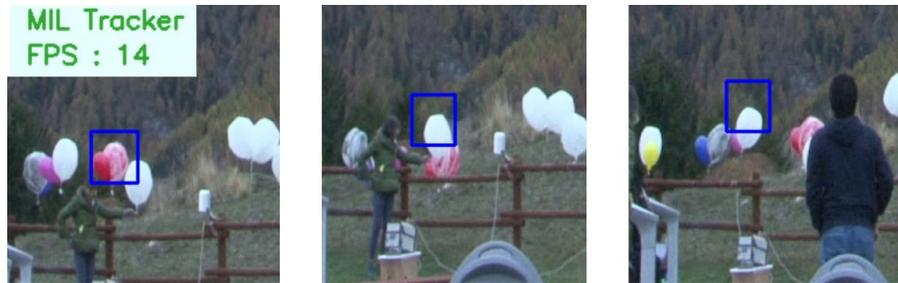
Figure 6.38: Tracker test. In the three consecutive frames it is shown how the algorithm loses tracking of the red balloon as soon as another one approaches it.
