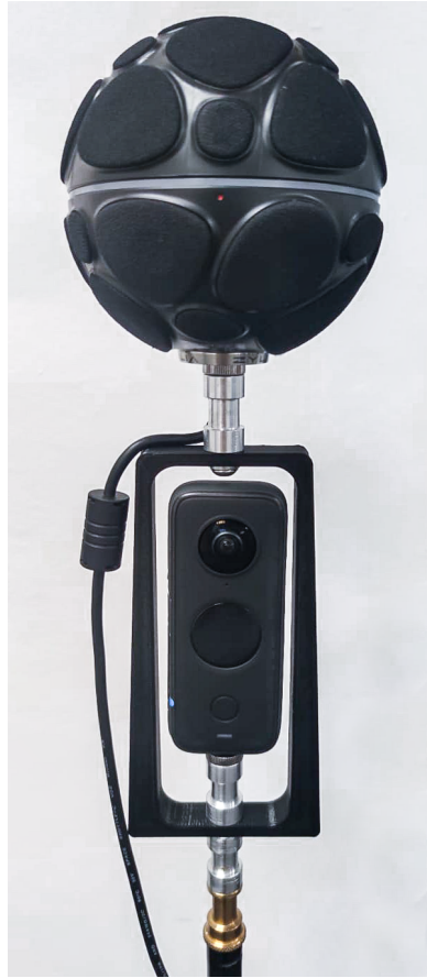
Figure 5.1: The stand that will be used to make synchronized audiovisual recordings in the environments that will be measured in the future.
