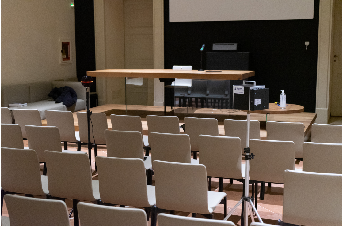
Figure 3.9: Measuring a RIR associated with a noise source in the conference hall.
