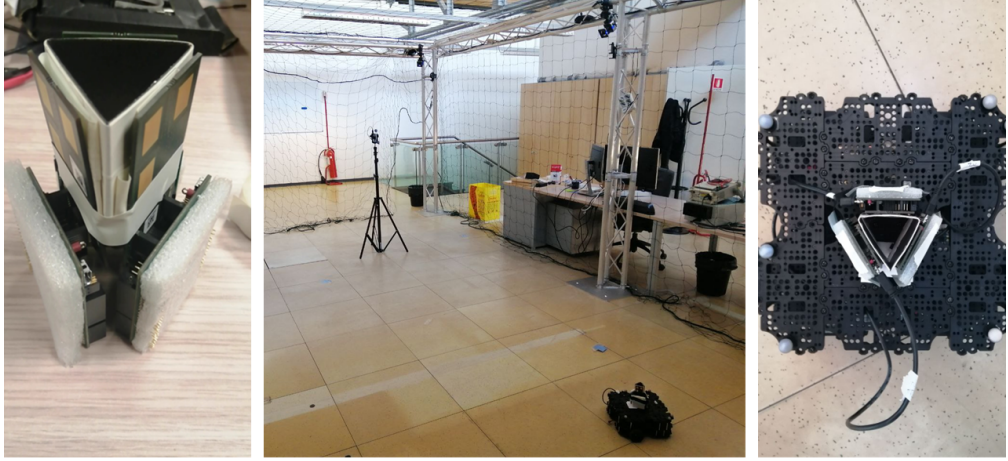
Figure 4.8: On the left the three anchors shifted of 120^\circ , in the center is possible to see the VICON cameras in the corners of the cage and on the right the TurtleBot with the anchors and the marker placed on.
