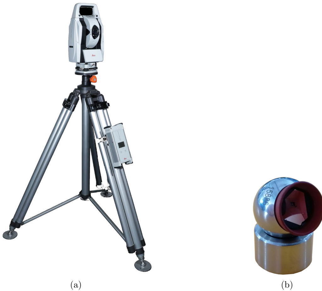
Figure 5.1.3: Leica AT430 mounted on a tripod with its control unit (a) and the 0.5" prism used in anchors' placement (b)
