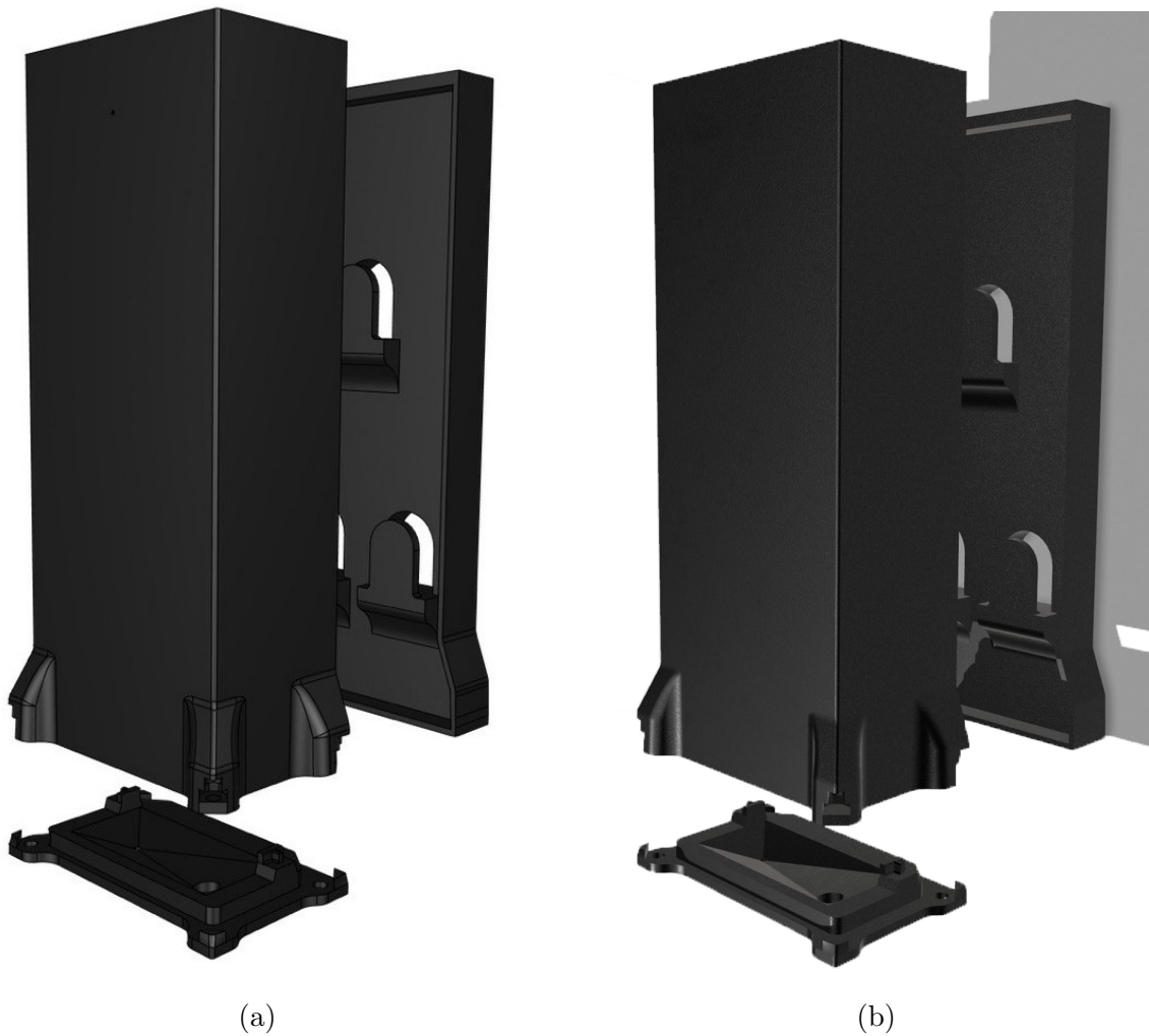
Figure 5.2.7: Case design expanded in its three components (a) and its render (b)
