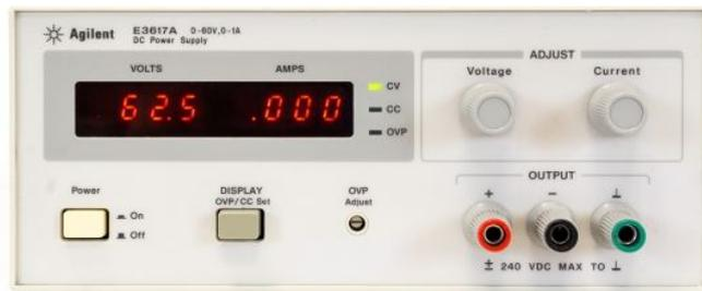
Figure 2.17: Front view of a Power Supply single channel (figure taken from [1])
