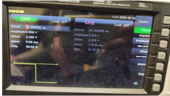
Figure 2.20: Parameters set to generate the square waves
