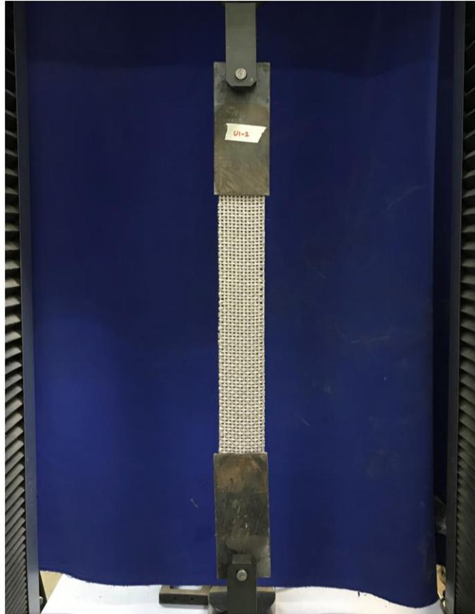
Figure 3.11 - Tensile test sample in Microforce Testing Machine (During Test)
