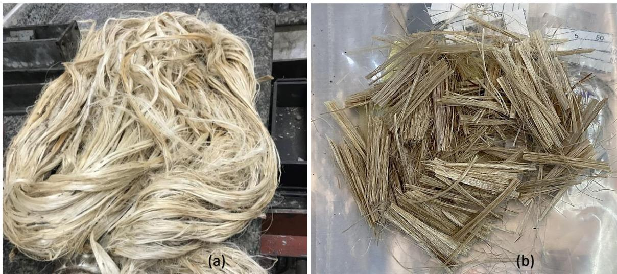
Figure 4.2 - Raw jute fibers as procured (a); treated & sized fibers to be used in mortar (b)
