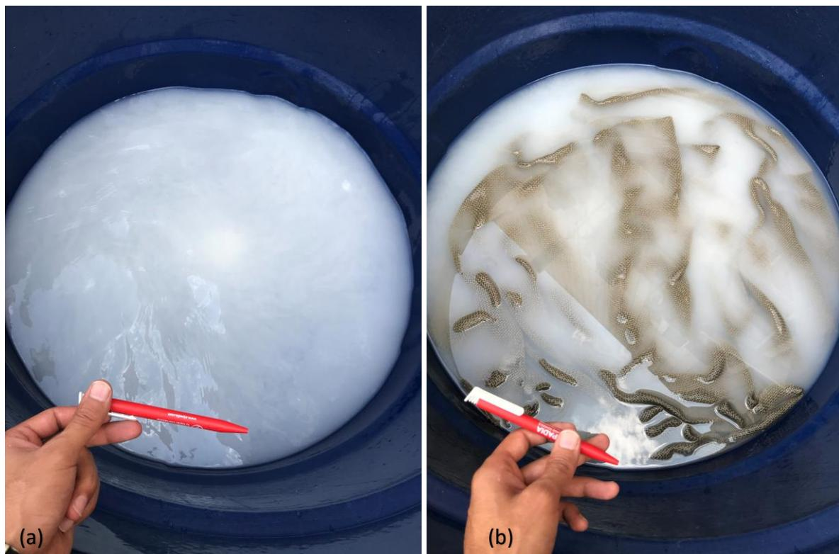
Figure 3.2 - Saturated solution of  $\text{Ca}(\text{OH})_2$  in water (a); flax fabric immersed in solution (b)
