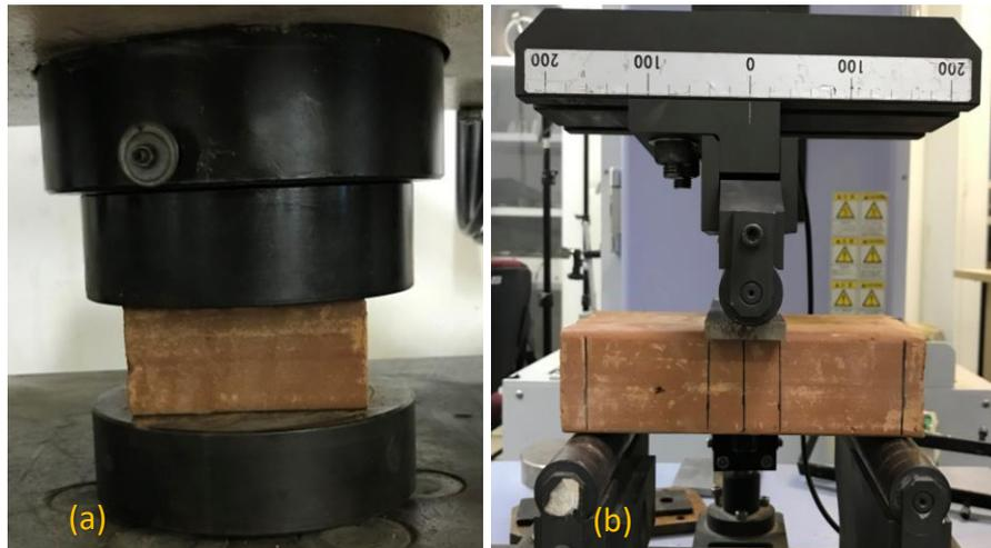
Figure 5.1 - Brick compression test set-up (a); test set-up for modulus of rupture (b)
