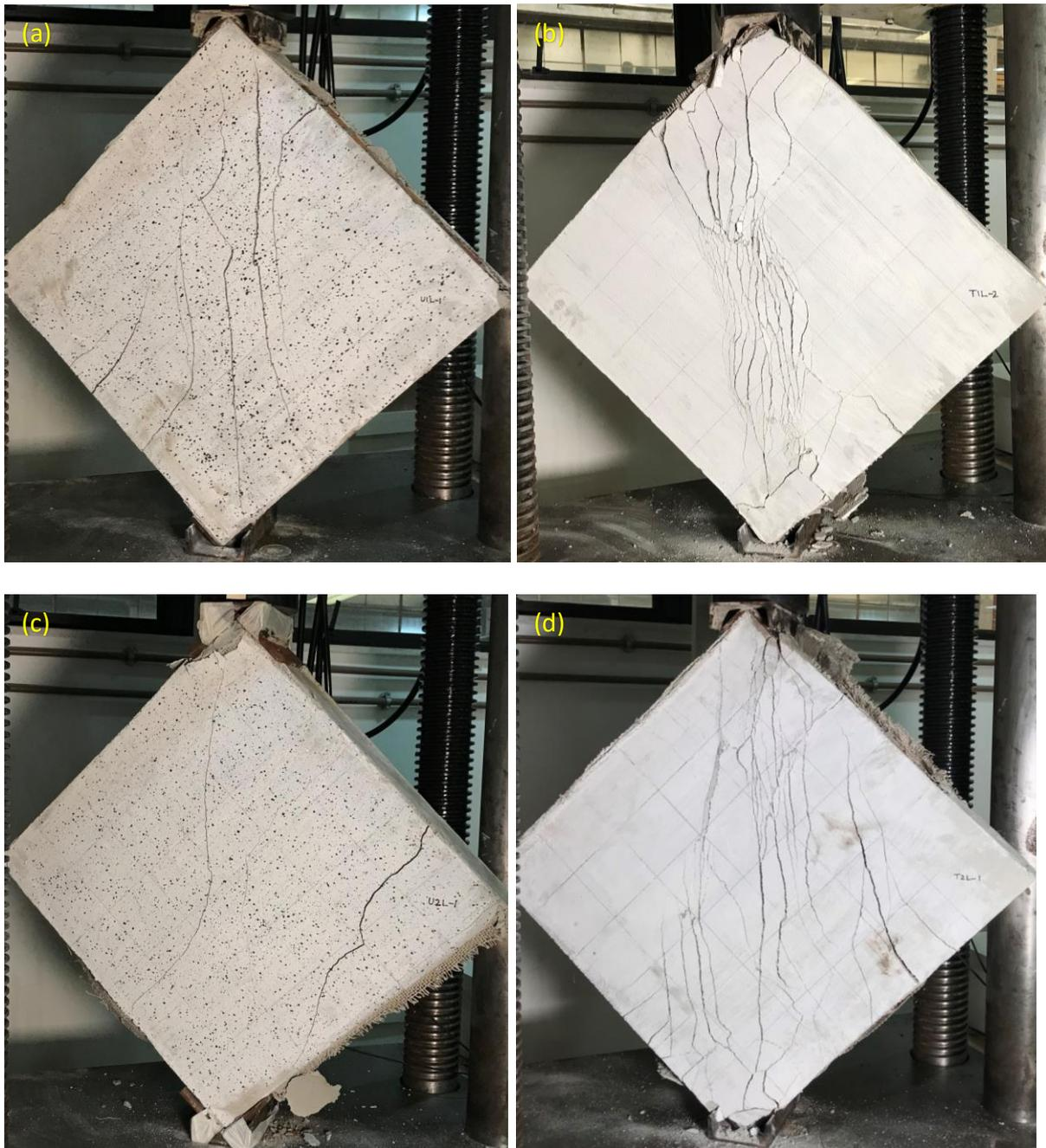
Figure 5.13 - Crack development in representative samples of Wall-U1L (a); Wall-T1L (b); Wall-U2L (c); Wall-T2L (d)
