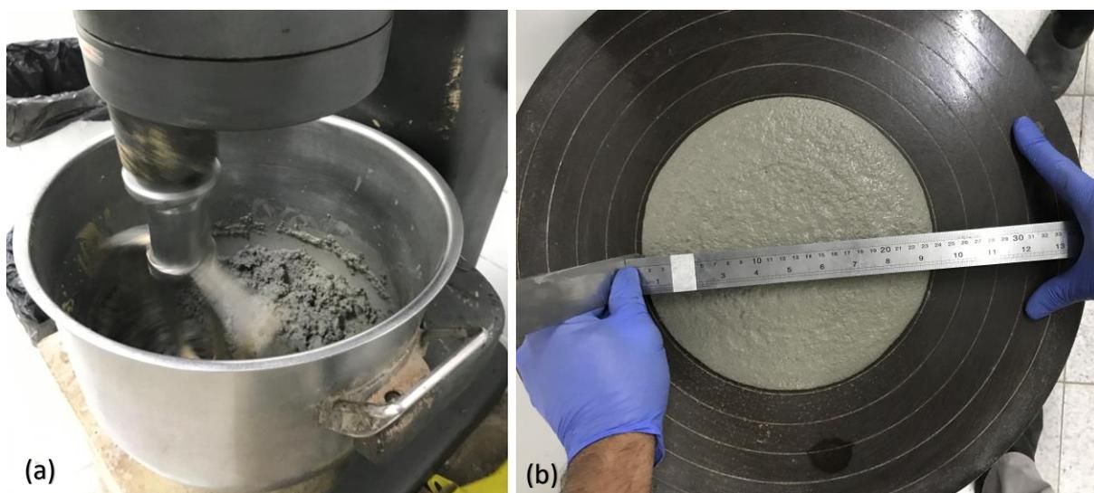
Figure 4.3 - Mortar during mixing (a); fresh state consistency measurement (b)
