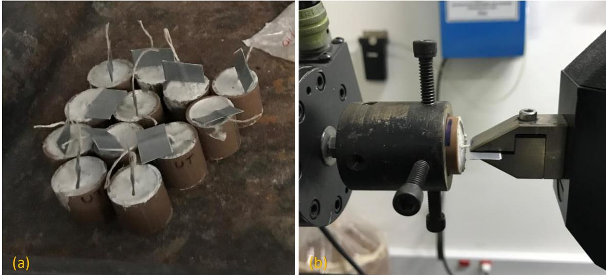
Figure 4.19 - Pull-out samples (a); test set-up (b)
