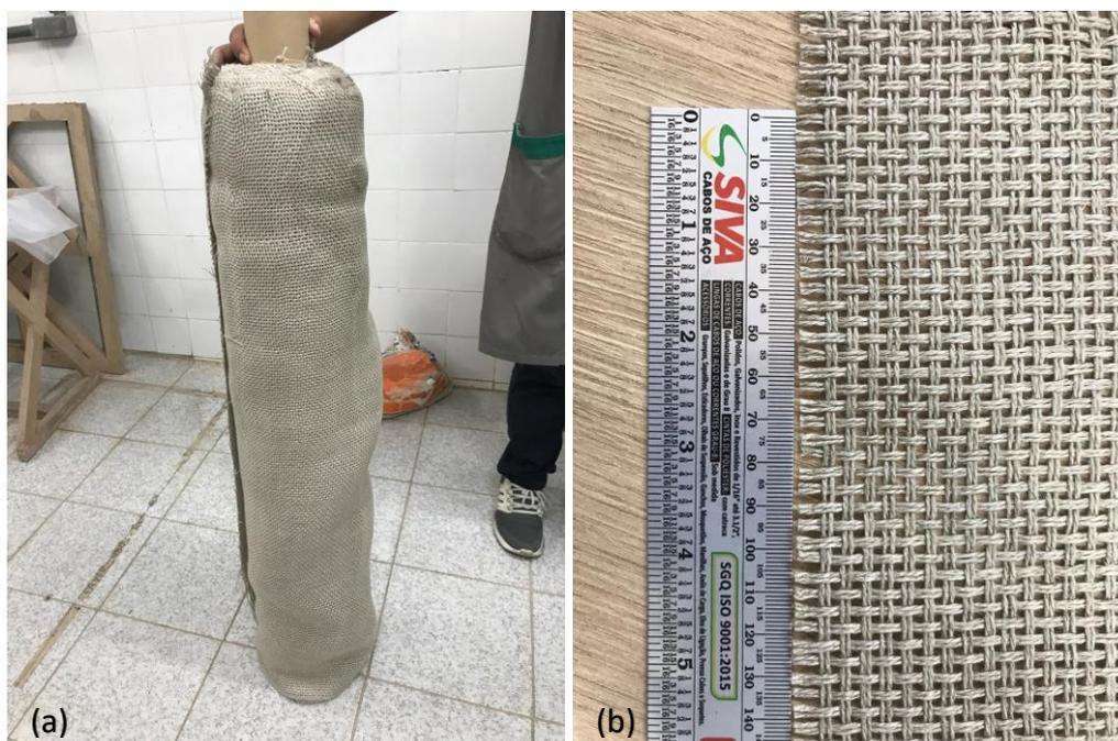
Figure 3.1 - Bidirectional Flax fabric 100 cm wide roll (a); magnified texture of the fabric (b)
