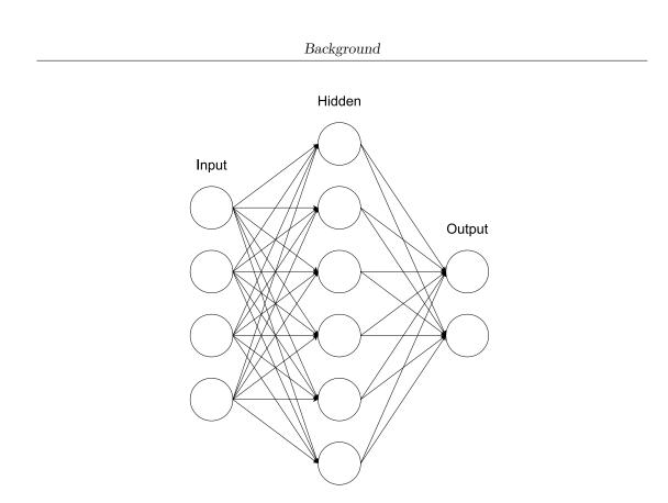
Figure 2.5: A deep neural network with one fully connected hidden layer. In this case, the Heaviside step function could be replaced by the positive part  $f^+$ , also known as the ReLU (Rectified Linear Unit) activation function (see figure 2.6c), commonly used in today's deep networks [61]. It can be implemented in Python as max(0, value).
