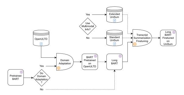
Figure 4.1: A diagram of the training process used to produce the models presented in this work. First we perform BART's [10] domain adaptation on OpenULTD (§ 4.2.1), then we convert BART with long attention to either LED [6] or LSG [7], and finally we finetune the resulting model on either the standard or the extended variant of the UniSum dataset (§ 4.2.2).
