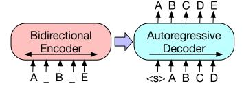
(c) With BART, the input document is subjected to arbitrary noise transformations and fed into a bidirectional encoder (on the left), then the likelihood of the original input sequence is computed with the autoregressive decoder (on the right). To finetune BART, an uncorrupted input is given to both encoder and decoder, then the representations from the final hidden state of the decoder are used.
