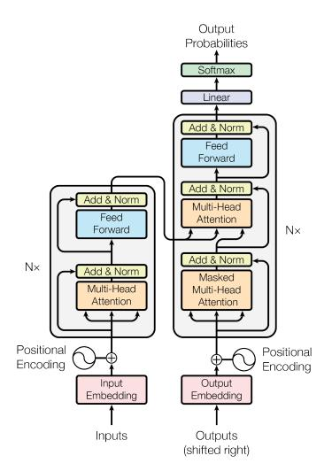
Figure 2.9: The Transformer architecture as presented in the original paper [1], where this is figure 1.
