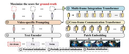
**Figure 3.7:** The X-CLIP framework, which allows for freely chosen natural language text labels and jointly processes them with a video clip using a cross-frame communication Transformer in combination with a multi-frame integration Transformer. Figure 2 in [4].
