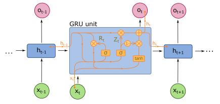
(b) A diagram for a one-unit Gated Recurrent Unit (GRU).
