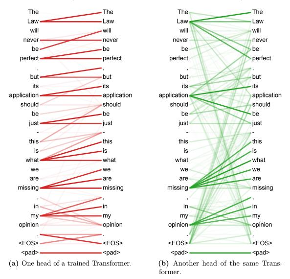
**Figure 2.10:** Figure 5 in the original Transformer paper [1]: «many of the attention heads exhibit behaviour that seems related to the structure of the sentence. We give two such examples above, from two different heads from the encoder self-attention at layer 5 of 6. The heads clearly learned to perform different tasks.»
