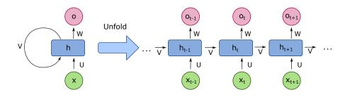
Figure 2.7: A diagram for a one-unit recurrent neural network (RNN). From bottom to top: input state x, hidden state h, output state o. U, V, and W are the weights of the network. Looping diagram on the left and unfolded version on the right. The t subscript indicates the time instant. By Wikipedia user fdeloche, shared under the CC BY-SA 4.0 license.
