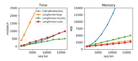
**Figure 3.4:** Runtime and memory usage dependence from the input sequence length in tokens. Comparison of full Self-Attention with respect to different implementations of the Longformer attention. Figure 1 in [6].
