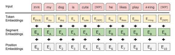
Figure 2.13: BERT's input representation. It is shown that, on top of the now familiar token and position embeddings (see § 2.2), BERT makes use of additional segment embeddings to encode information useful for its NSP pretraining task. Figure 2 in [2].
