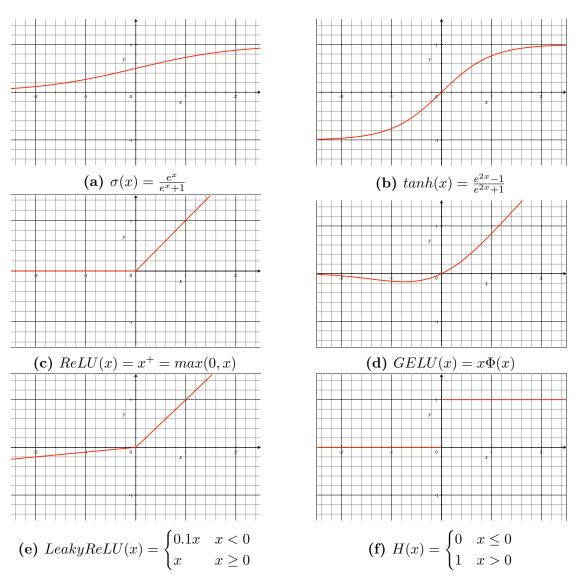
**Figure 2.6:** Five commonly used activation functions in today's deep networks and the Heaviside step function used in the Perceptron (2.6f). The most notable are the rectified linear unit (2.6c) and its derivatives: the GELU [62] (2.6d) and the leaky ReLU (2.6e, shown with an arbitrary 0.1 slope factor in the negative part). The sigmoid (2.6a) and the hyperbolic tangent (2.6b) were more widely used in the past.
