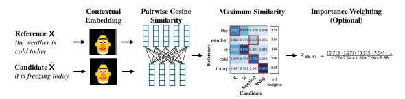
**Figure 5.1:** A diagram of the computation of the recall measure in BERTScore. Figure 1 in [9].
