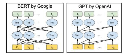
**Figure 2.11:** A diagram highlighting the bidirectional Transformer architecture of BERT [2] versus the left-to-right GPT [13]. BERT's representations are conditioned on left and right context in every layer. From figure 3 in [2].
