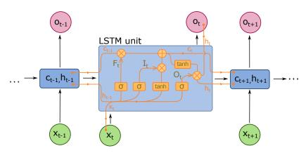
(a) A diagram for a one-unit Long Short-Term Memory (LSTM).
