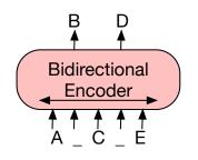
(a) With BERT, tokens are randomly replaced with masks and the input sequence is encoded bidirectionally. The masked tokens are predicted independently of each other, which does not allow for text generation.
