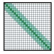
(b) Sliding window attention. If the sliding window's width is w, every *i*th token attends to the tokens in the sliding window:  $\{t_{i-\frac{w}{2}}, ..., t_{i}, ..., t_{i+\frac{w}{2}}\}.$
