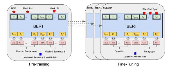
Figure 2.12: «Overall pre-training and fine-tuning procedures for BERT. Apart from output layers, the same architectures are used in both pre-training and fine-tuning. The same pre-trained model parameters are used to initialize models for different down-stream tasks. During fine-tuning, all parameters are fine-tuned. [CLS] is a special symbol added in front of every input example, and [SEP] is a special separator token (*e.g.* separating questions/answers).» Figure 1 in [2].
