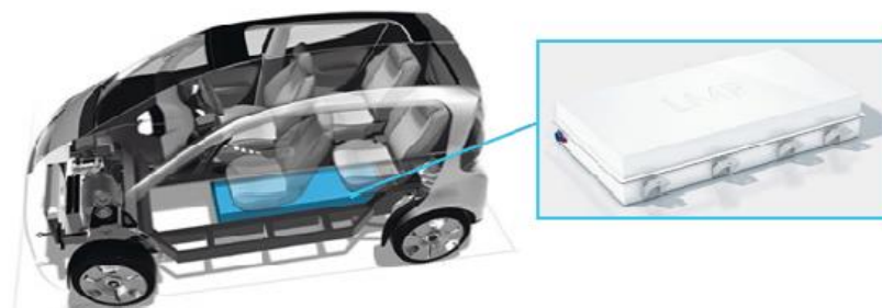
Fig. 8. Floor integration configuration in the Bolloré Bluecar (Wisch, Marcus, Crash compatibility and battery safety, EVERSAFE, 2014)
