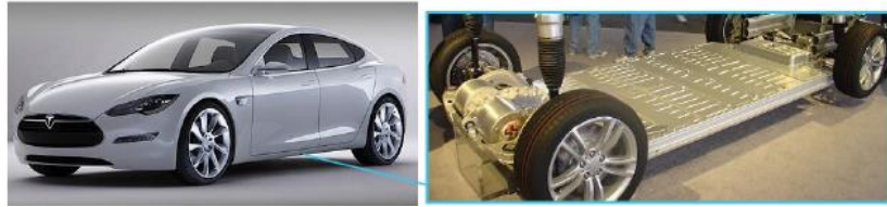
Fig. 11. Platform configuration in the Tesla model S (Wisch, Marcus, Crash compatibility and battery safety, EVERSAFE, 2014)
