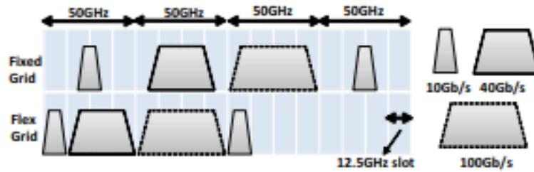
Figure 2.2.4.1 Fixed Grid and Flex Grid [11].
