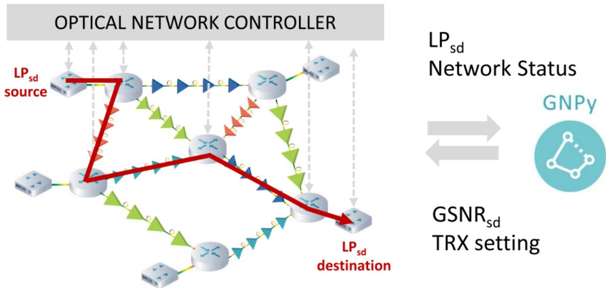
Figure 4.1.1 Architecture for the optical path computation using GNPY [24]
