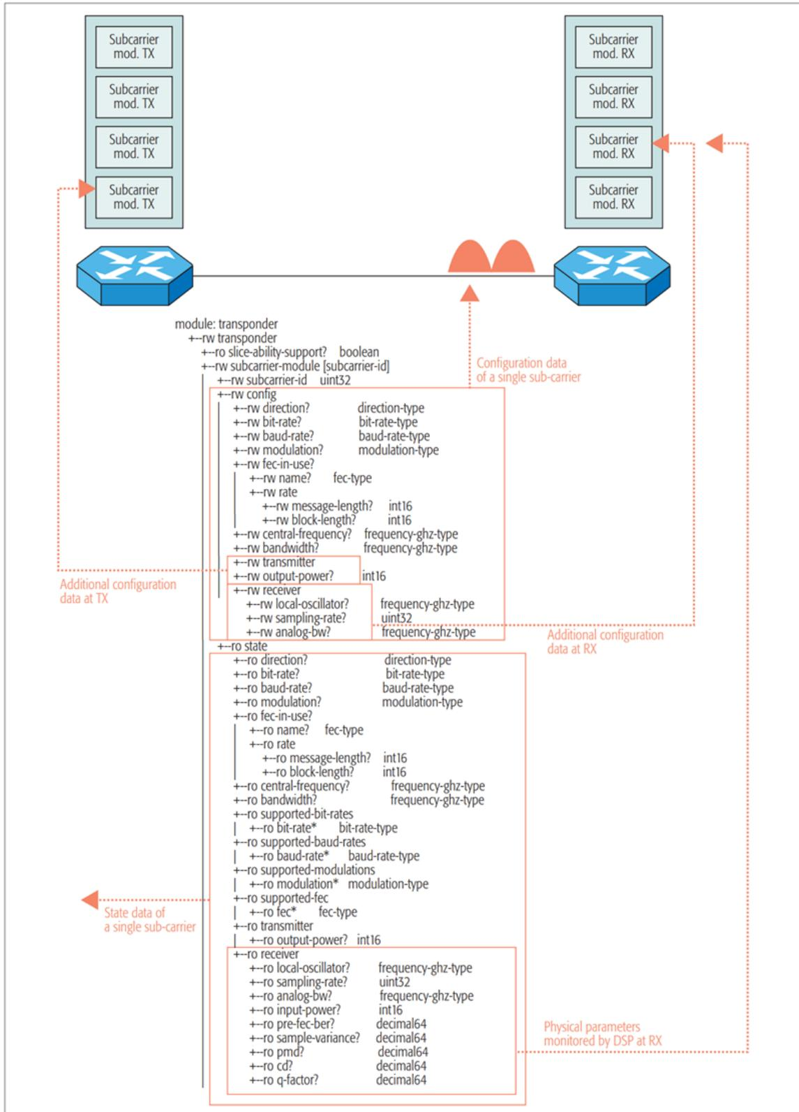
Fig. 6.1.2 YANG tree model representation of a sliceable transponder [8]
