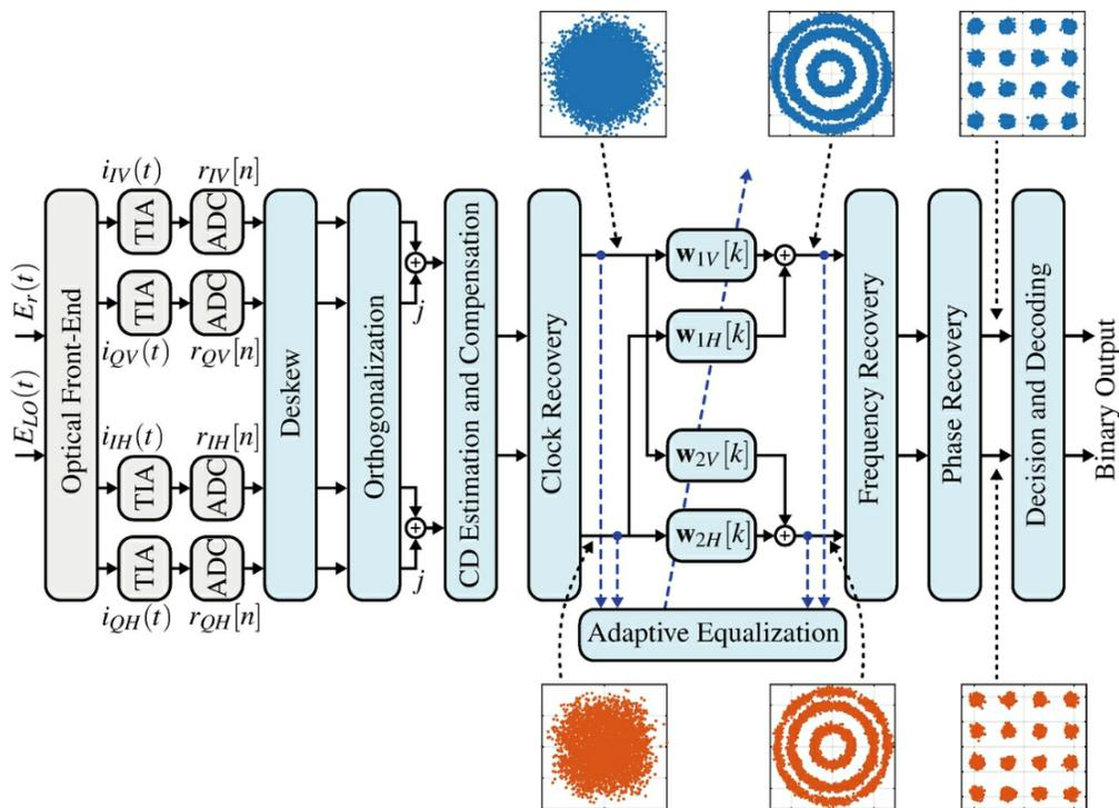
Figure 2.2.7.2 Digital Coherent Receiver [5].
