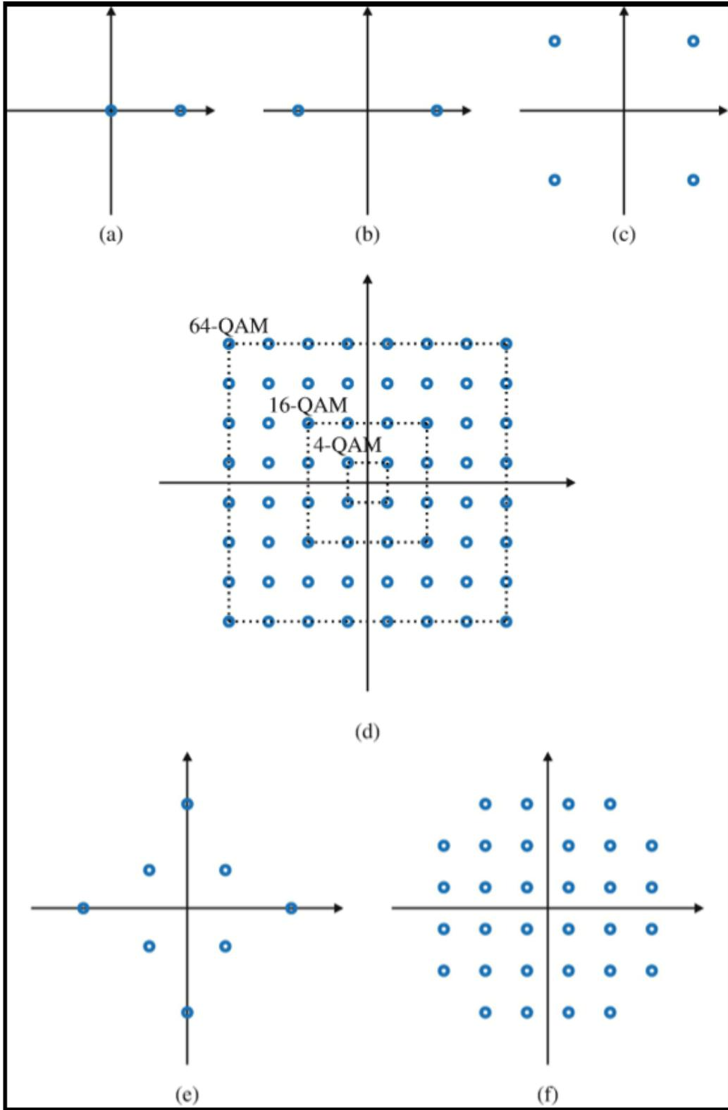
Figure 2.2.6.2 Common constellation used in digital communications [5]
