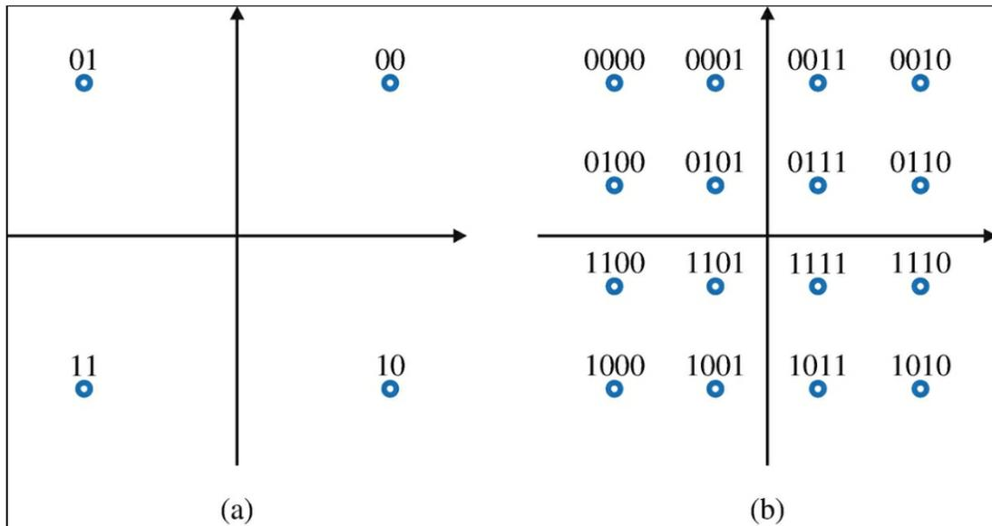
Figure 2.2.6.3 Gray mapping for (a) QPSK (b) 16-QAM [5].
