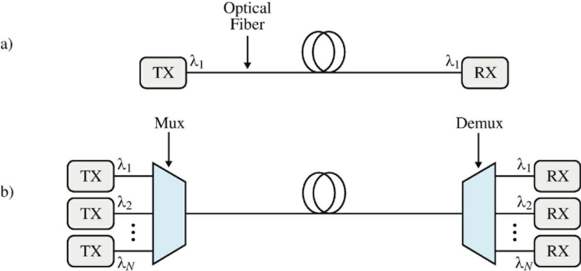
Figure 2.2 (a) Single-wavelength unamplified optical transmission [5]
