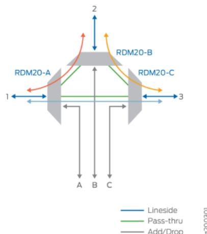
Figure 2.2.1.3 Allowable channel connectivity using pass-through [15].
