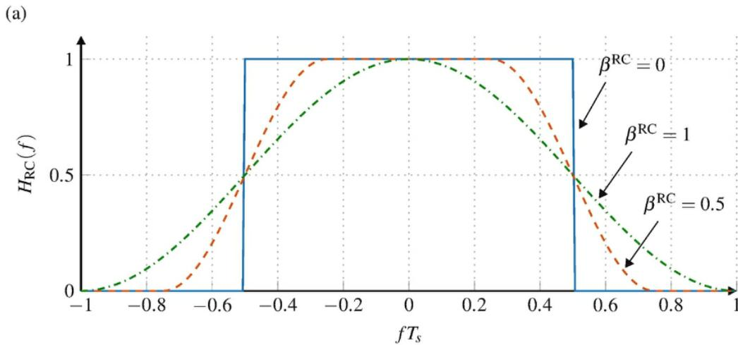
Fig. 2.2.6.4 (a) Raised cosine (RC) filter for different  $\beta^{RC}$  and  $T_s$  - Frequency response [5].
