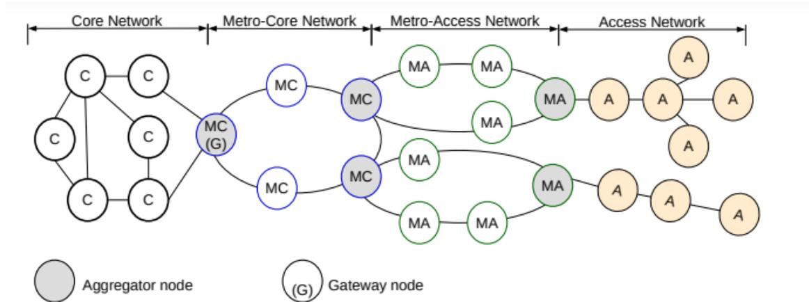
Figure 2.1.1: Structure of an optical transport network [10].
