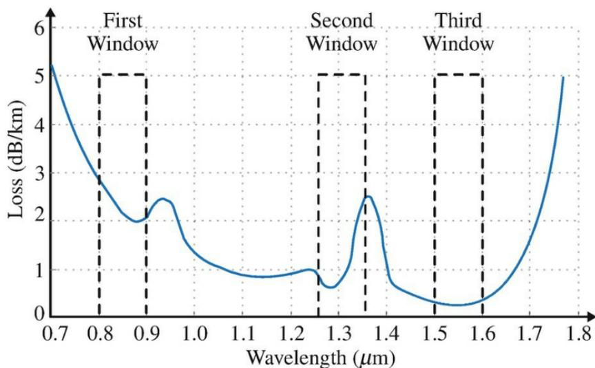
Figure 2.2.5.3.1 Attenuation Profile Of An Fiber [5].
