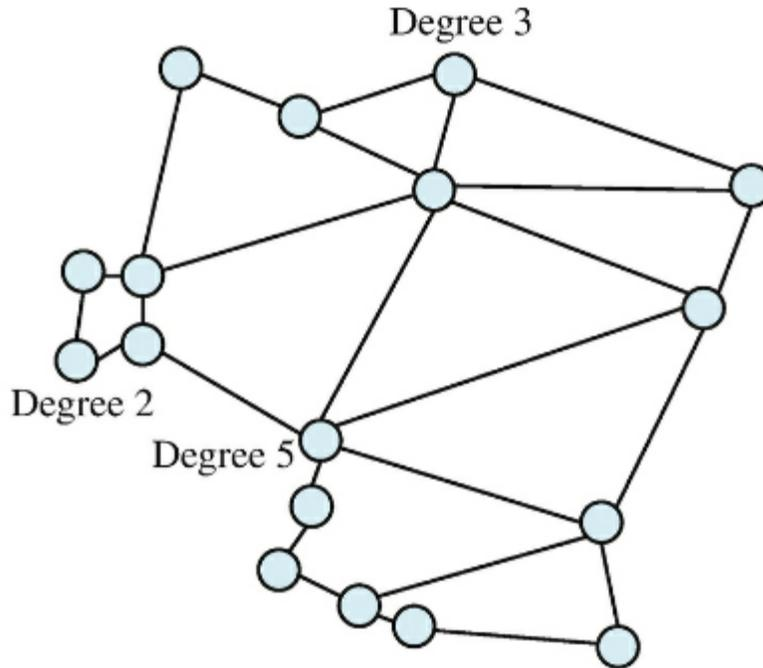
Figure 2.2.1.4 Mesh Optical Network[5]
