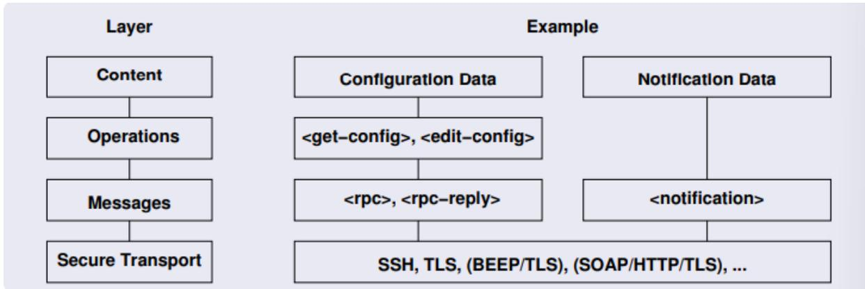
Figure 5.1 NETCONF Layer Model [ RFC 6241 ]
