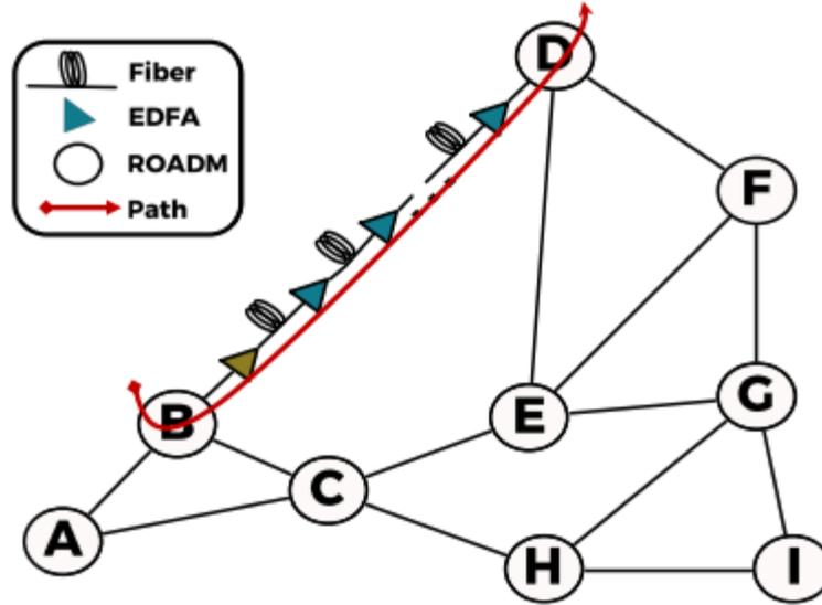
Figure 4.1.2 Path propagation on GNPY to assess the QoT [26]
