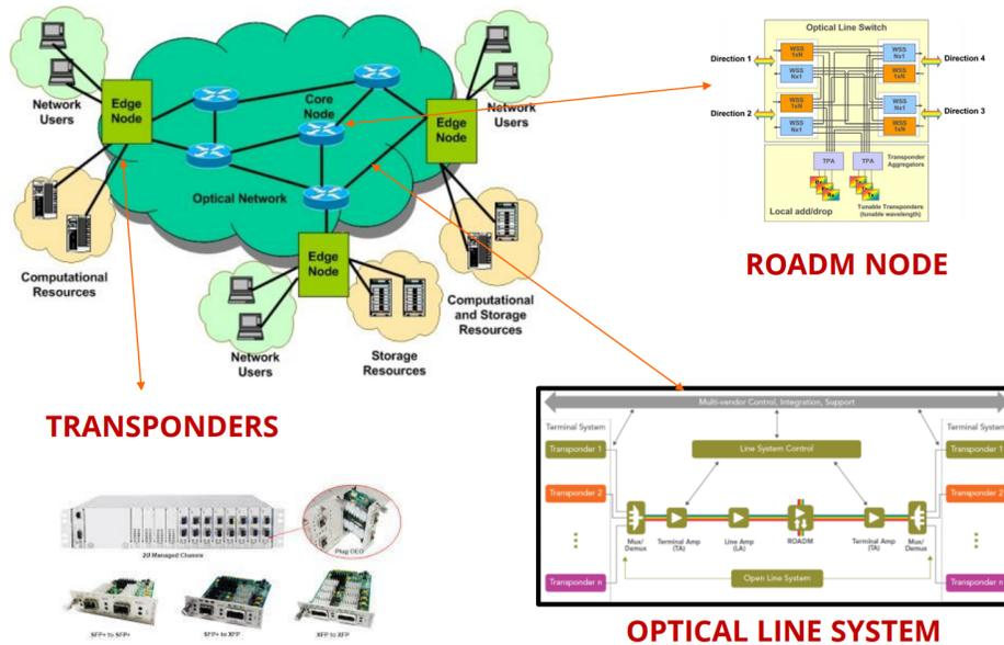
Figure 2.1.4 Sketch of an optical network and its main components
