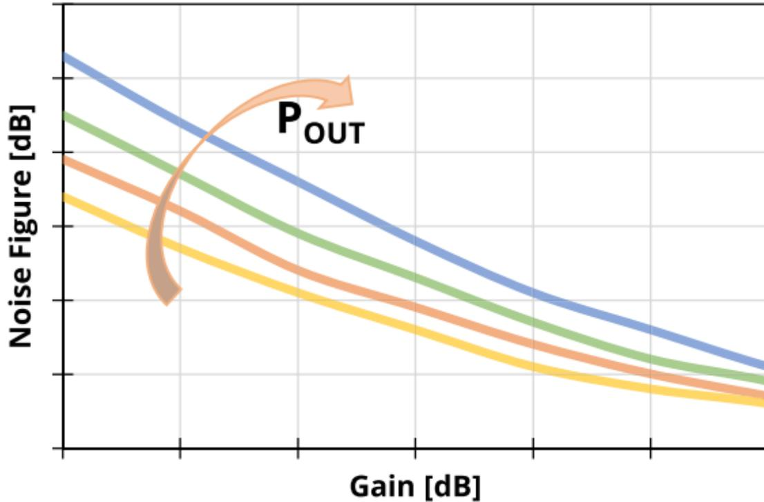
Figure 4.1.3 Qualitative example of the noise-figure-versus-gain and  $P_{out}$  curve of amplifier [26]
