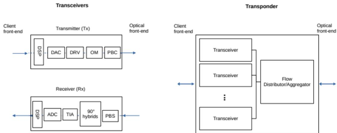
Figure 2.2.2.1 Transceiver and Transponder [10].
