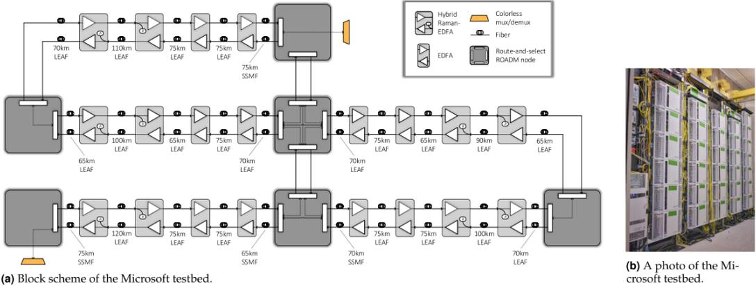
Figure 4.1.5 (a) Block schema and (b) photo of Microsoft testbed [26]
