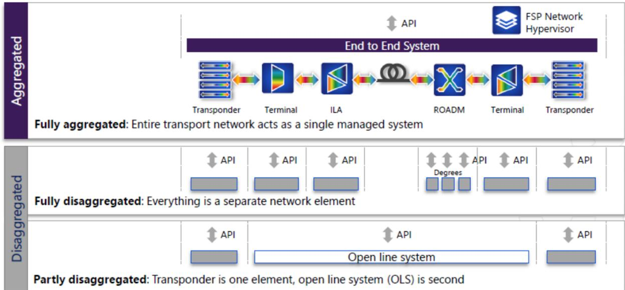
Figure 3.3.2 Optical Network Classification[34]
