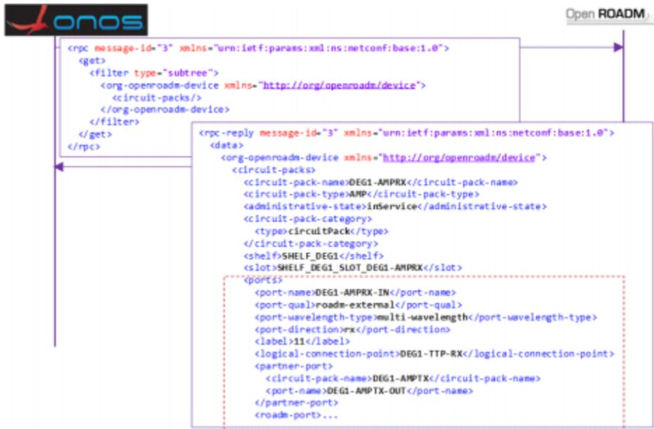
Figure 5.3.1 NETCONF <get> operation to retrieve list of circuits of ROADMs [27]
