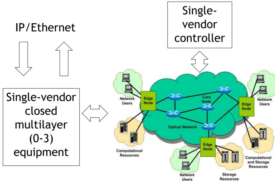
Figure 3.3.1 Closed Optical Network
