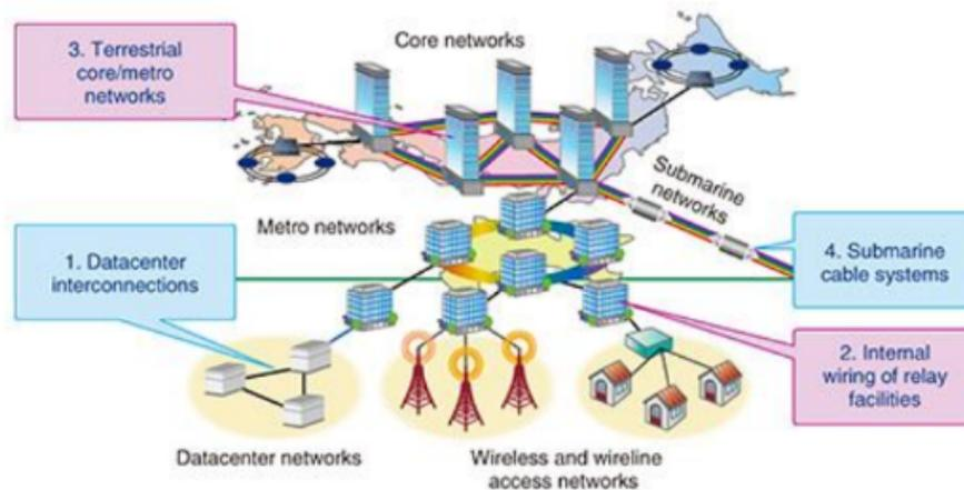
Figure 1.1: Logical subdivision of an optical network [10].
