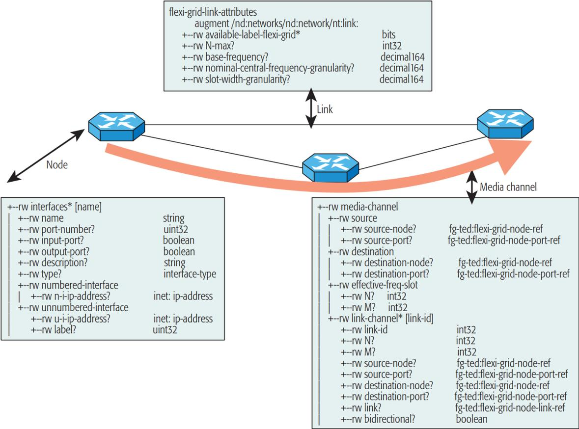
Figure 6.1.1 YANG model of node, link and media channel [8]
