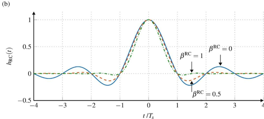
Figure 2.2.6.4 (b) Raised cosine (RC) filter for different  $\beta^{RC}$  and  $T_s$  - Impulse response [5].
