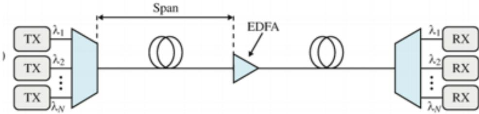
Figure 2.2.4.2 WDM optical system with EDFA [5].
