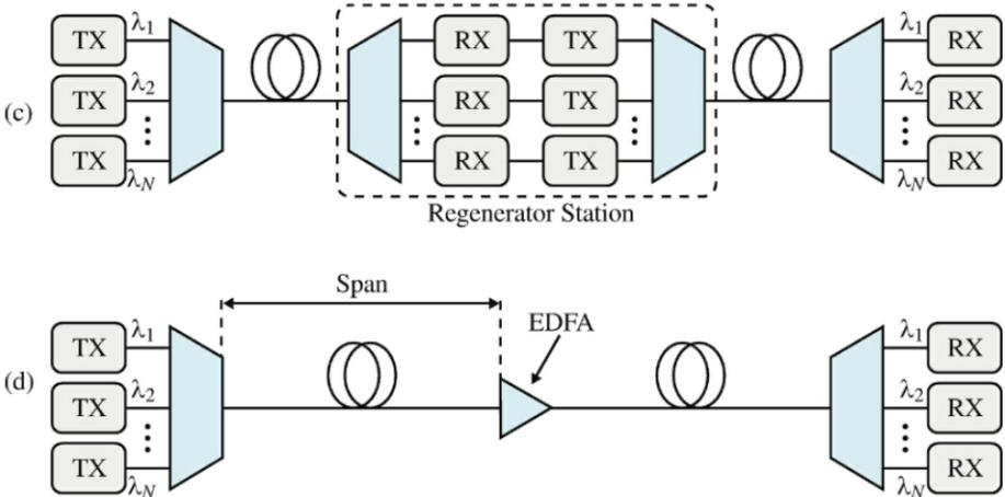
Figure 2.2 (c) WDM unamplified long-reach system [5].
