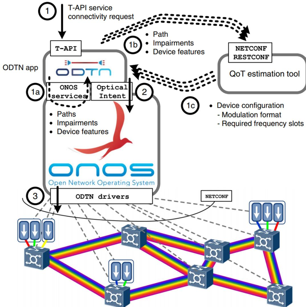
Figure 7.2.2 SDN reference architecture [2]
