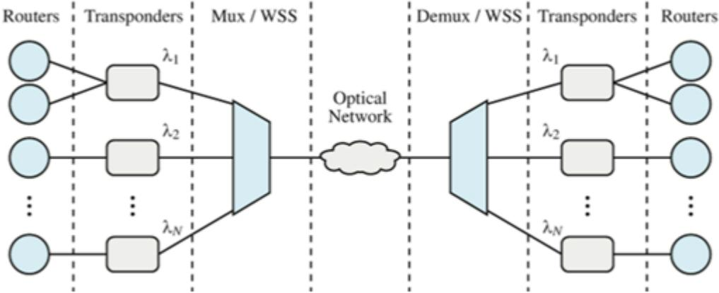
Figure 2.2.4.3 Transponder and WDM signal generation [5].
