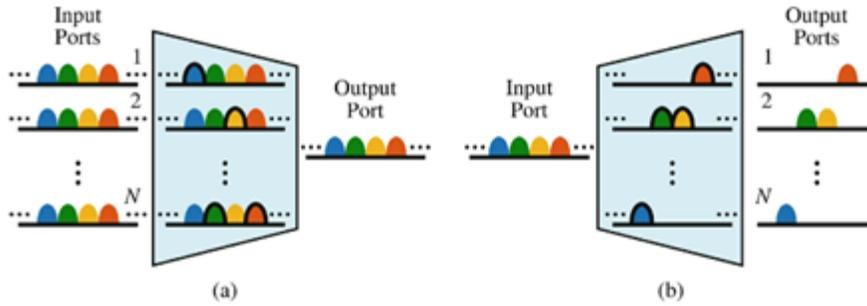
Figure 2.2.1.1 (a) WSS Multiplexer (b) WSS Demultiplexer [5]
