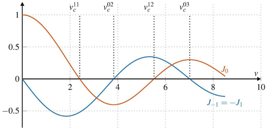
Figure 2.2.5.2 Cut-off frequencies of LP for  $l=0$  and  $l=1$  [5].
