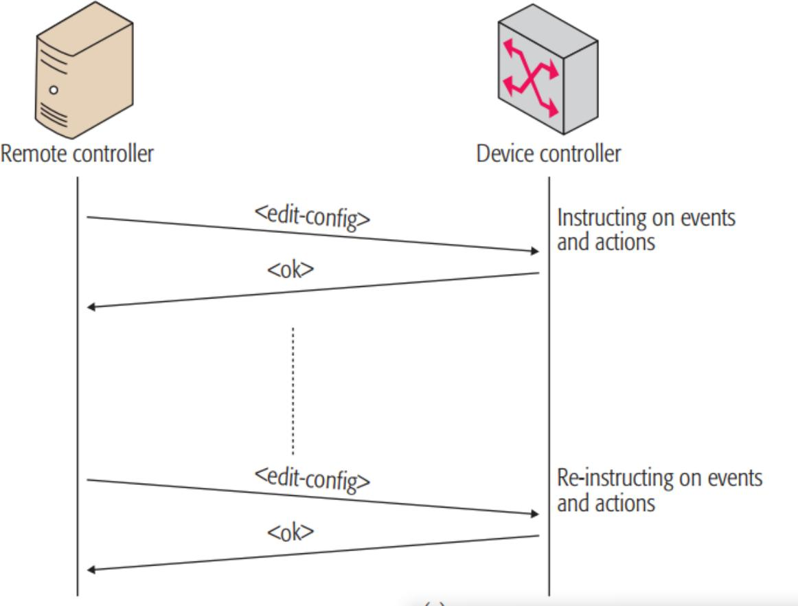
Figure 6.1.3 NETCONF exchange message where Remote Controller is centralized network controller (example ONOS) and Device Controller is the transponder device. [8]
