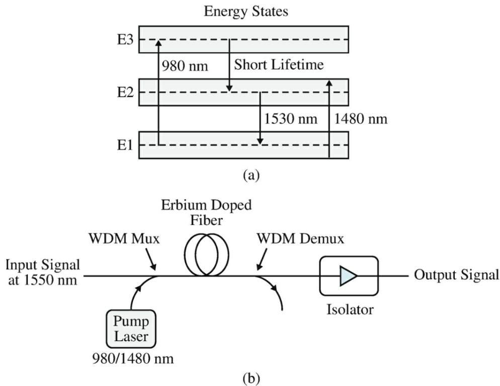
Figure 2.2.3.1 EDFA Amplification: (a) energy level, (b) architecture [5]
