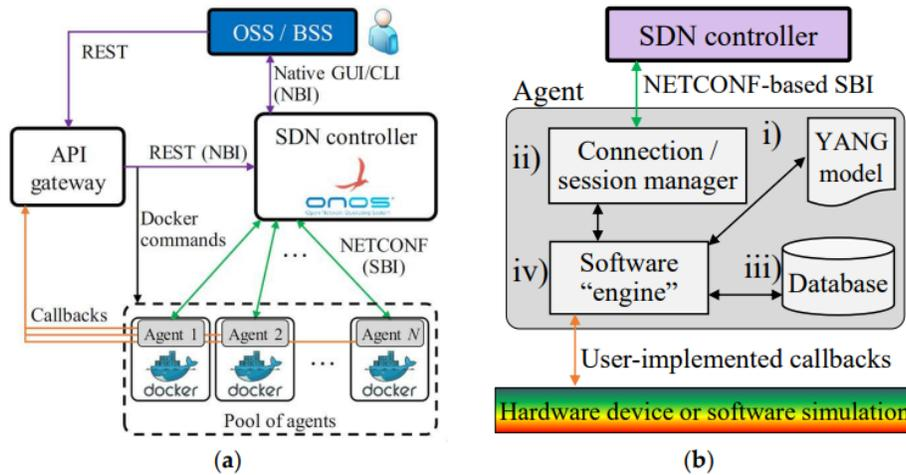
Figure 5.3.2 (a) Architecture (b) Detail agent view [35]
