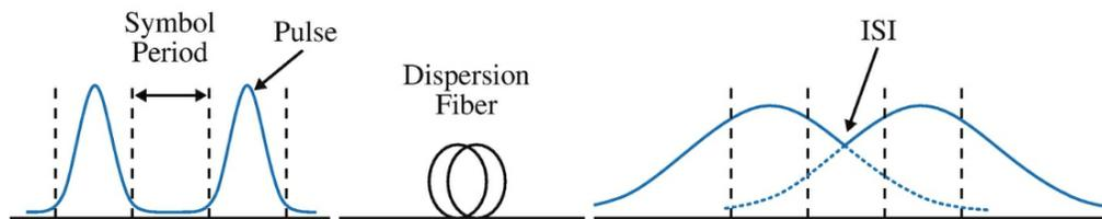
Figure 2.2.5.1.1 Effects of Chromatic Dispersion on signal propagation [5].
