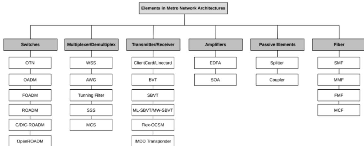
Figure 2.1.2: Main equipment involved in optical network infrastructures [10]
