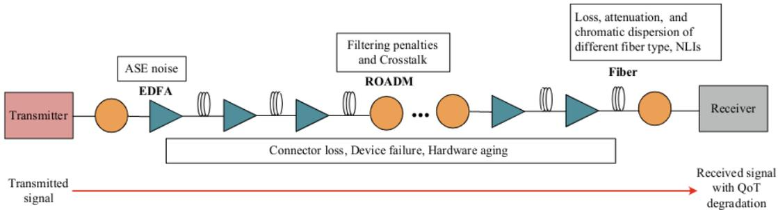
Figure 4.1 Signal transmission suffering impairment in light-path [36]
