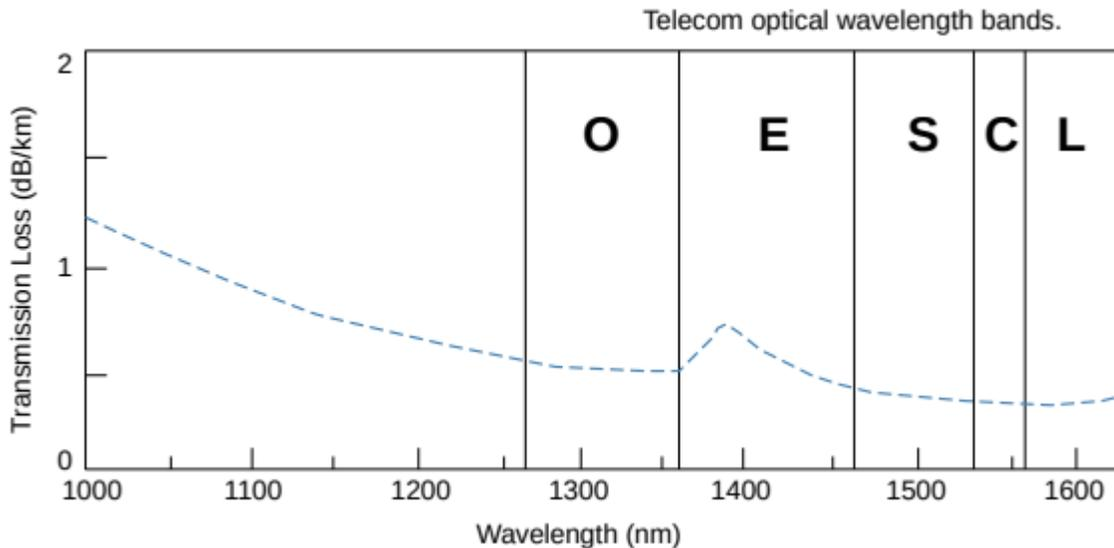
Figure 2.1.3: Behavior of the fiber transmission loss as the wavelength varies [10].
