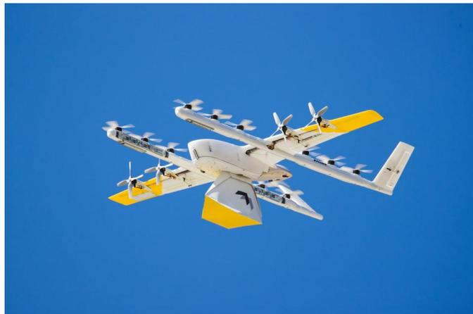
**Figure 2.2:** Delivery UAV from Alphabet's Wing company [7]
