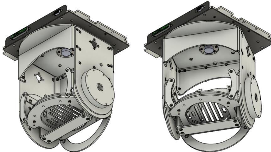
Figure 2.2: The PAN rotation joint
