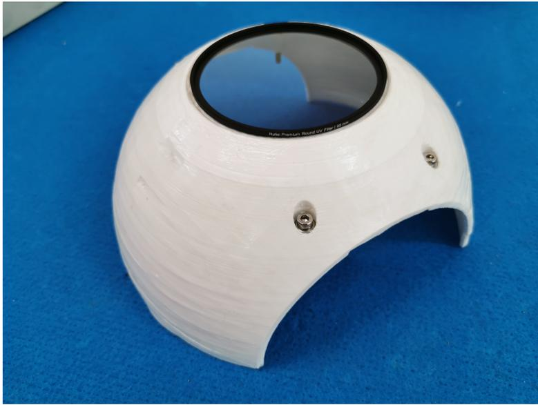
Figure 6.2: The front sphere of the aerodynamic fairing
