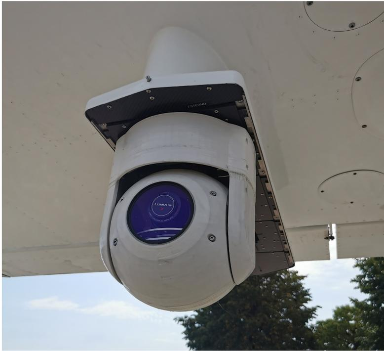
Figure 9.2: The *SmartGimbal* installed on the *SmartBay*
