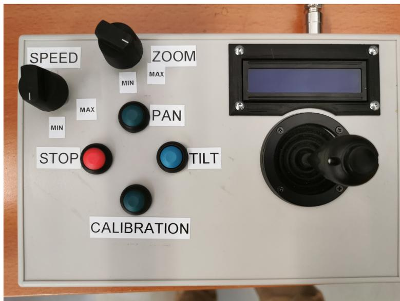
Figure 7.9: The console "test configuration"
