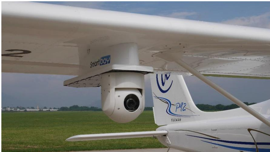
Figure 1.4: The *SmartBay* platform with the *SmartGimbal* device installed
