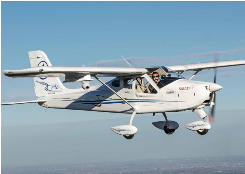
Figure 1.5: The P92 plane with, on the right wing, the *SmartBay* pylon
