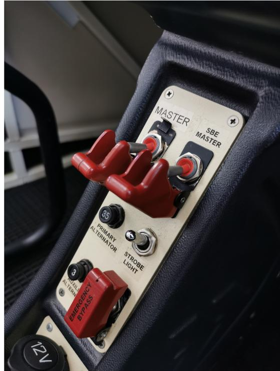
Figure 7.3: The *SmartBay* master switch
