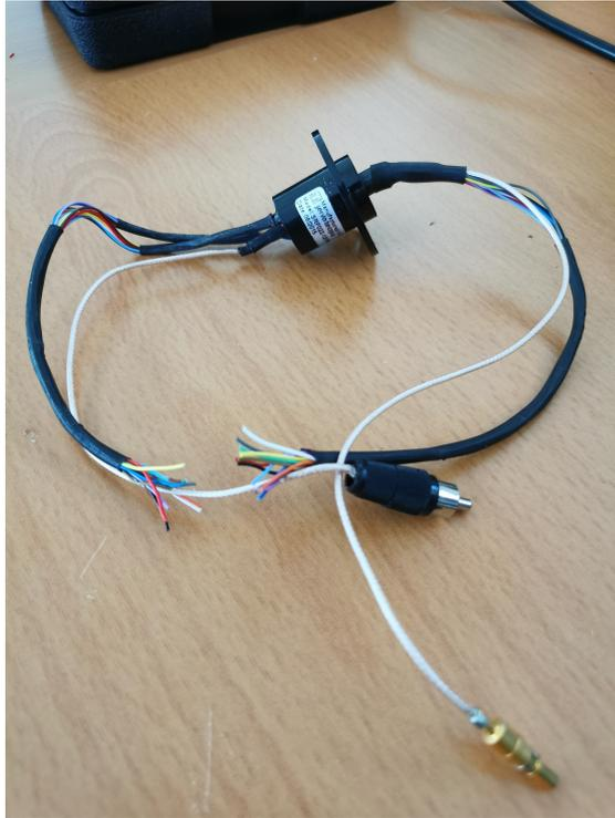
Figure 2.5: The *SmartGimbal* slip ring
