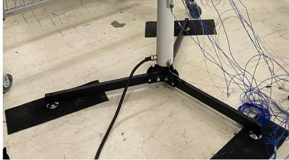
Figure 5.20: Wind turbine base and supporting tripod
