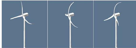
Figure 1.6: 1<sup>st</sup> rotor flapwise modes [6]
