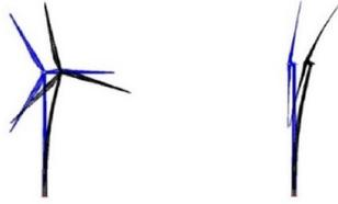
Figure 1.3: 1<sup>st</sup> tower bending modes [13],[5]
