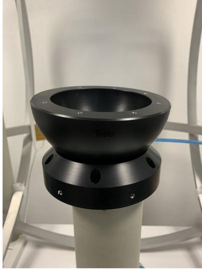
**Figure 3.5:** Air Bearing system implemented in  $\mu 3S$  facility consisted of an articulated stand (Ferronato® ULTAS-1 from Serviciencia, Toledo, Spain), a spherical air bearing (150mm of diameter) by Physical Instrumentns and tabletop-style platform
