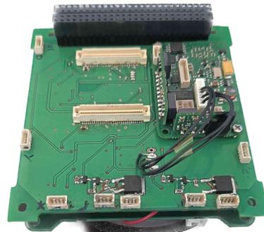
**Figure 6.22:** ADCS's IMU connections
