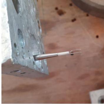
**Figure 3.9:** Hot wire anemometer is the sensor used to measure the velocity of a fluid
