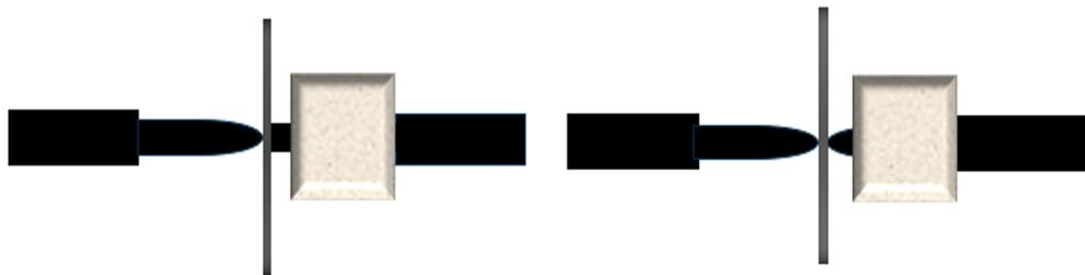
**Figure 4.7:** Flat (left) or round (right) thermocouples are used to take measurements of the back temperature
