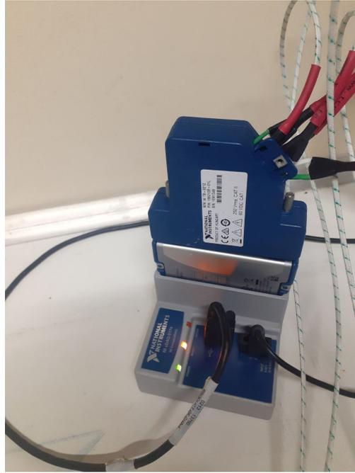
**Figure 3.13:** Acquisition system used for the voltage of the thermocouples
