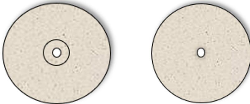
**Figure 4.8:** The insulator (macor) with (left) and without(right) air chamber
