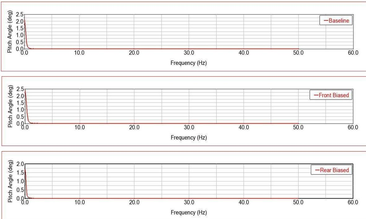
Figure 48. Pitch angle magnitude in the frequency domain
