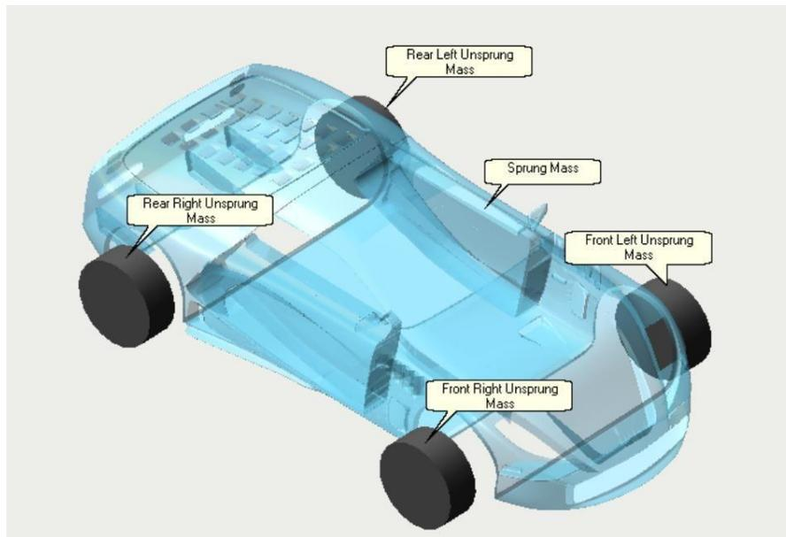
Figure 11. Vehicle model in VI-CRT. From [21]
