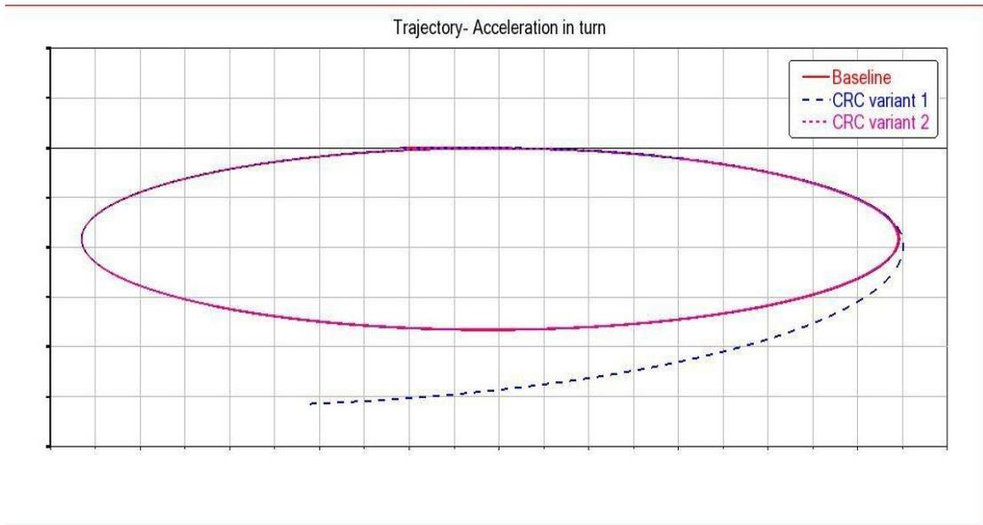
Figure 35. Trajectory during an acceleration in turn test. While the baseline and the less understeering variant manage to maintain the trajectory, the understeering variants struggles and goes out of track.
