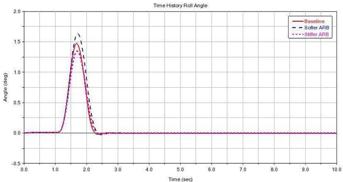
Figure 31. Time history of roll angle in an impulse steer test
