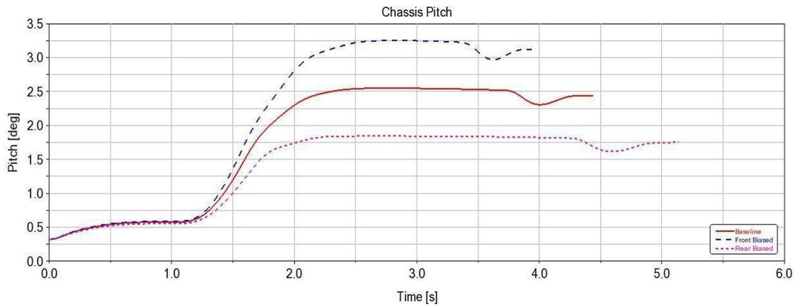
Figure 27. Time history of pitch angle in a straight and braking maneuver
