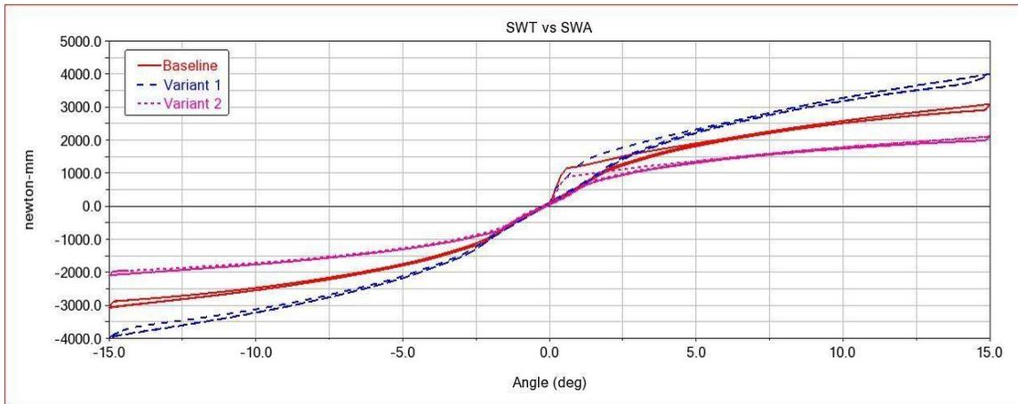
Figure 55. SWT versus SWA in an On Center Weave test. Variant 1 has a stiffer torsion bar compared to the Baseline, while Variant 2 has a softer one.
