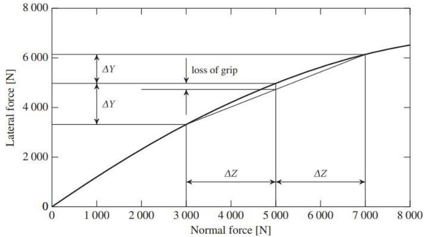
Figure 13. Lateral force exerted by the tire with respect to the normal force applied on it, from [13].
