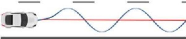
Figure 50. On Center Weave Test. Image courtesy of [54].
