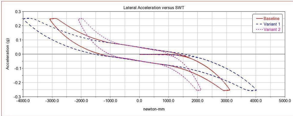
Figure 56. lateral Acceleration versus SWT in an On Center Weave test. Variant 1 has a stiffer torsion bar compared to the Baseline, while Variant 2 has a softer one.
