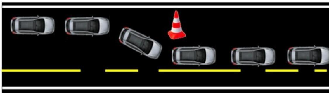
*Figure 29. The trajectory of a vehicle subjected to an impulse steering wheel angle input [38].*
