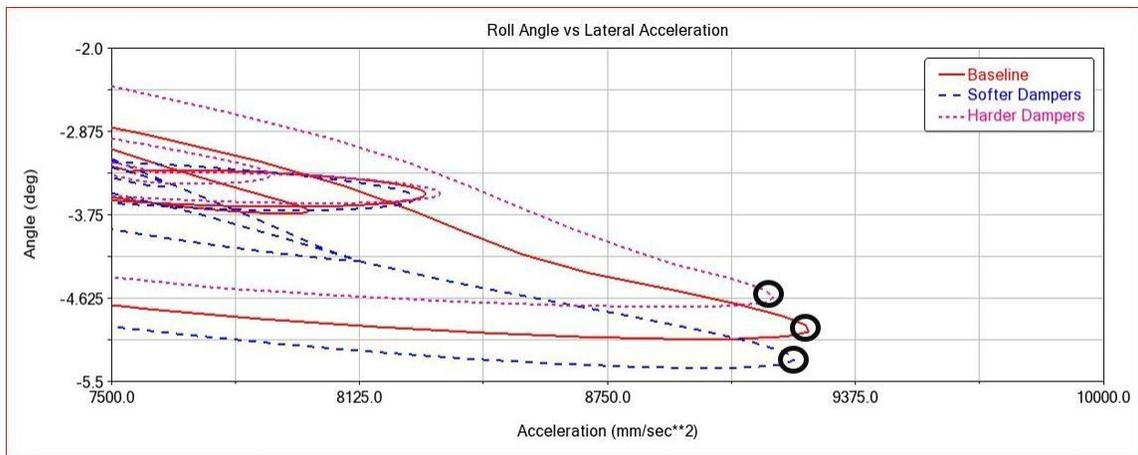
Figure 42. Roll angle versus lateral acceleration. The roll gradient is measured in the circled points (peak acceleration)
