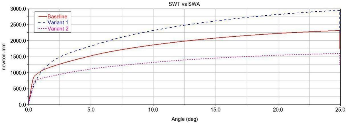
Figure 54. SWT vs SWA in a Transition Test. Variant 1 has a stiffer torsion bar compared to the Baseline, while Variant 2 has a softer one.
