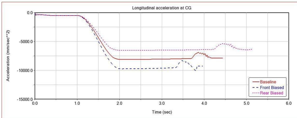
Figure 47. Longitudinal acceleration experienced at the vehicle CG during an open loop braking maneuver
