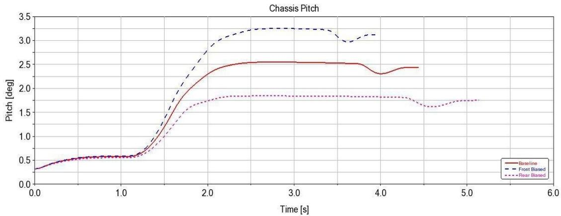
Figure 46. Pitching angle during open loop braking maneuver
