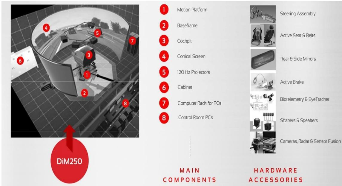
Figure 3. DiM250 simulator ecosystem. by VI Grade [10].
