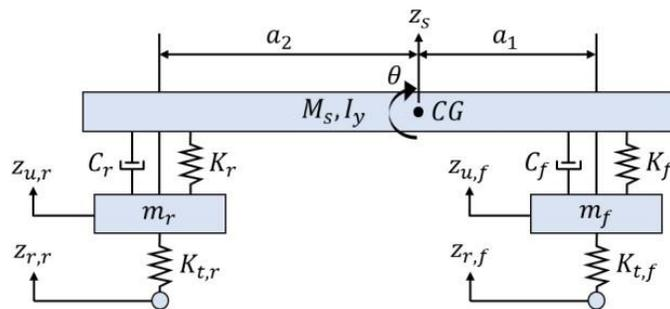
Figure 10. Bicycle Vibrating Model, from [20].
