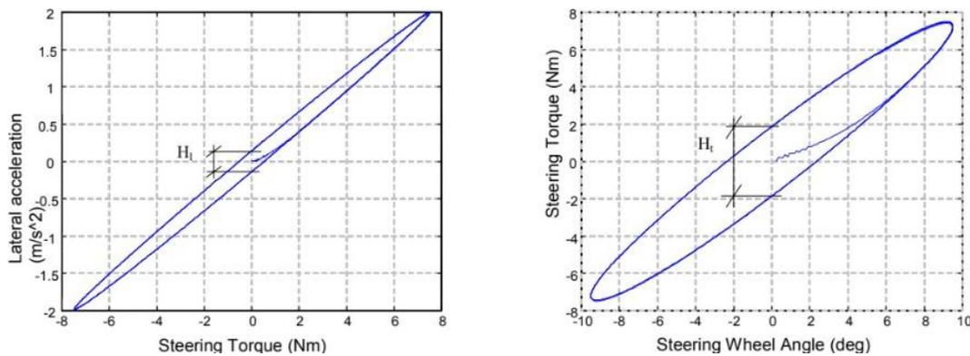
Figure 25. Lateral acceleration versus SWT and SWT versus SWA, from [41].
