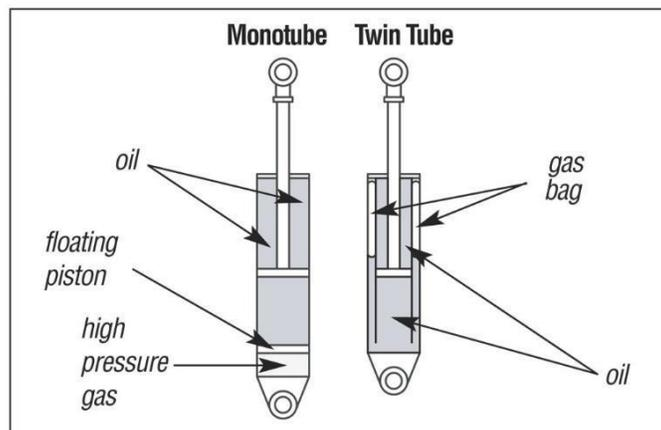
Figure 20. Two different damper designs: monotube (more expensive) and twin tube (cheaper), from [32]
