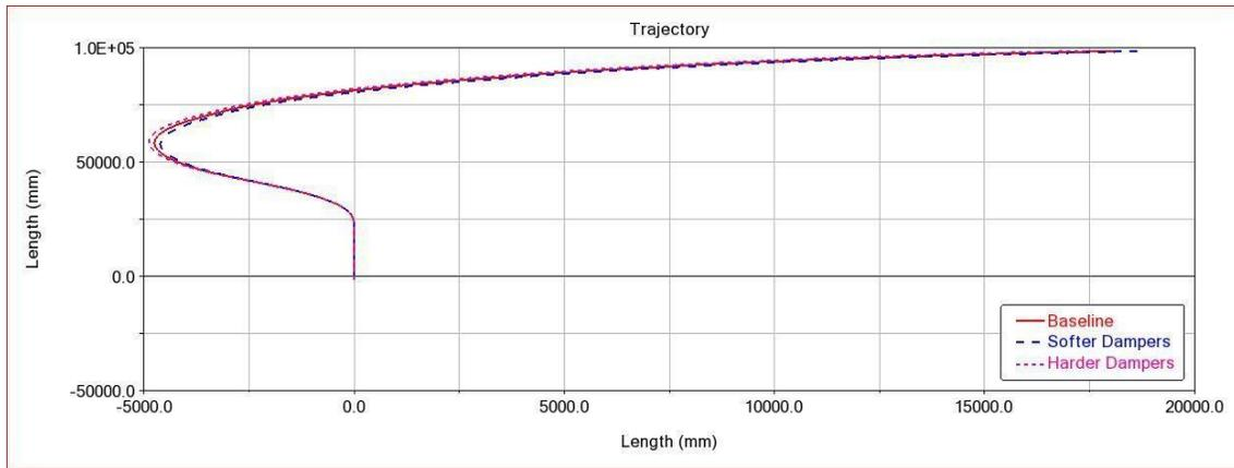
Figure 43. Trajectory in the fishhook test. The x-axis is the displacement in the longitudinal direction, the y-axis in the lateral one.
