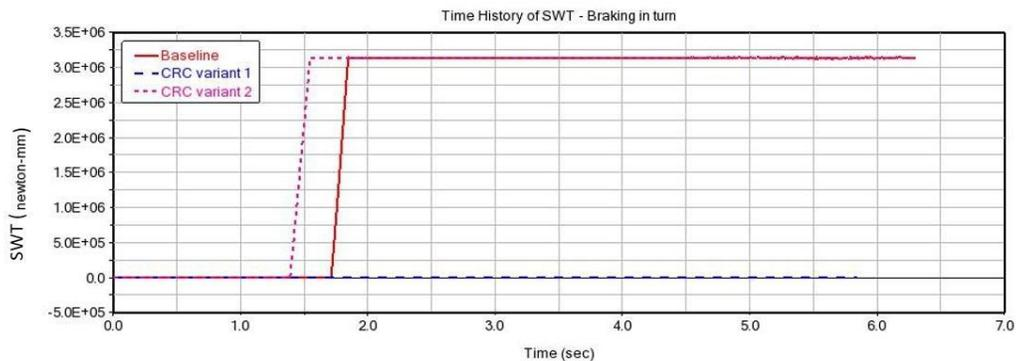
Figure 36. SWT versus time in a brake- in- turn simulation. Variant 1 has a stiffer rear ARB, while Variant 2 has a stiffer front ARB.
