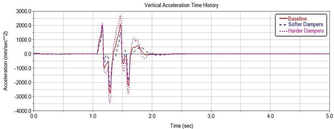
Figure 62. Vertical Acceleration at body CoG
