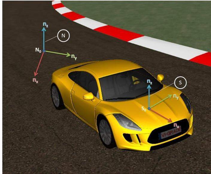
Figure 5. Global and Vehicle Reference System. From [16]
