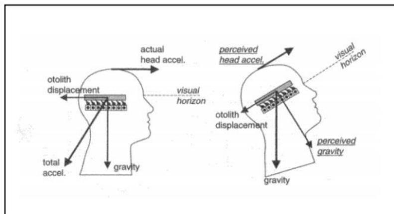
Figure 66. Tilt coordination technique, from [55].
