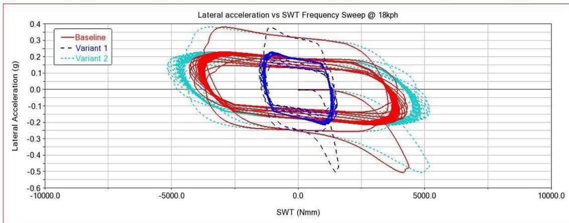
Figure 61. Lateral acceleration vs SWT in a Frequency Sweep Test run at 18 kph.
