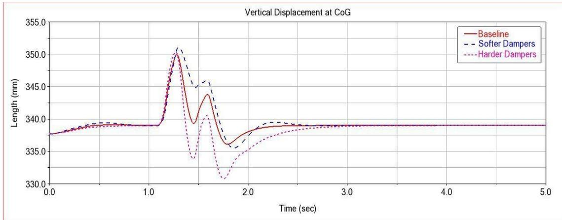
Figure 63. Vertical displacement at body CoG
