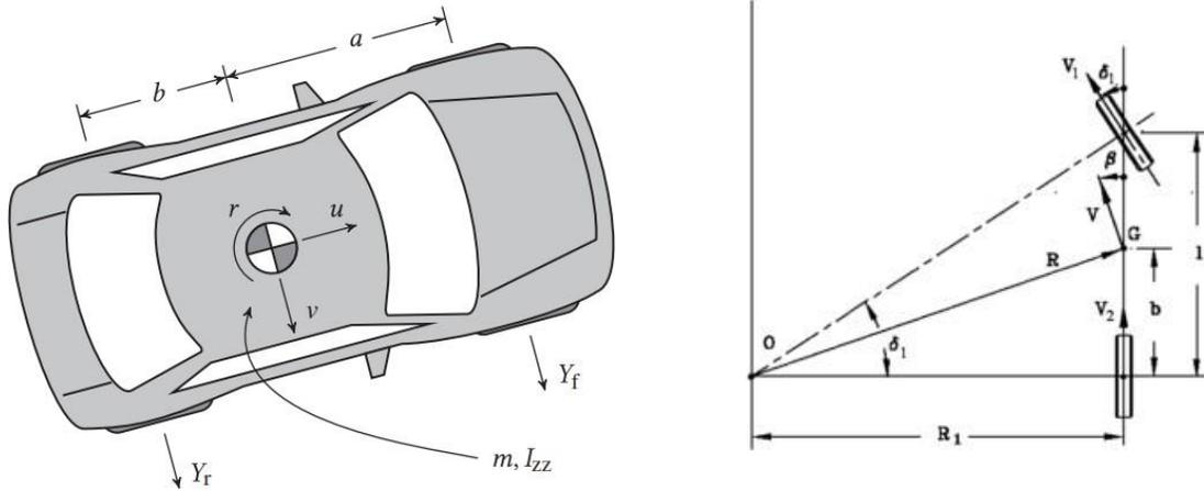
Figure 7. Yaw Plane model, from [13] and bicycle model, from [19].
