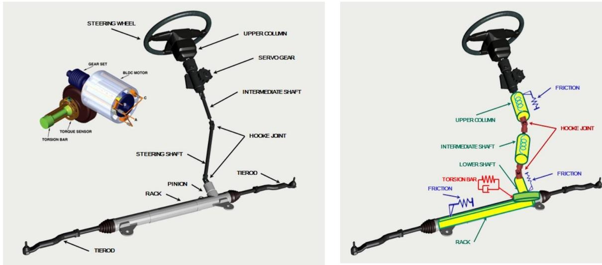
Figure 17. Advanced steering system model - Rack-and-Pinion, from [29].
