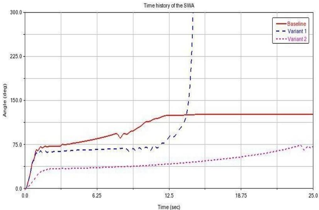
Figure 33.SWA versus time in a CRC test. Variant 1 has a stiffer rear ARB, while Variant 2 has a stiffer front ARB.
