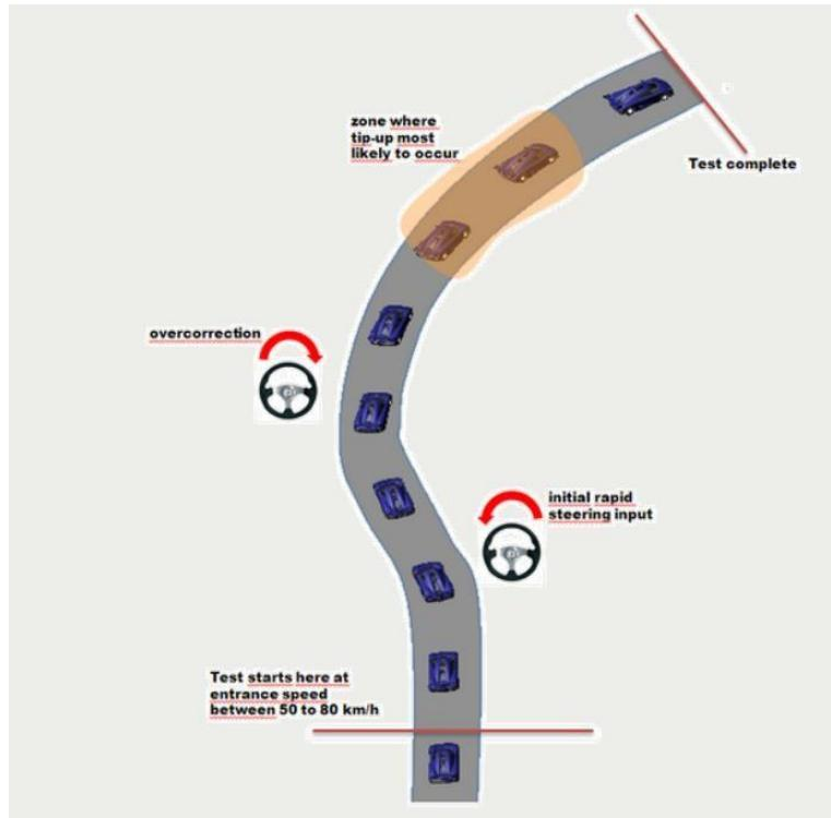
Figure 38. Fishhook test, picture taken from [53].
