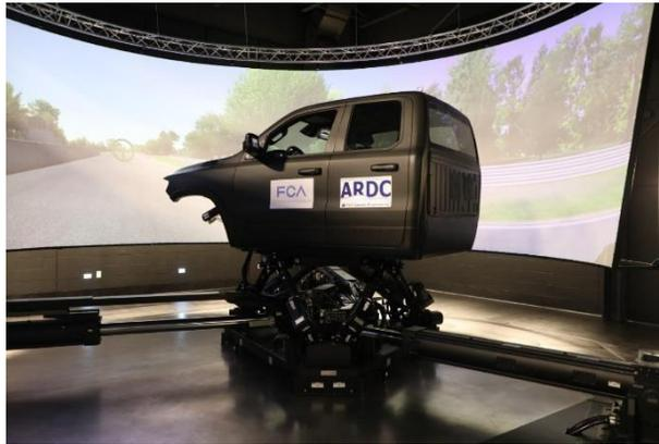
*Figure 4. DiM 250 Dynamic Simulator as installed at the Automotive Research and Development Center in Windsor, Ontario [12].*
