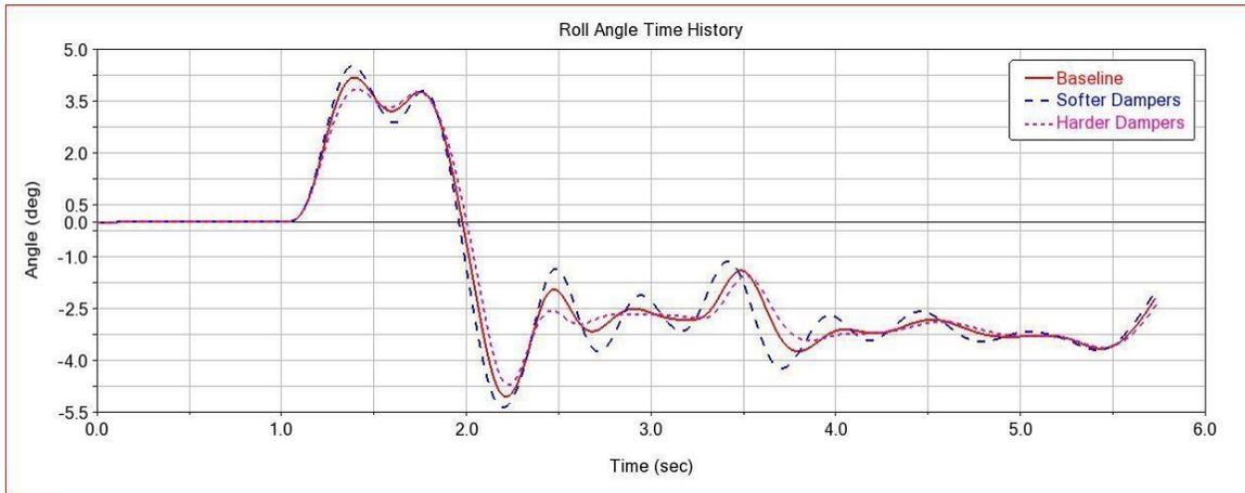
Figure 41. Roll Angle in a fishhook maneuver
