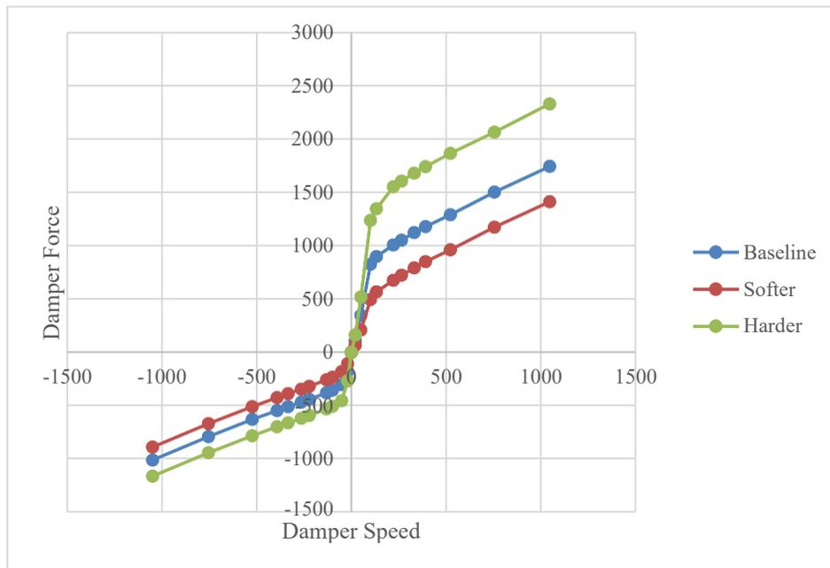
Figure 40. Rear dampers characteristic curve.
