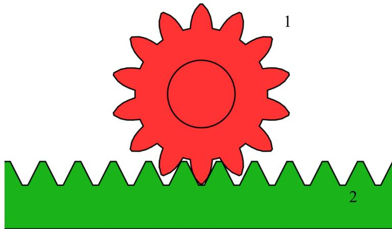
*Figure 16. Rack and pinion, from [27].*
