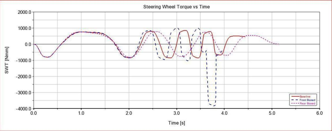
Figure 49. Time history of the SWT during an open brake maneuver. The Front Biased variant reaches higher peaks, which might make it harder for the driver to keep control of the car during the maneuver.
