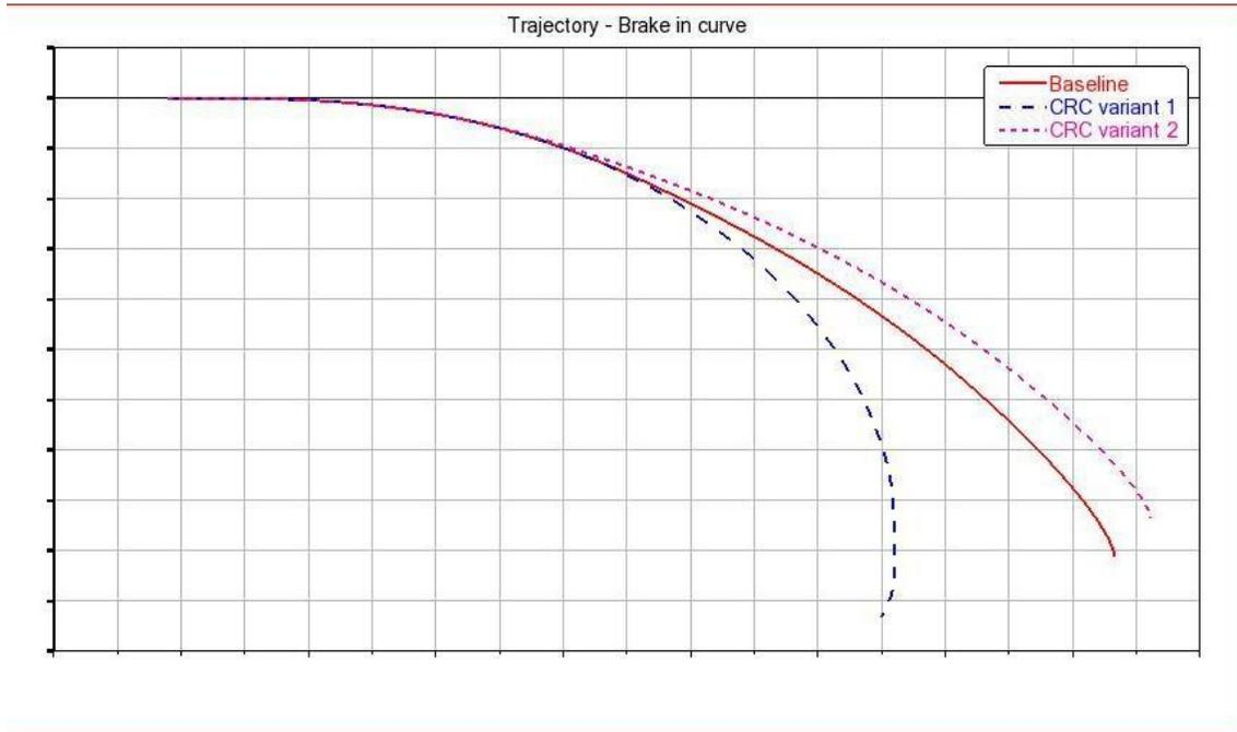
Figure 37. Trajectory in a brake-in-turn maneuver. Variant 1 has a stiffer rear ARB, while Variant 2 has a stiffer front ARB.
