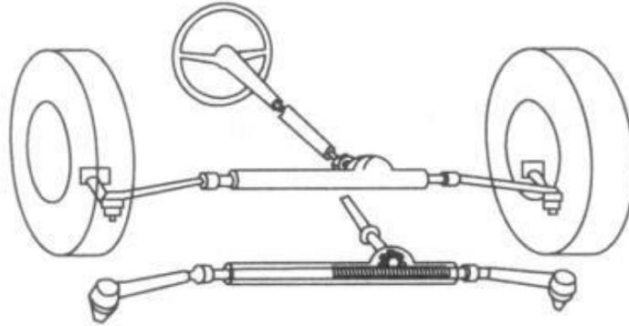
*Figure 15. Rack- and- pinion linkage, from [26]*
