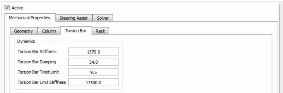
Figure 18. Torsion bar panel, from [30].
