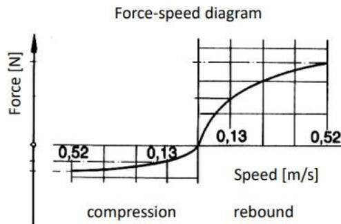
Figure 19. Force versus Speed characteristics, from [31]
