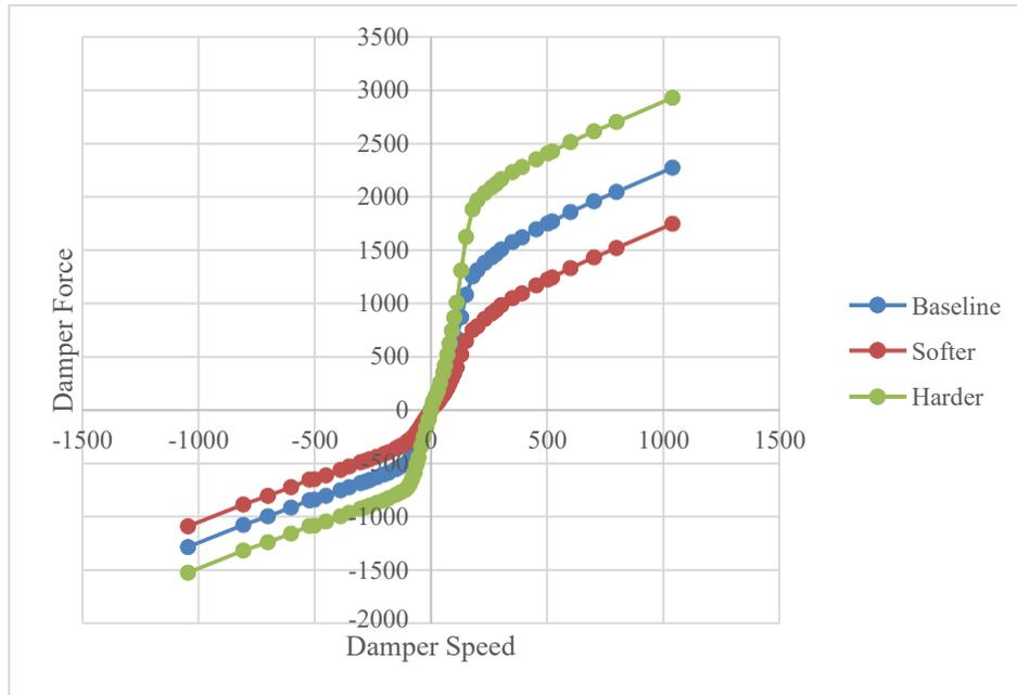
Figure 39. Front dampers characteristic curve.
