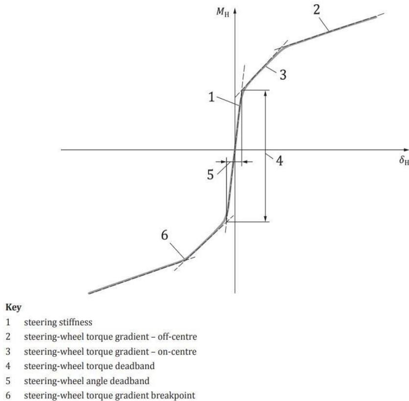
Figure 26. SWT versus SWA in ISO Transition Test [36]
