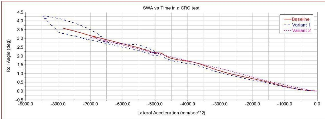
Figure 34. Roll angle versus Lateral Acceleration in a CRC test. Variant 1 has a stiffer rear ARB, while Variant 2 has a stiffer front ARB.
