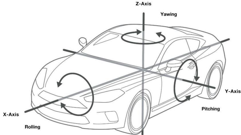
Figure 6. Motions about the three axes of the reference frame of a vehicle. From [17]
