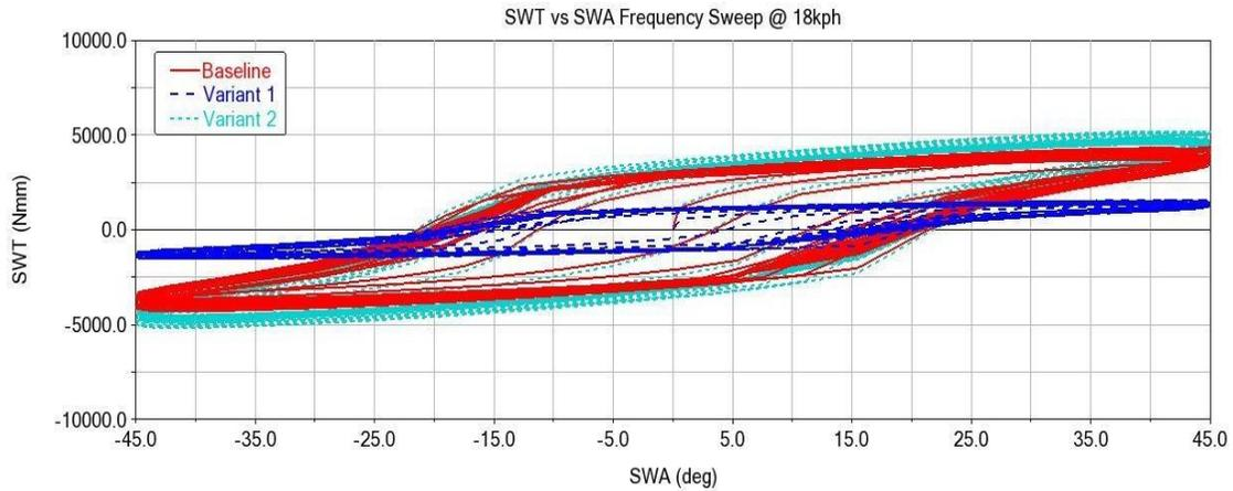
Figure 60. SWT vs SWA in a Frequency Sweep Test run at 18 kph.
