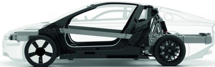
Figure 52: Carbon Monocoque Structure
