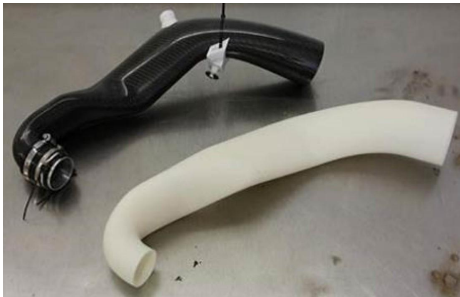
Figure 4.15 The composite turbo inlet duct by Indirect AM, source: Stratasys [59]
