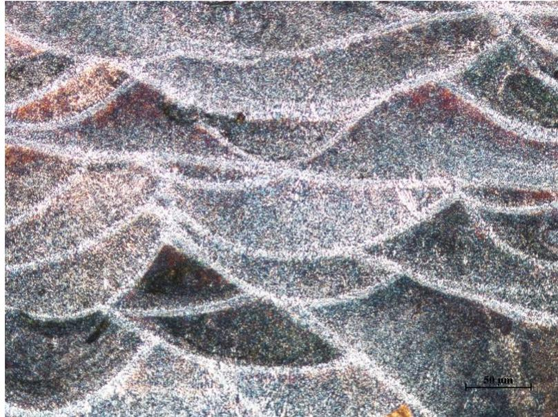
**Figure 33** Melt pools, magnified view sample P
