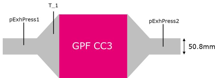
Figure 3-23 – Visual representation of the GPF ATS brick testing conditions
