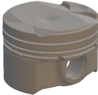
Figure 2-29 – PHOENICE new piston design with CR 13.6
