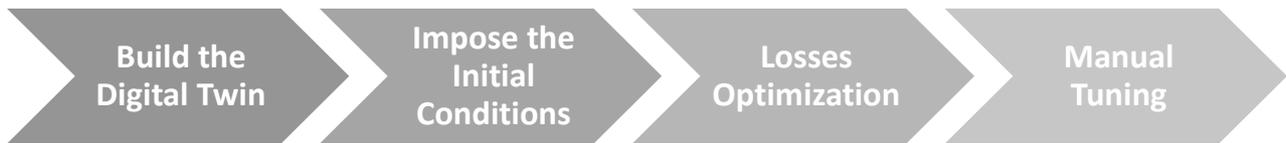
Figure 3-35 – Coolers' Calibration Procedure Flowchart
