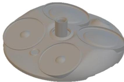
Figure 2-30 – PHOENICE new cylinder head design
