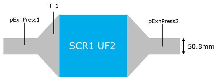
Figure 3-31 – Visual representation of the SCR<sub>1</sub> ATS brick testing conditions
