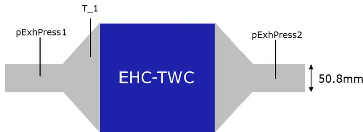
Figure 3-11 – Visual representation of the EHC-TWC<sub>1</sub> ATS brick testing conditions
