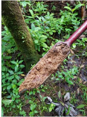
**Figure 3:** Dutch auger tool
