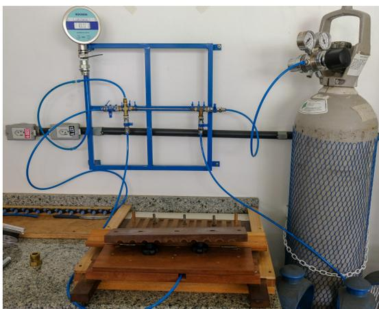
**Figure 2.9:** Cleaning and evacuation system
