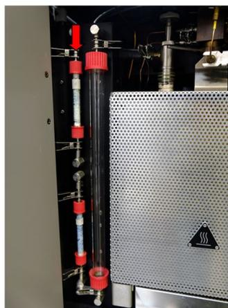
**Figure 3.9:** Analyzer drying cylinders
