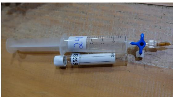
Figure 2.8: Syringe and vial for GHGs
