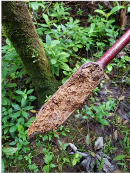
**Figure 3.3:** Dutch auger tool
