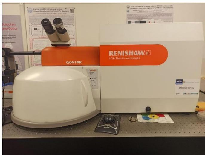
*Figura 18: Microscopio Raman confocale inVia™*
