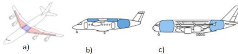
Figure 1-9 - Fuel tank locations for kerosene and future medium or large aircrafts. a) Conventional; b) c) Hydrogen
