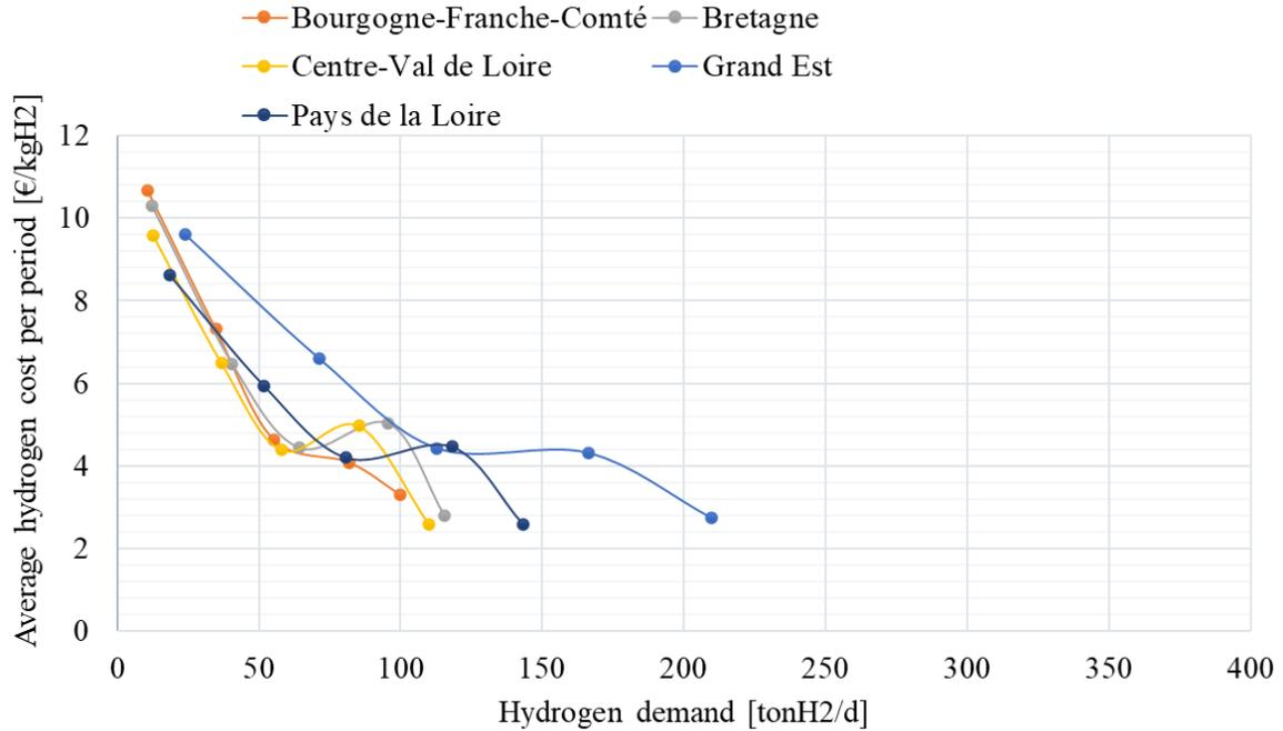
Figure 6.12: Average hydrogen cost in the regions with low hydrogen demand in the Hydrogen + scenario
