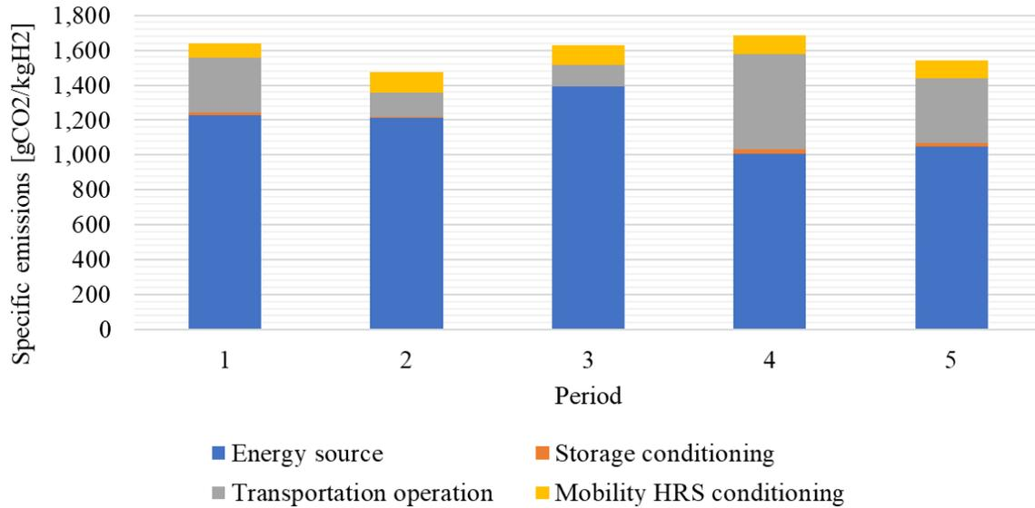
Figure 6.10: Specific emissions in Auvergne-Rhône-Alpes in the Hydrogen + scenario
