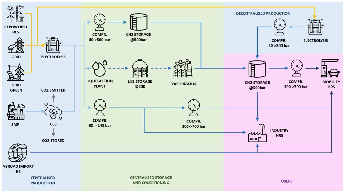
Figure 5.2: Elements of the HSC when the product is produced and consumed in the same grid
