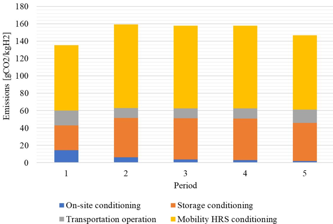
Figure 6.20: Specific emissions in Auvergne-Rhône-Alpes in Hydrogen + scenario, emission minimisation
