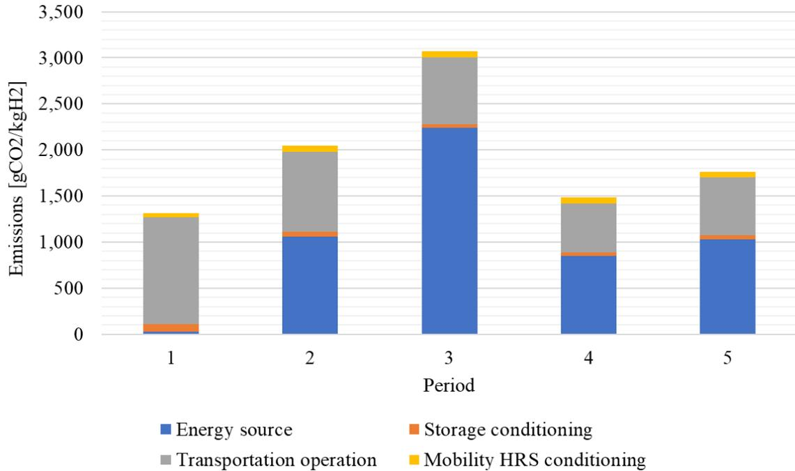
Figure 6.17: Specific emissions in Auvergne-Rhône-Alpes in the Hydrogen + scenario, post-war alternative
