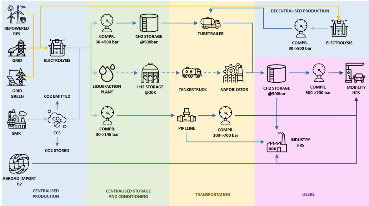
Figure 5.1: Elements of the HSC when transporting product from one grid to another
