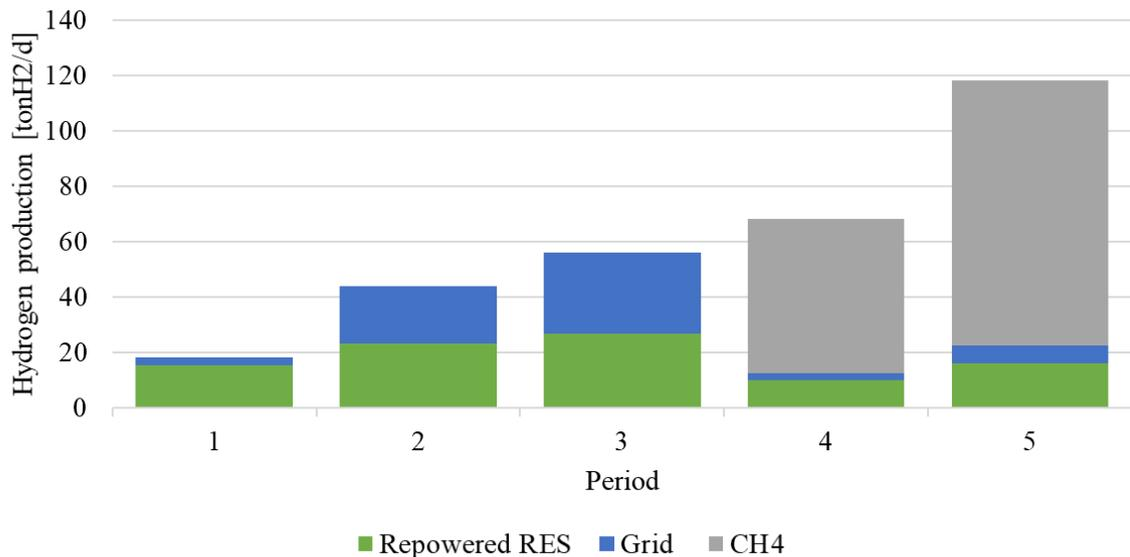
Figure 6.2: Hydrogen production per energy source in Auvergne-Rhône-Alpes in the Reference scenario
