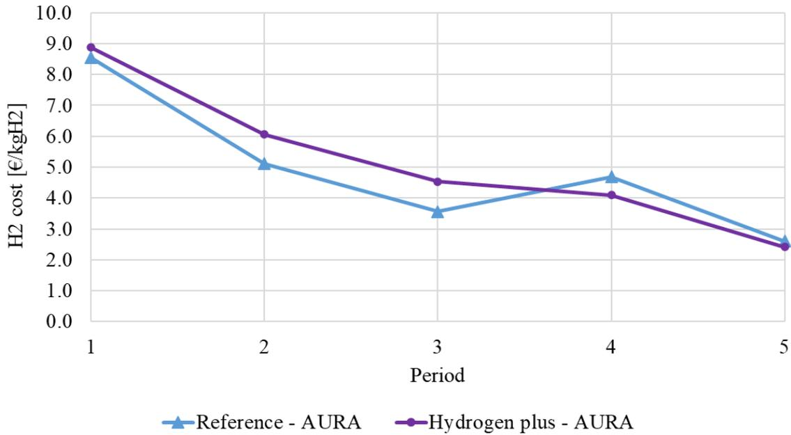
Figure 6.9: Final hydrogen cost comparison between Reference and Hydrogen + case studies for the Auvergne-Rhône-Alpes region
