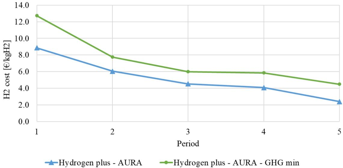
Figure 6.19: Final hydrogen cost comparison between cost minimisation and emission minimisation case studies in the Hydrogen + scenario
