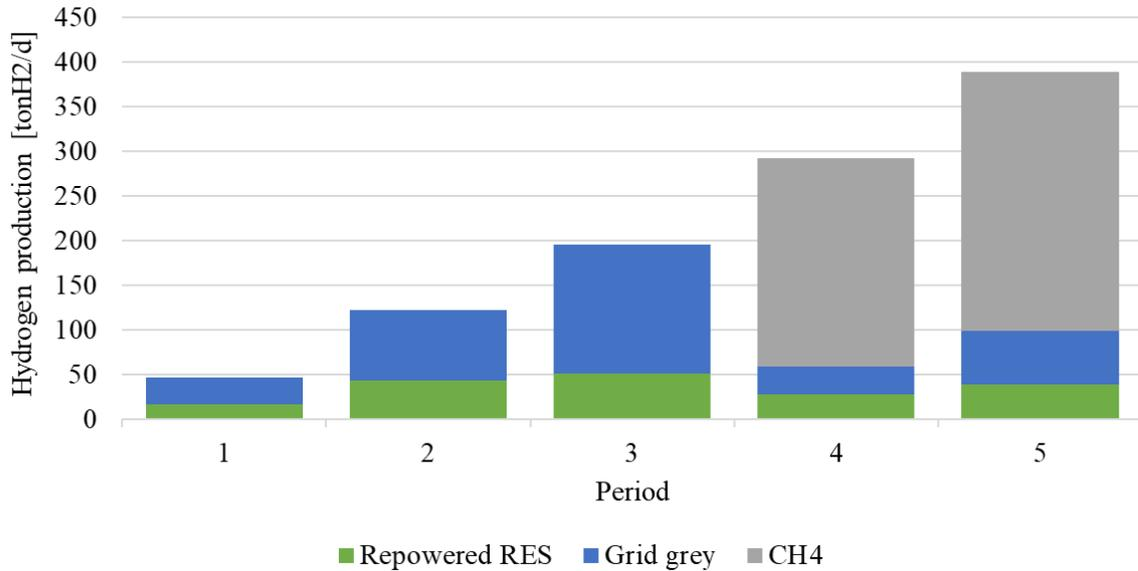
Figure 6.6: Hydrogen production per energy source in Auvergne-Rhône-Alpes in the Hydrogen + scenario
