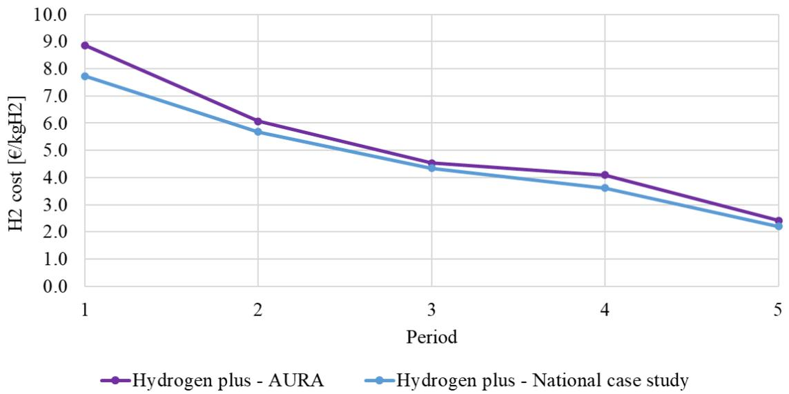
Figure 6.25: Final hydrogen cost comparison between the AURA and national case studies in the Hydrogen + scenario
