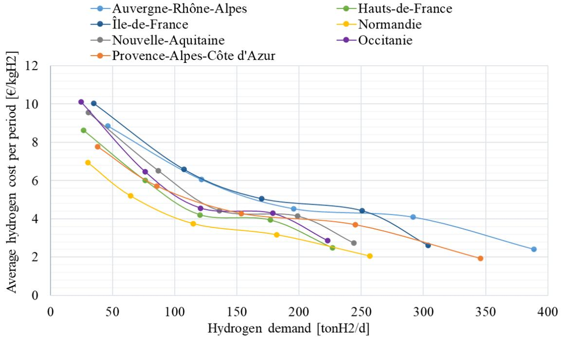
Figure 6.11: Average hydrogen cost in the regions with high hydrogen demand in the Hydrogen + scenario
