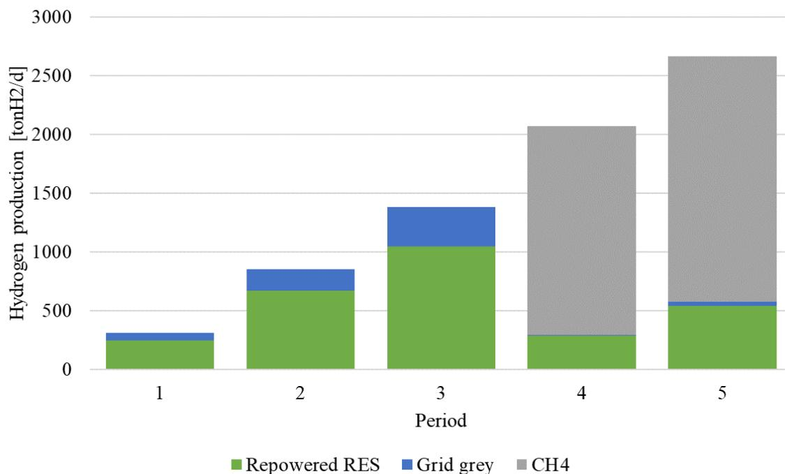
Figure 6.21: Hydrogen production per energy sources used in National case study in the Hydrogen + scenario
