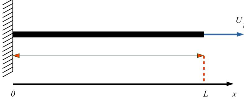
Figure 1.1: A 1D tensile test representation: the specimen is clamped at  $x = 0$  and subjected to an imposed displacement  $u_t(x = L) = U_t$  (i.e. a Dirichlet boundary condition) at  $x = L$ .
