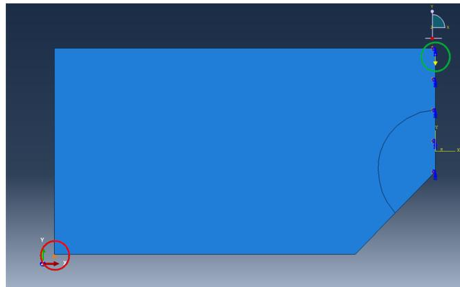
Figure 2.5: Typical boundary condition setup on TPB samples. A XSYMM condition over the right side and a  $u_y = 0$  condition on the lower contour leftmost point (circled in red) are imposed. The applied concentrated force over the top contour (circled in green) is also displayed.
