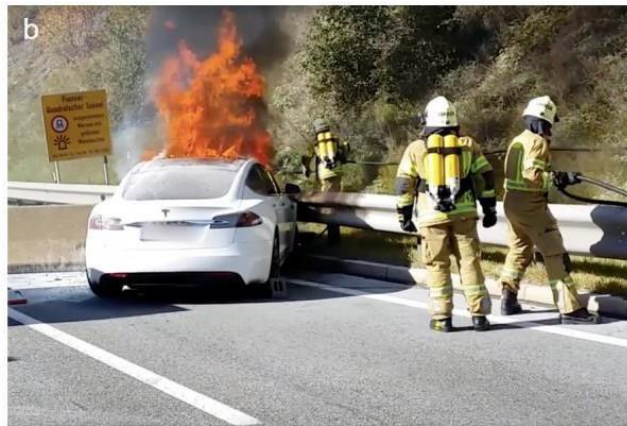
FIGURE 33 EXAMPLE OF A FIRE DUE TO A COLLISION [16]
