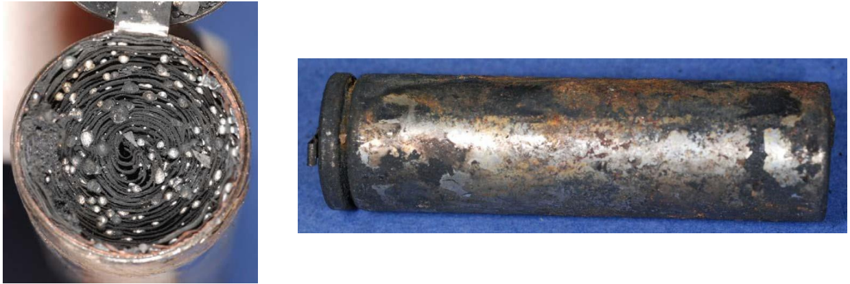
FIGURE 27 CONDITION OF A CYLINDRICAL CELL (18650) AFTER THERMAL RUNAWAY, THE RESOLIDIFICATION OF ALUMINIUM IS EVIDENT IN THE CROSS-SECTION [24]
