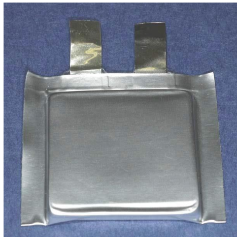
FIGURE 12 EXAMPLE OF POUCH STRUCTURE ENERGY STORAGE. [13]
