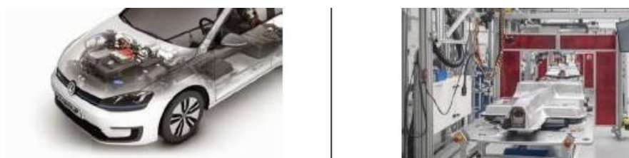
FIGURE 22 THE VOLKSWAGEN “E-GOLF” MODEL USES A T-SHAPED BATTERY PACK, IN ACCORDANCE WITH THE INTERIOR SPACES OF THE CAR (SEATS, FLOOR). 24.2 KWH [26] [27]
