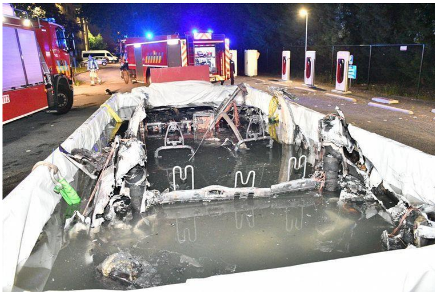
FIGURE 35 EXAMPLE OF COMPLETE IMMERSION IN WATER [37]
