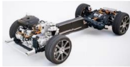
FIGURE 23 VOLVO XC60 MODEL, A PLUG-IN HYBRID EV, HAS A PARTIAL T-SHAPE LAYOUT AS ONE “BRANCH” IS THE BATTERY WHILE THE OTHER HAS THE FUEL TANK [26] [29]
