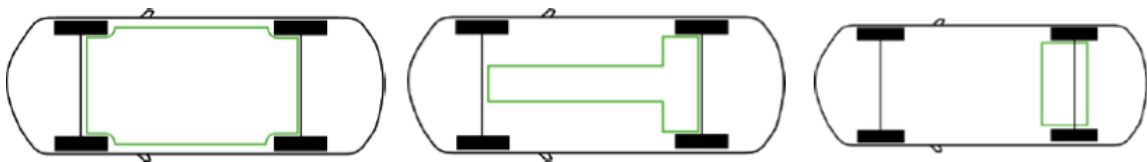
FIGURE 21 EXAMPLES OF BATTERY ARRAYS; FLOOR; "T" AND REAR AXLE [16]
