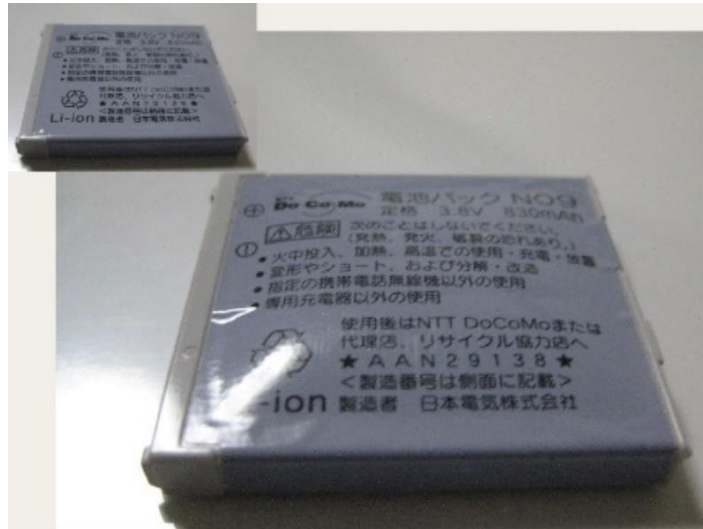
FIGURE 25 EXAMPLE OF A BATTERY INFLATED AS A RESULT OF GAS RELEASE [9]
