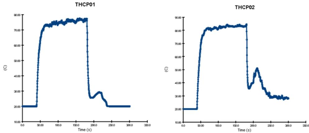
Figure 53. Temperature of thermocouples 01 and 02
