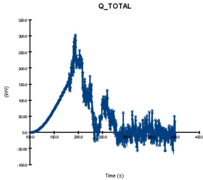
Figure 84. Total heat curve (EV case)
