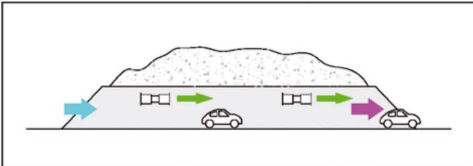
Figure 35. Longitudinal ventilation with jet fans in a road tunnel
