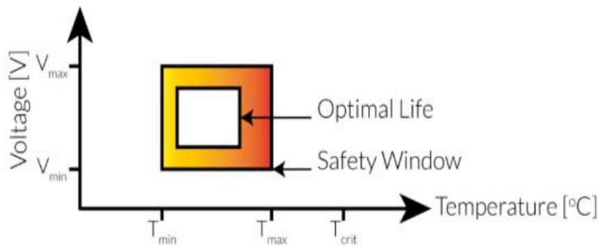
Figure 15. Working temperature window of Li-ion cells
