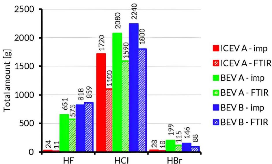
Figure 26. HF, HCl and HBr measuring test for ICEVs and BEVs
