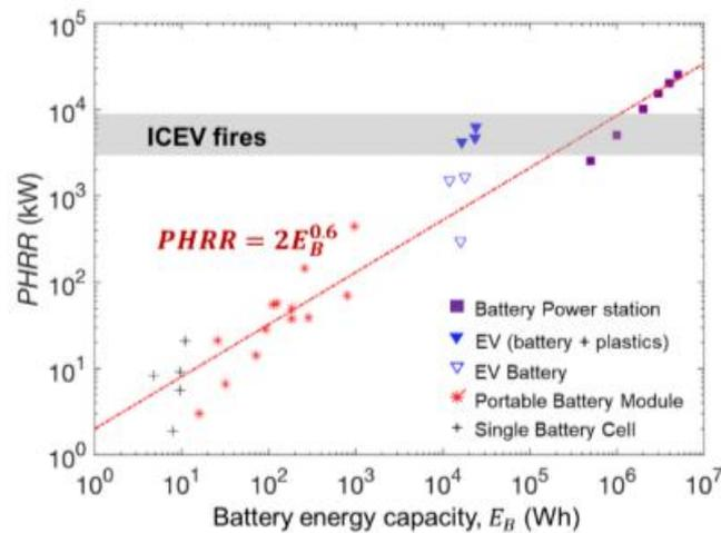
Figure 25. Peak heat release rate based on test results
