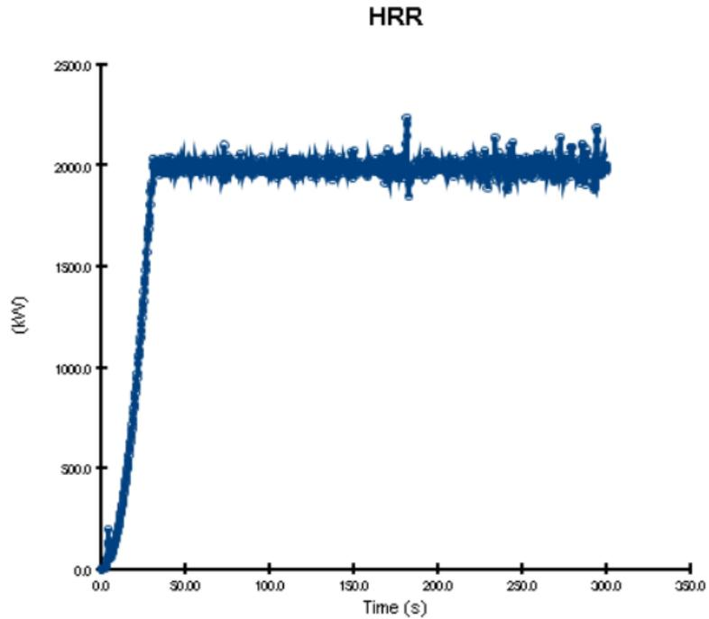
Figure 66. HRR curve for methane vehicle (second case)
