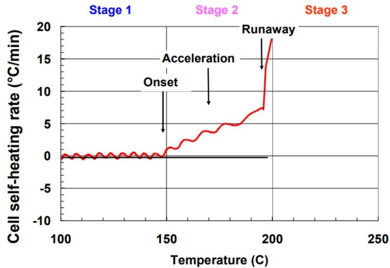
Figure 16. Evolution of temperature due to cell self-heating
