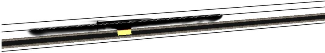
Figure 61. Stratification of the smoke in the first part of the simulation
