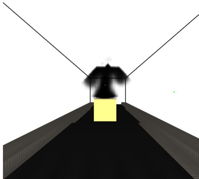
Figure 60. Smoke diffusion in the gallery after 15 seconds
