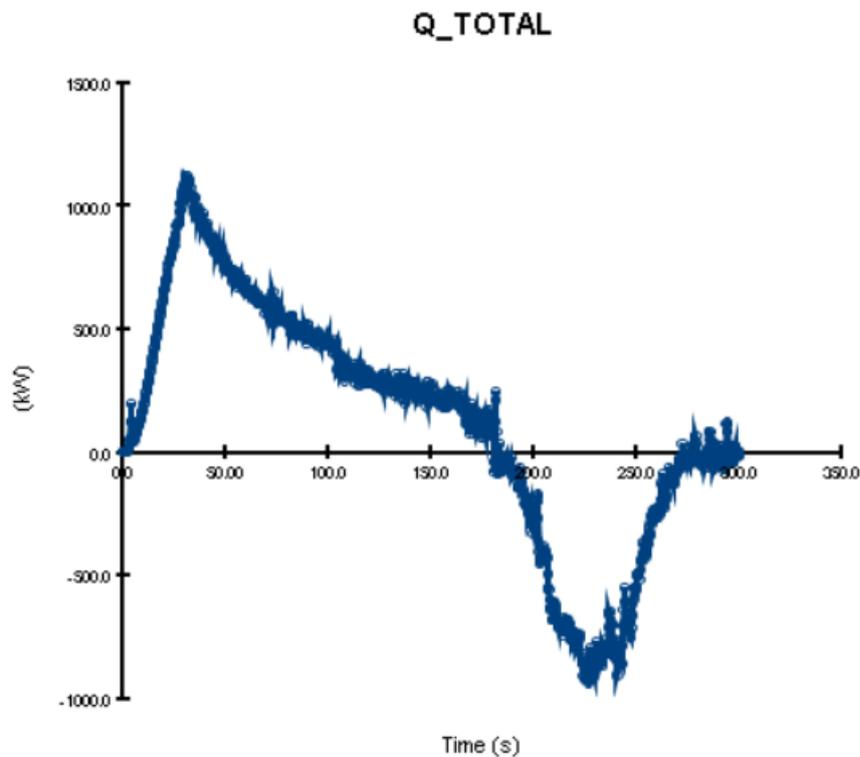
Figure 69. Total heat curve of a methane car (second case)
