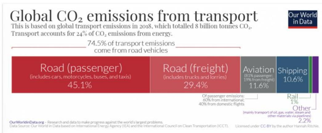
Figure 3. Global CO<sub>2</sub> emissions from transport
