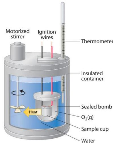
Figure 40. Calorimeter representation
