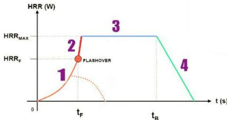
Figure 23. Ideal heat release rate curve
