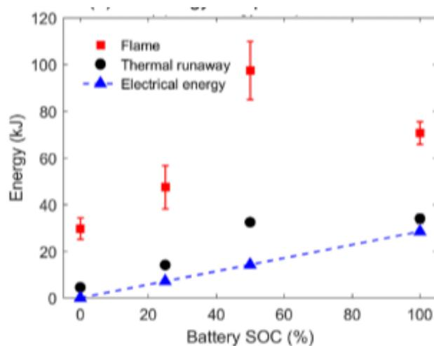
Figure 22. LIB energy comparison vs SOC
