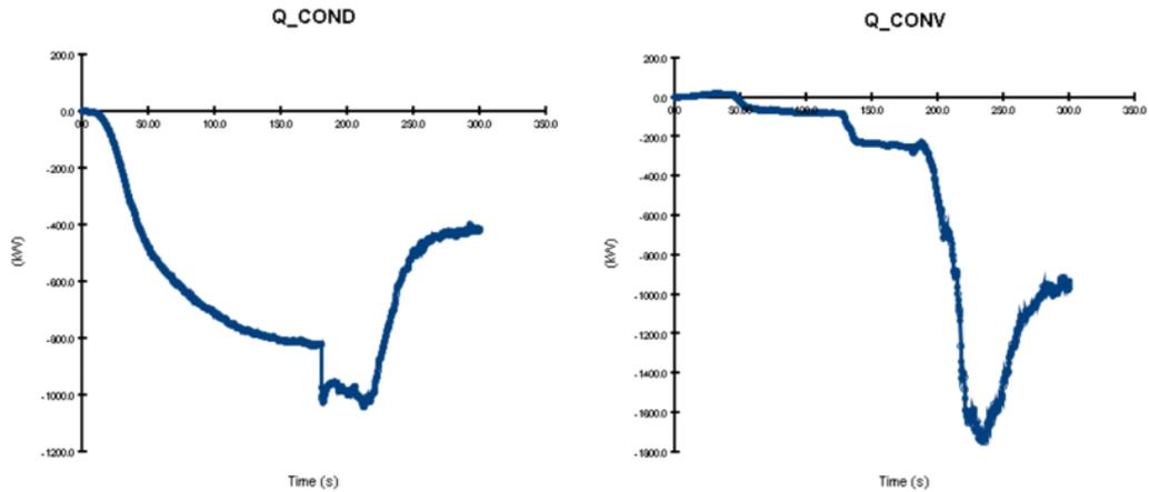
Figure 55. Heat released due to conduction and convection phenomena
