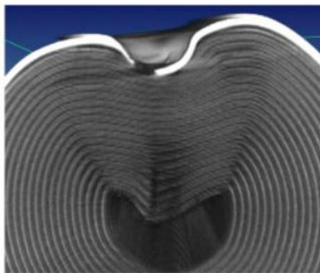
Figure 17. Mechanical abuse in Lithium-ion batteries
