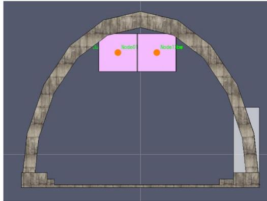
Figure 36. 2D view of modelled jet fans
