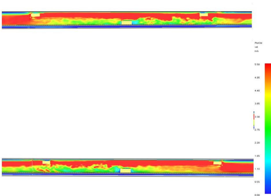
Figure 78. Gas velocity in the tunnel after 200s and 300s
