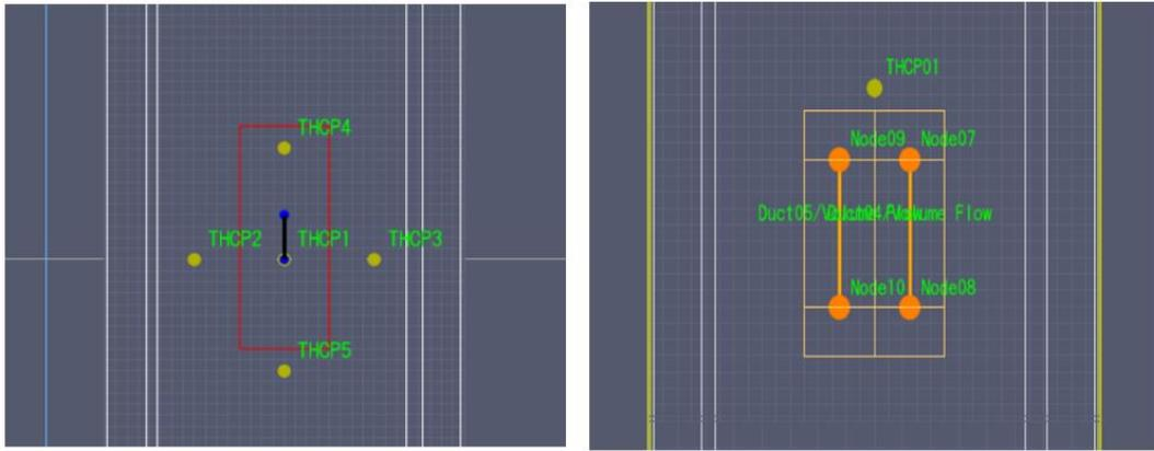
Figure 38. Position of thermocouples 1-2-3-4-5-01
