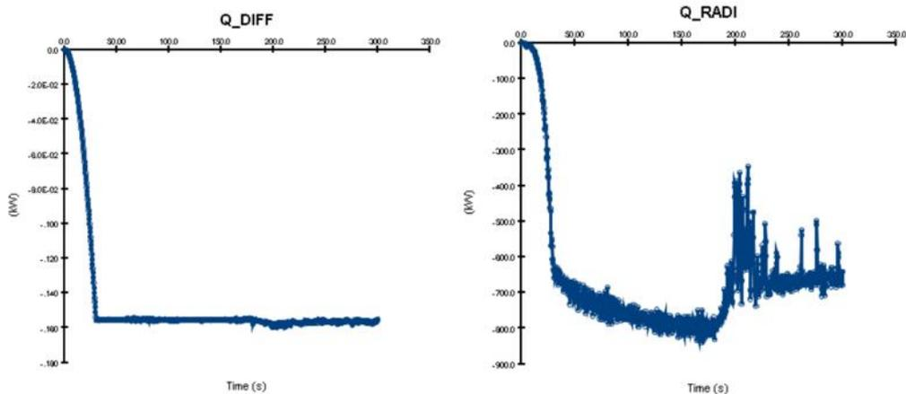
Figure 56. Heat released due to diffusion and radiation phenomena
