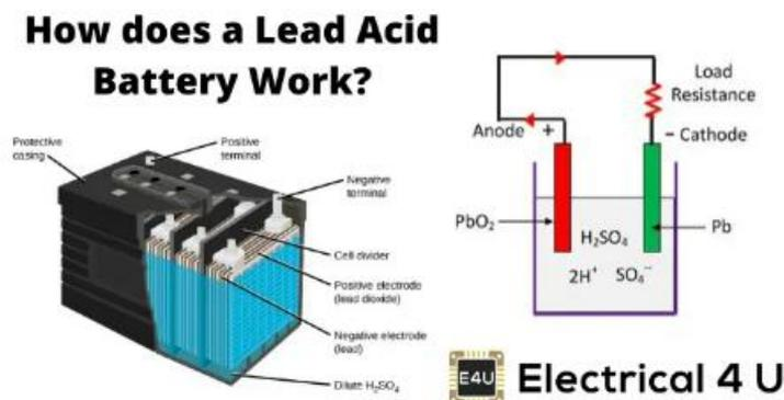
Figure 6. Representation of a Lead Acid battery
