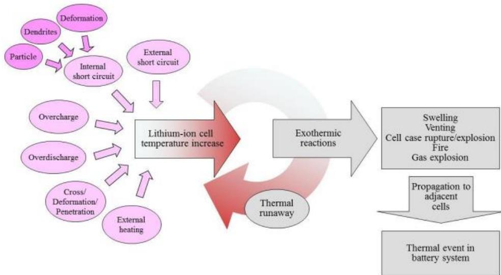
Figure 21. Schematization of thermal runaway causes and effects
