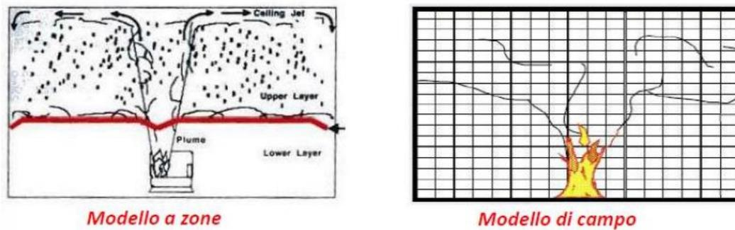
Figure 29. “Zone” and “Field” model in FDS simulations
