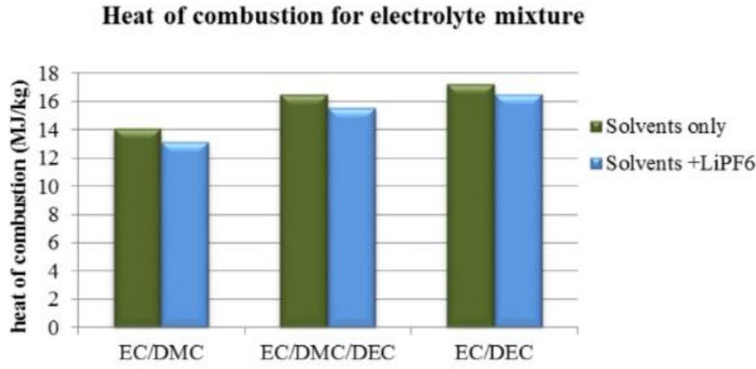
Figure 20. Heat of combustion for different electrolyte mixtures
