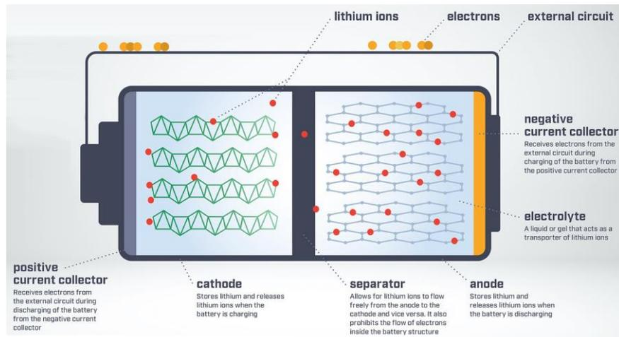
Figure 10. Main components of a Lithium-ion battery
