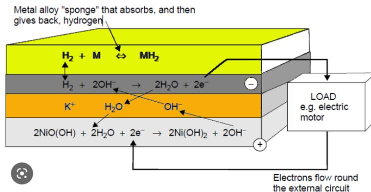
Figure 7. Design of a nickel-metal hydride battery
