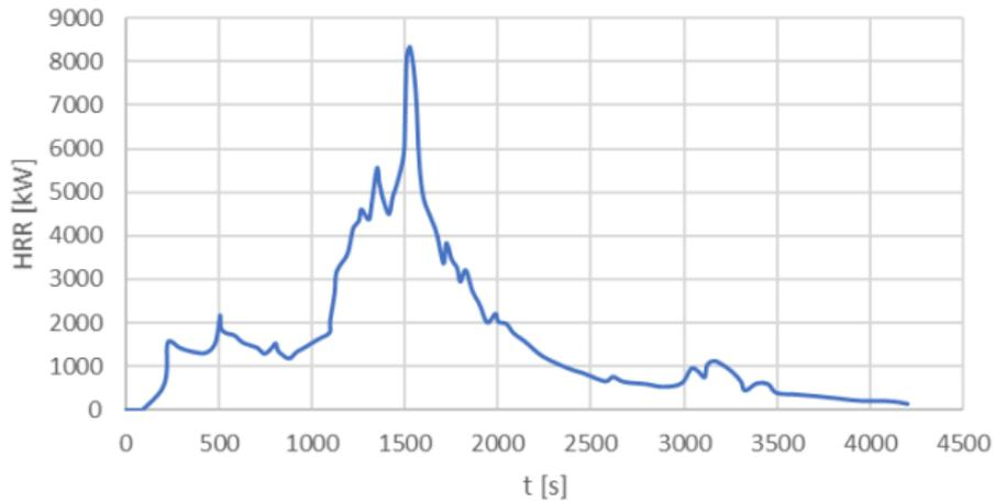
Figure 24. General curve of an internal combustion engine vehicle (ICEV)
