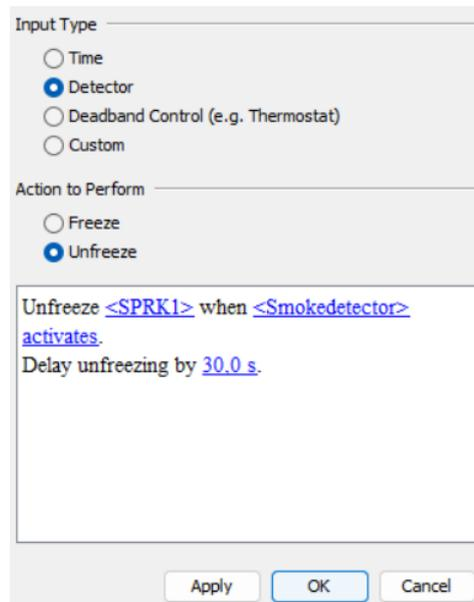
Figure 46. Control system for sprinkler activation
