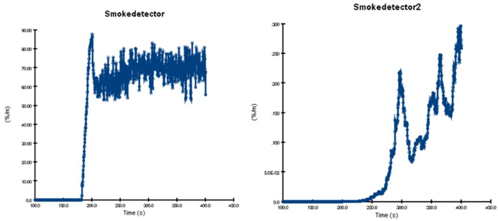
Figure 83. Smoke detectors results (EV case)
