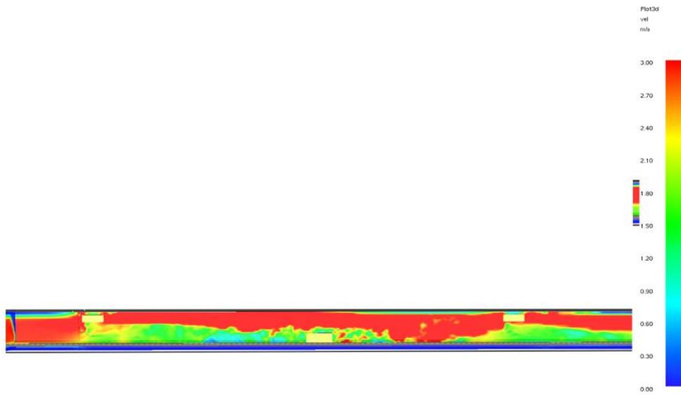
Figure 77. Gas velocity in the tunnel after 100 seconds
