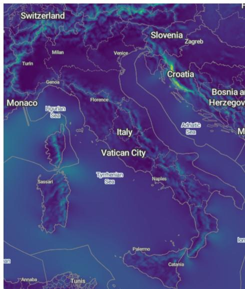
**Figure 2.8:** Italy mesoscale modelling of Wind Power Density at 100 m.
