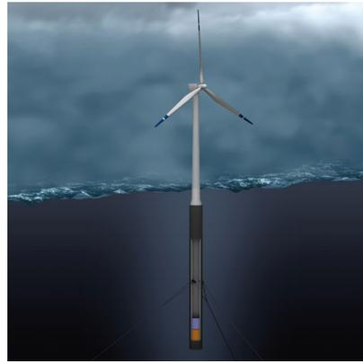
**Figure 3.9:** Hywind spar-buoy concept.
