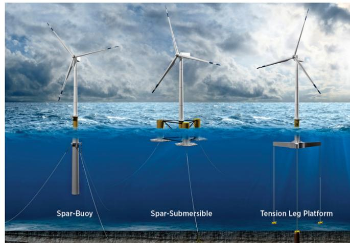
**Figure 3.8:** Main foundations for floating offshore wind [39].
