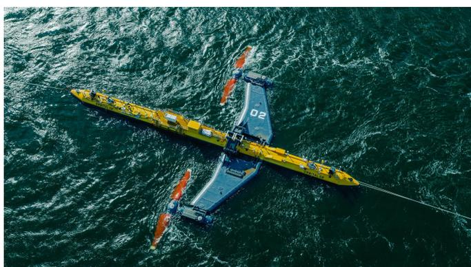
**Figure 3.17:** Picture of Orbital O2, the most powerful tidal turbine in the world.[49]
