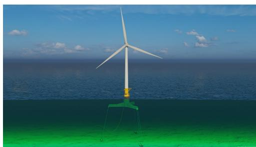
Figure 3.11: Bluewater TLP conceptual design.
