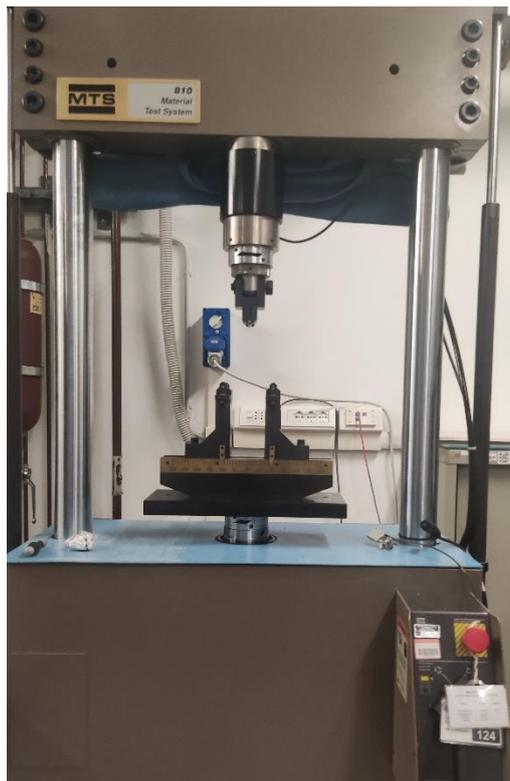
Figura 45 Pressa servo-idraulica MTS 810.
