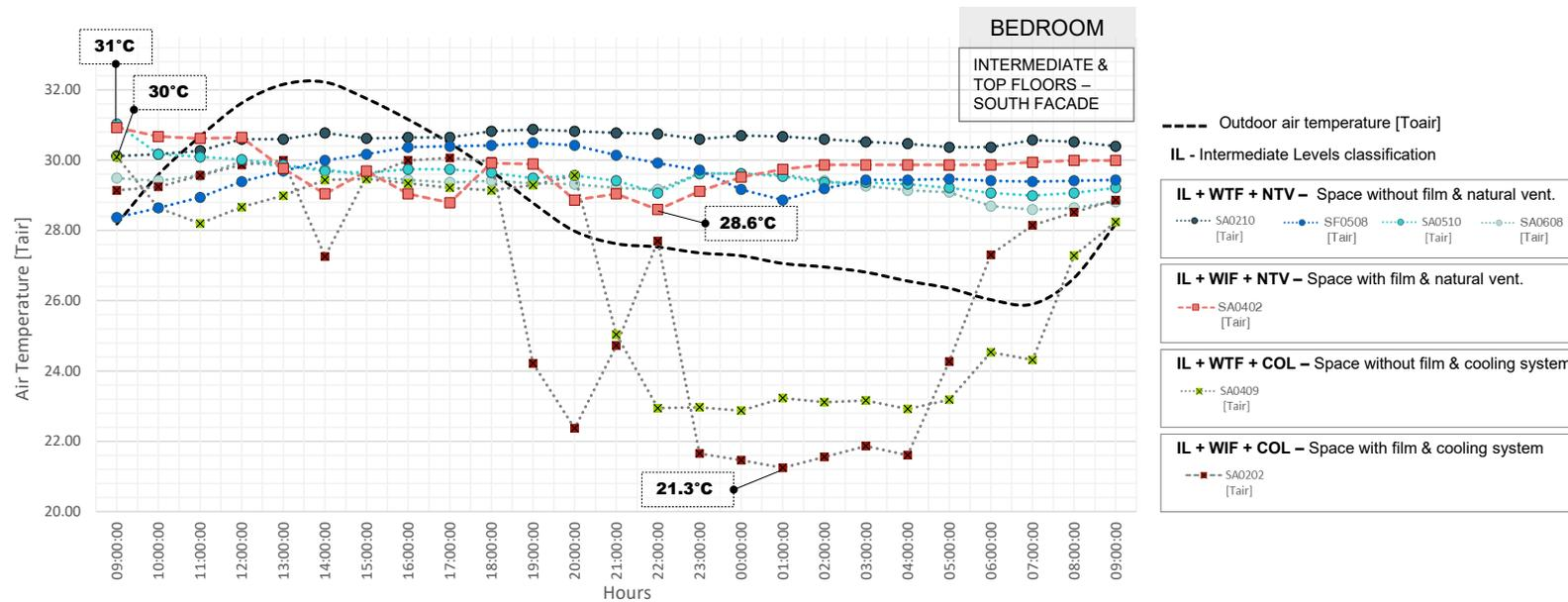
Figure 21. Bedrooms air temperature [ $T_{air}$ ] in intermediate & Top floors at south façade. The outdoor air temperature daily average was taken from IDEAM climate data. Source: developed by the author with indoor thermal comfort survey data.
