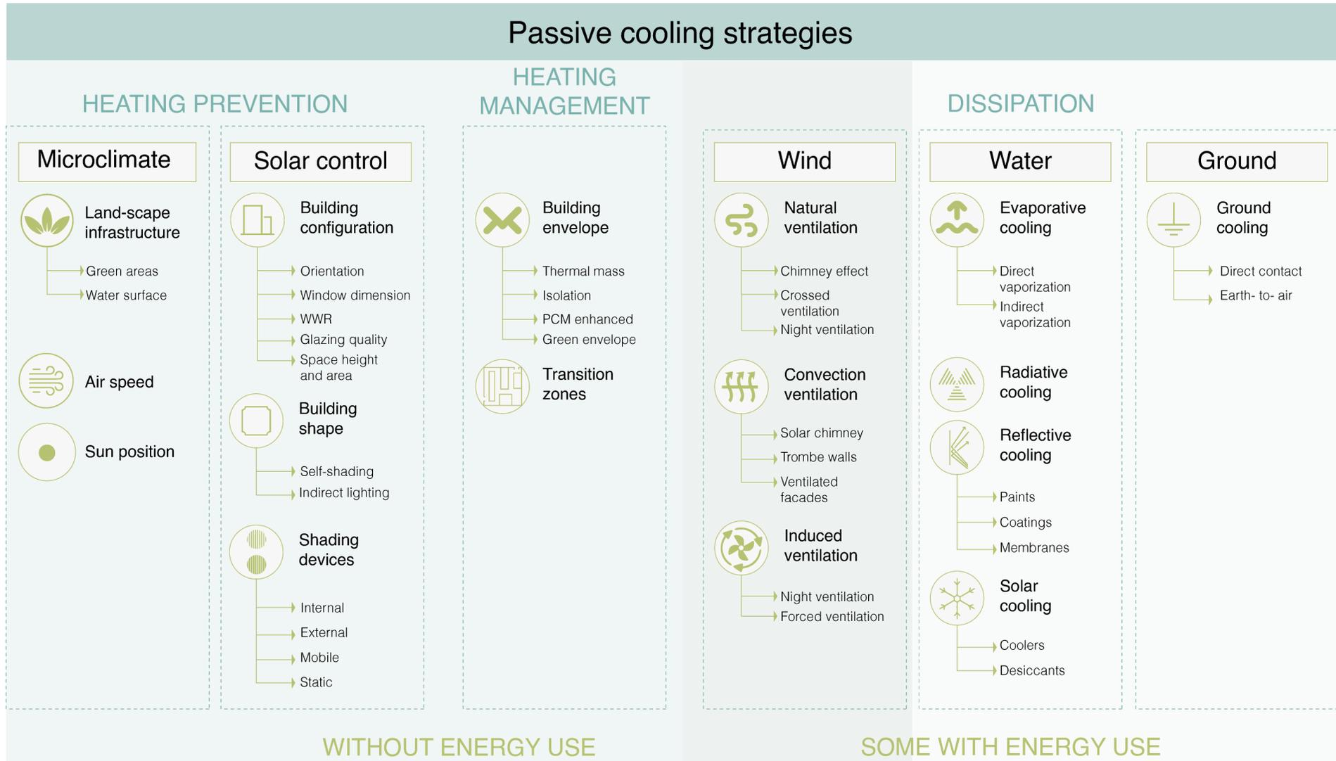
Figure 18. Passive cooling strategies. Source: Compilation based on (Giraldo, 2018), (Geetha & Velraj, 2012), (Hernández Sánchez, 2018), (Varas Vega, 2020), (Architecture 2030, n.d.),
