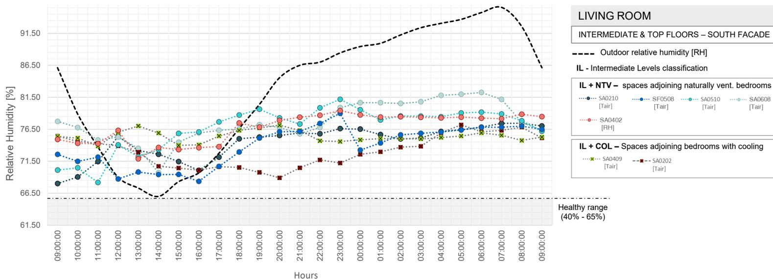
Figure 23. Living rooms relative humidity [RH]. The outdoor RH is from IDEAM climate data. Source: developed by the author with indoor thermal comfort survey data.
