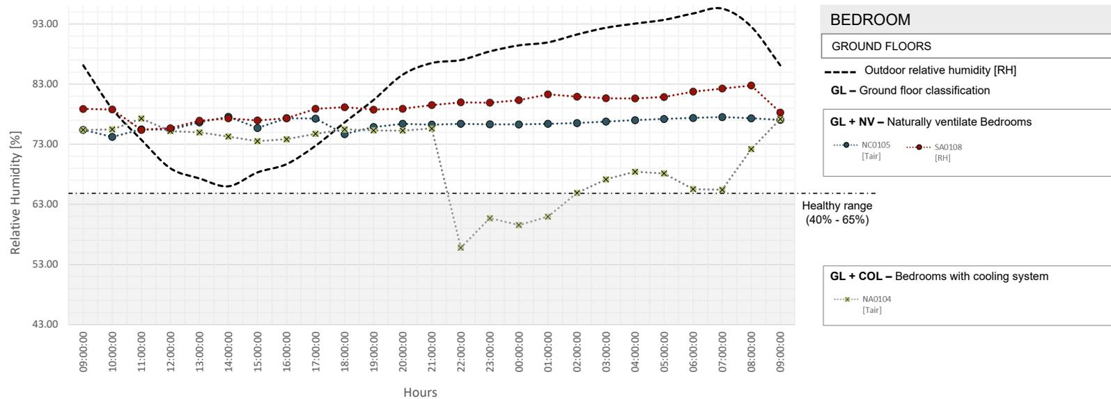
Figure 28. Bedrooms relative humidity [RH] on the ground floor. The outdoor RH is from IDEAM climate data. Source: developed by the author with indoor thermal comfort survey data.
