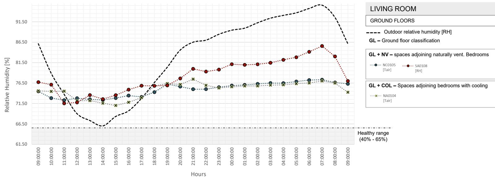
Figure 24. The outdoor RH is from IDEAM climate data. (1) Above: Living rooms relative humidity [RH] in intermediate & Top floors at north façade. (2) Below: Living rooms relative humidity [RH] on the ground floor. Source: developed by the author with indoor thermal comfort survey data.
