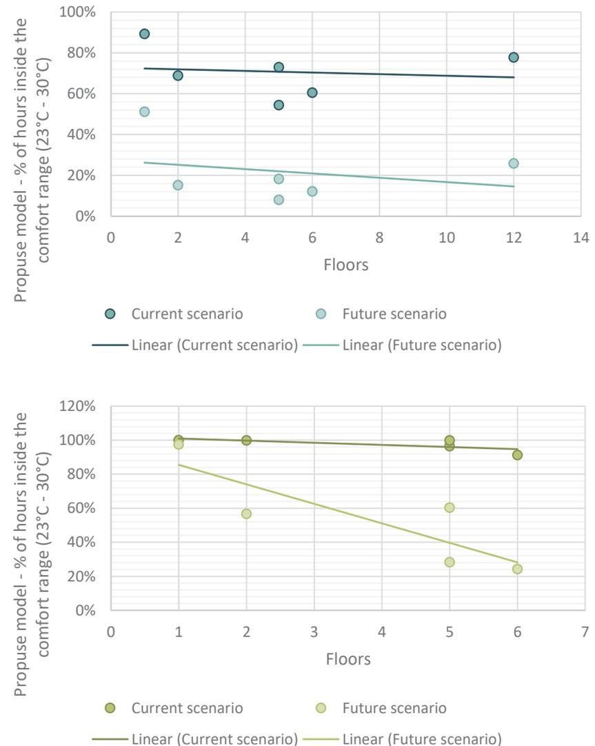
Figure 30. (1) Above proposed model living room % of hours inside the comfort range in current and future scenario. (2) below proposed model bedroom % of hours inside the comfort range in current and future scenario. Source: Author's elaboration.
