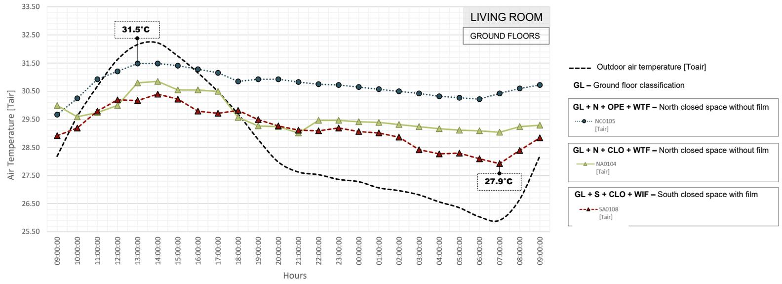
Figure 20. The outdoor air temperature daily average was taken from IDEAM climate data. (1) Above: Living rooms air temperature [Tair] in intermediate & Top floors at north façade. (2) Below: Living rooms air temperature [Tair] on the ground floor. Source: developed by the author with indoor thermal comfort survey data.
