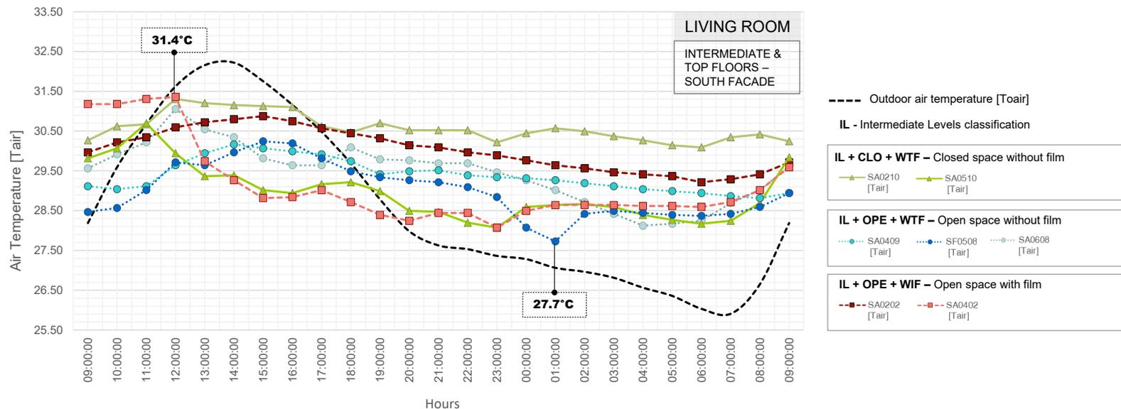
Figure 19. Living rooms air temperature [Tair] in intermediate & Top floors at south façade. The outdoor air temperature daily average was taken from IDEAM climate data. Source: developed by the author with indoor thermal comfort survey data.
