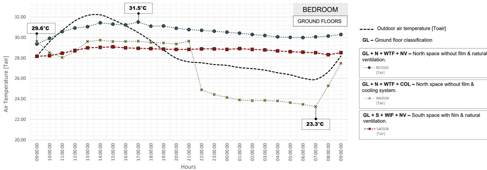
Figure 22. The outdoor air temperature daily average was taken from IDEAM climate data. (1) Above: Bedrooms air temperature [Tair] in intermediate & Top floors at north façade. (2) Below: Bedrooms air temperature [Tair] on the ground floor. Source: developed by the author with indoor thermal comfort survey data
