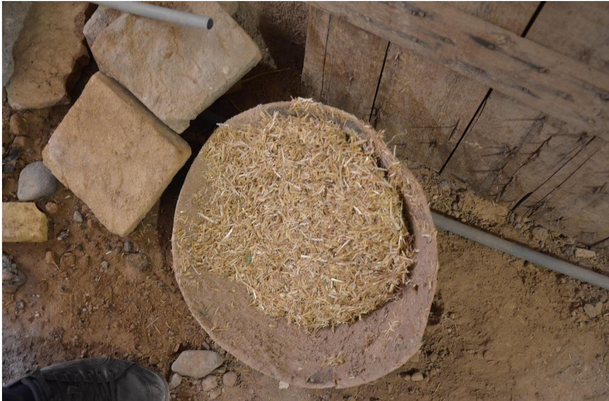
Figure 3-81: tiny particles of straw which use in mud walls. (Photo by Arsalan Chabok)
