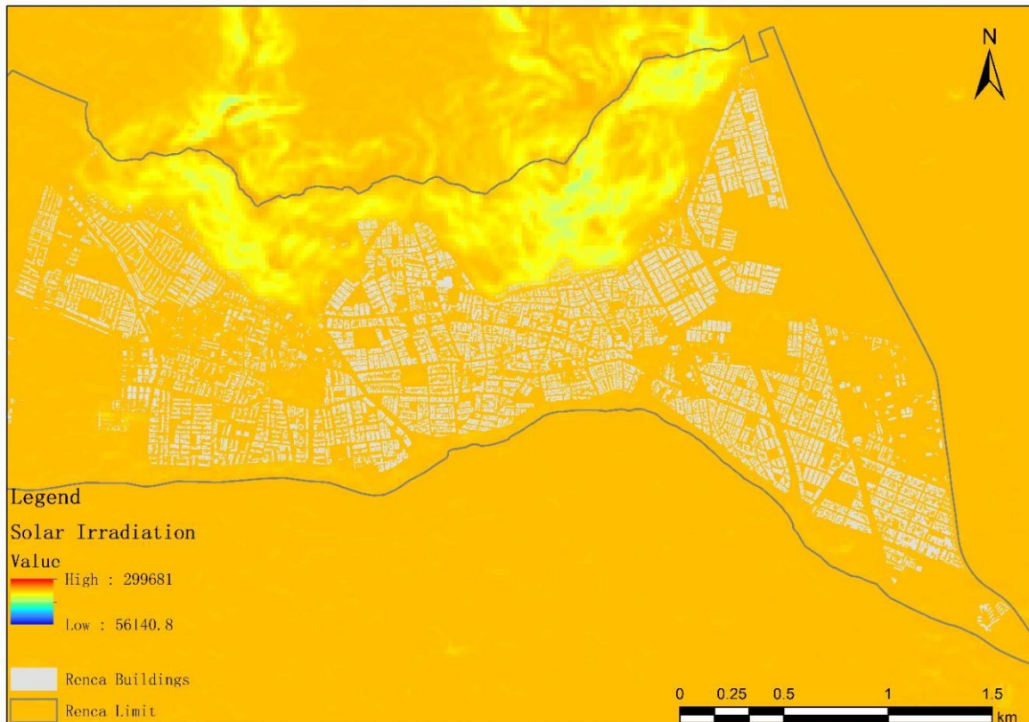
Figure 13: Annual Solar irradiation simulation of the municipality Renca (DEM in 2011 with the accuracy 30m × 30m)
