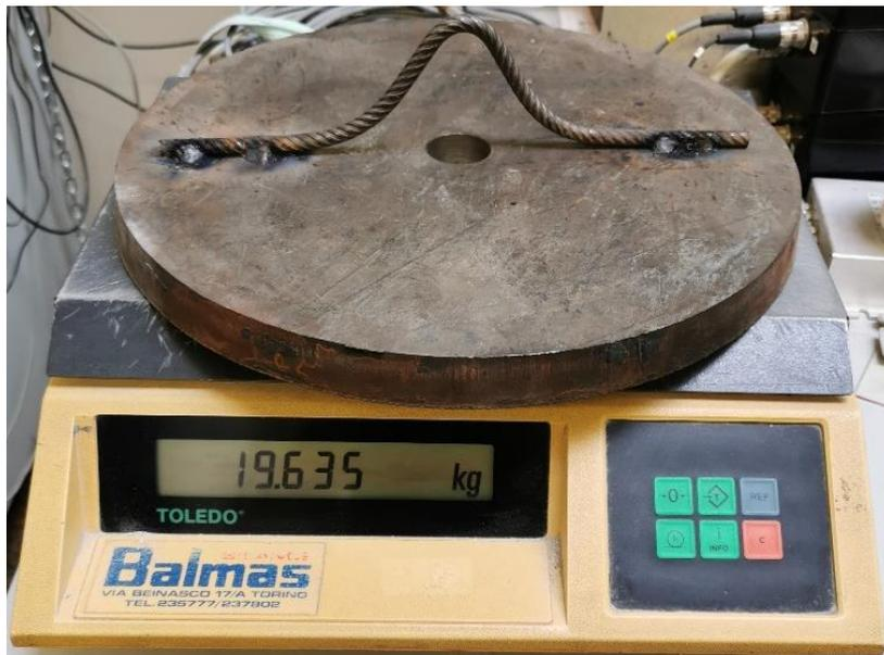
Figure 4.9 Compaction hammer overall weight
