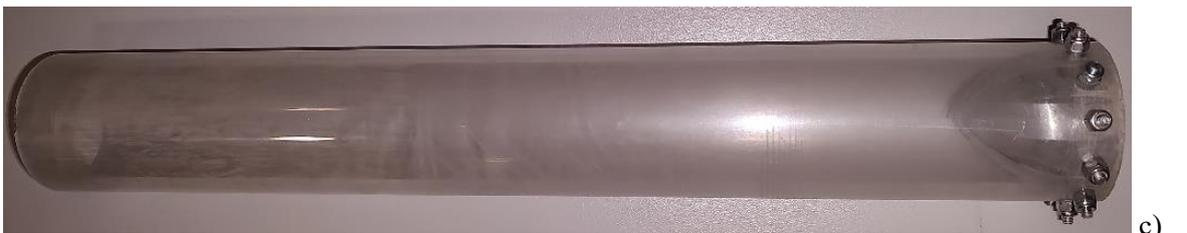
Figure 4.21 "PMMA" catcher equipped on the holder: a) bottom view, b) lateral view, c) top view
