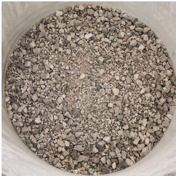
*Figure 4.5 Test soil: uniform gravel*
