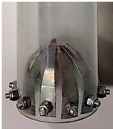
Figure 3.14 DIANA's harmonic steel catcher prototype
