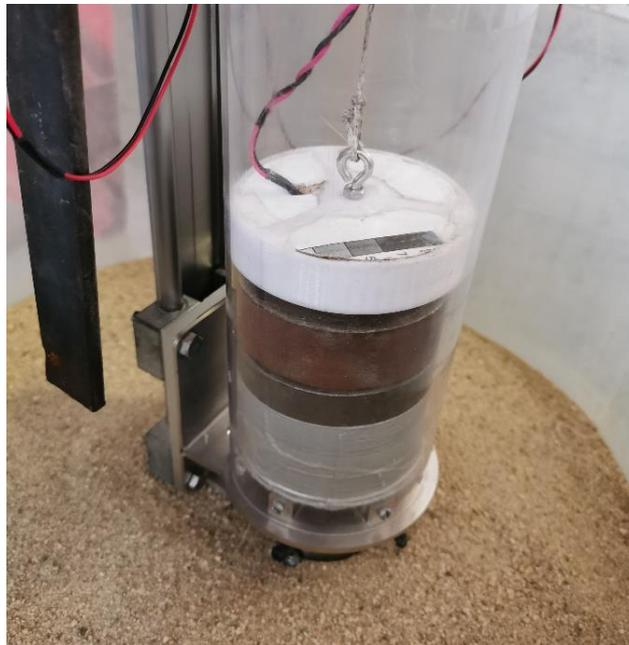
*Figure 4.36 End of sampling test with sampler prototype on loose uniform sand*
