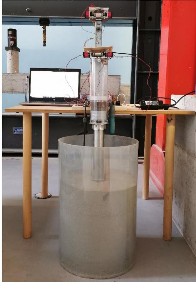
*Figure 4.35 Beginning of sampling test with sampler prototype on loose uniform sand*
