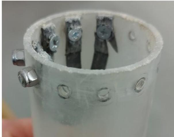
*Figure 4.29 PLA 1 mm catcher failure during assembly*
