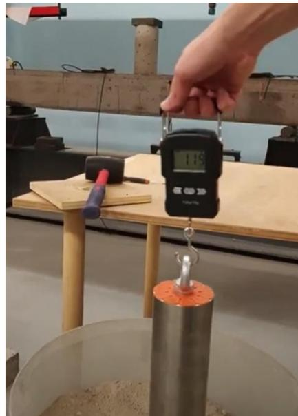
Figure 3.7 Test: measure of extraction weight from Mars regolith
