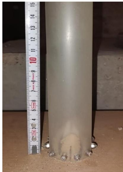
Figure 4.33 Recovered soil after test with uniform sand
