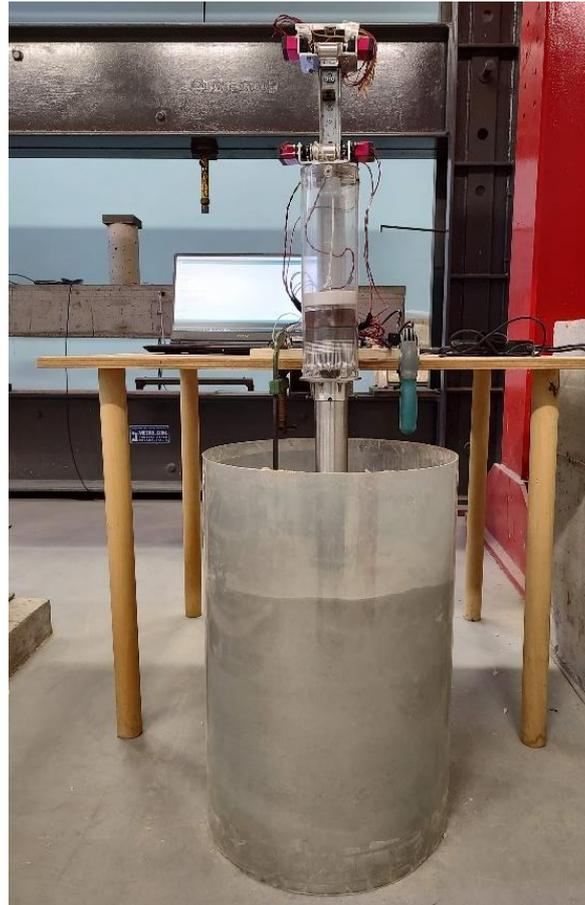
*Figure 4.38 Beginning of sampling test with sampler prototype on Mars regolith simulant*
