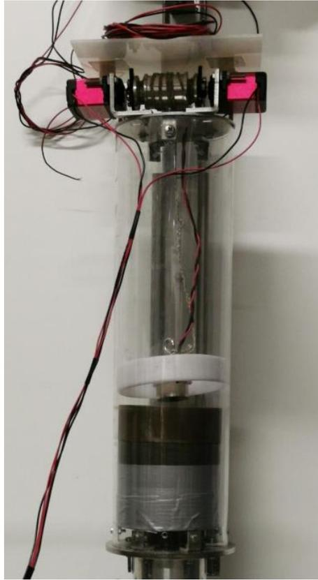
*Figure 3.27 DIANA's sampler: detail of the percussion system*
