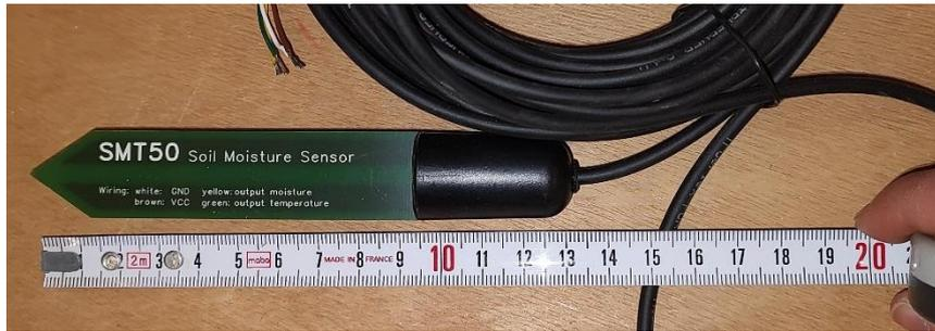
Figure 3.17 Humidity and temperature soil sensor to be positioned inside the holder
