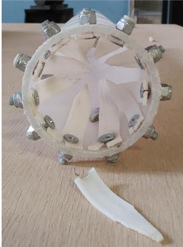
*Figure 4.30 PLA 0.5 mm catcher failure after tests with uniform gravel*
