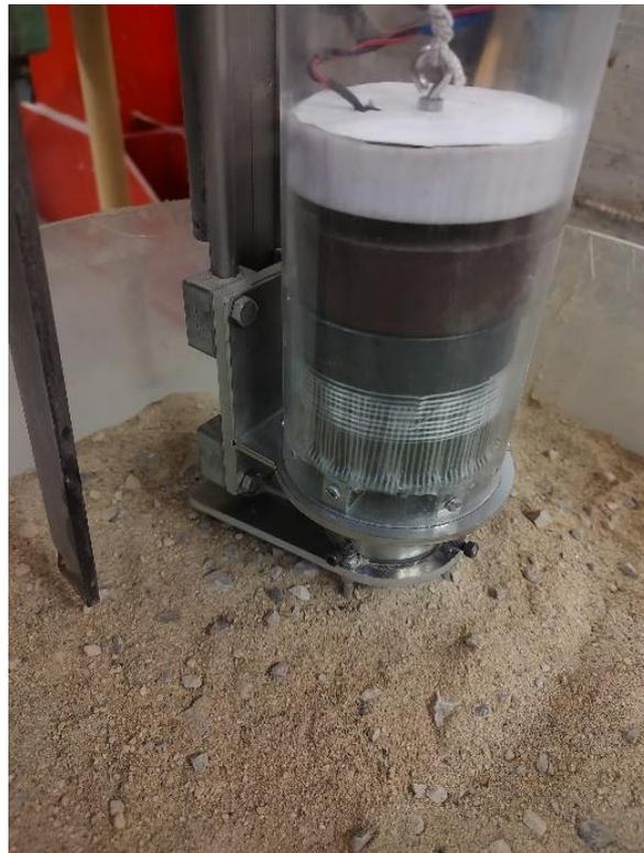
*Figure 4.39 End of sampling test with sampler prototype on Mars regolith simulant*
