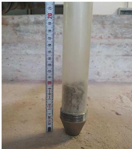
Figure 4.43 Holder with sampled material of compacted Mars regolith simulant
