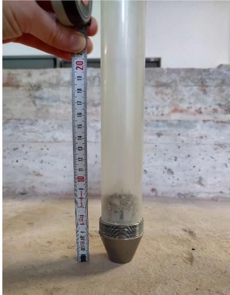
Figure 4.40 Holder with sampled material of Mars regolith simulant
