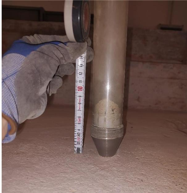
Figure 4.42 Holder with sampled material of compacted uniform sand
