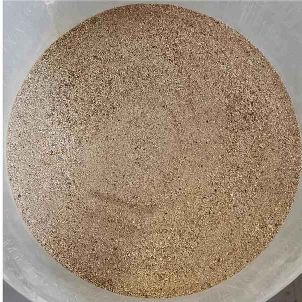
*Figure 4.4 Test soil: uniform sand*
