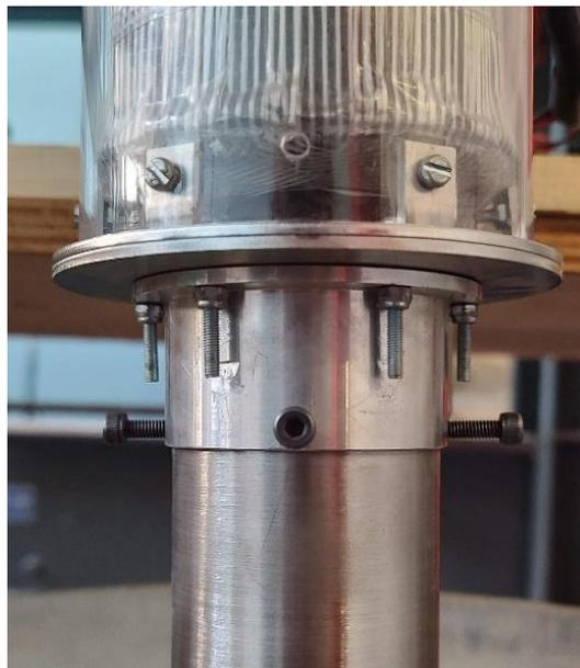
*Figure 3.28 DIANA sampler: detail of the aluminium connection between sampler and percussion system*
