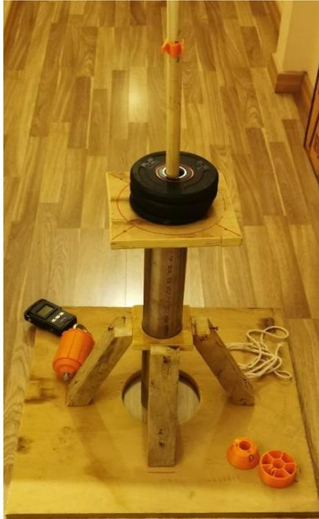
Figure 3.22 DIANA's test equipment for evaluation of weight and dropping height
