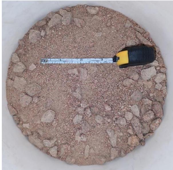
Figure 2.5 Sample of Mars soil simulant from Thales Alenia Space
