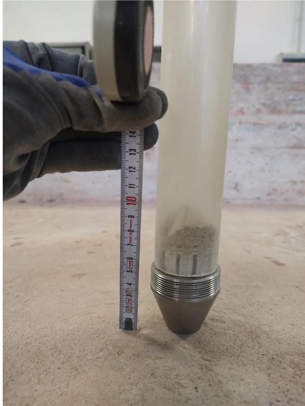
*Figure 4.37 Holder with sampled material of loose uniform sand*
