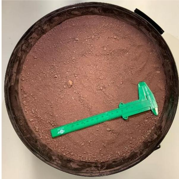
Figure 2.3 Sample of Mars soil simulant from ALTEC S.p.A.
