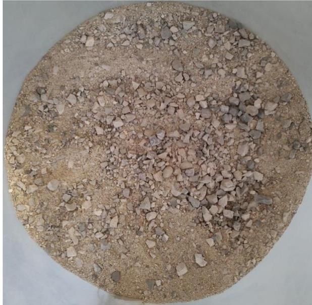
Figure 4.8 Test soil: 50% sand - 50% gravel
