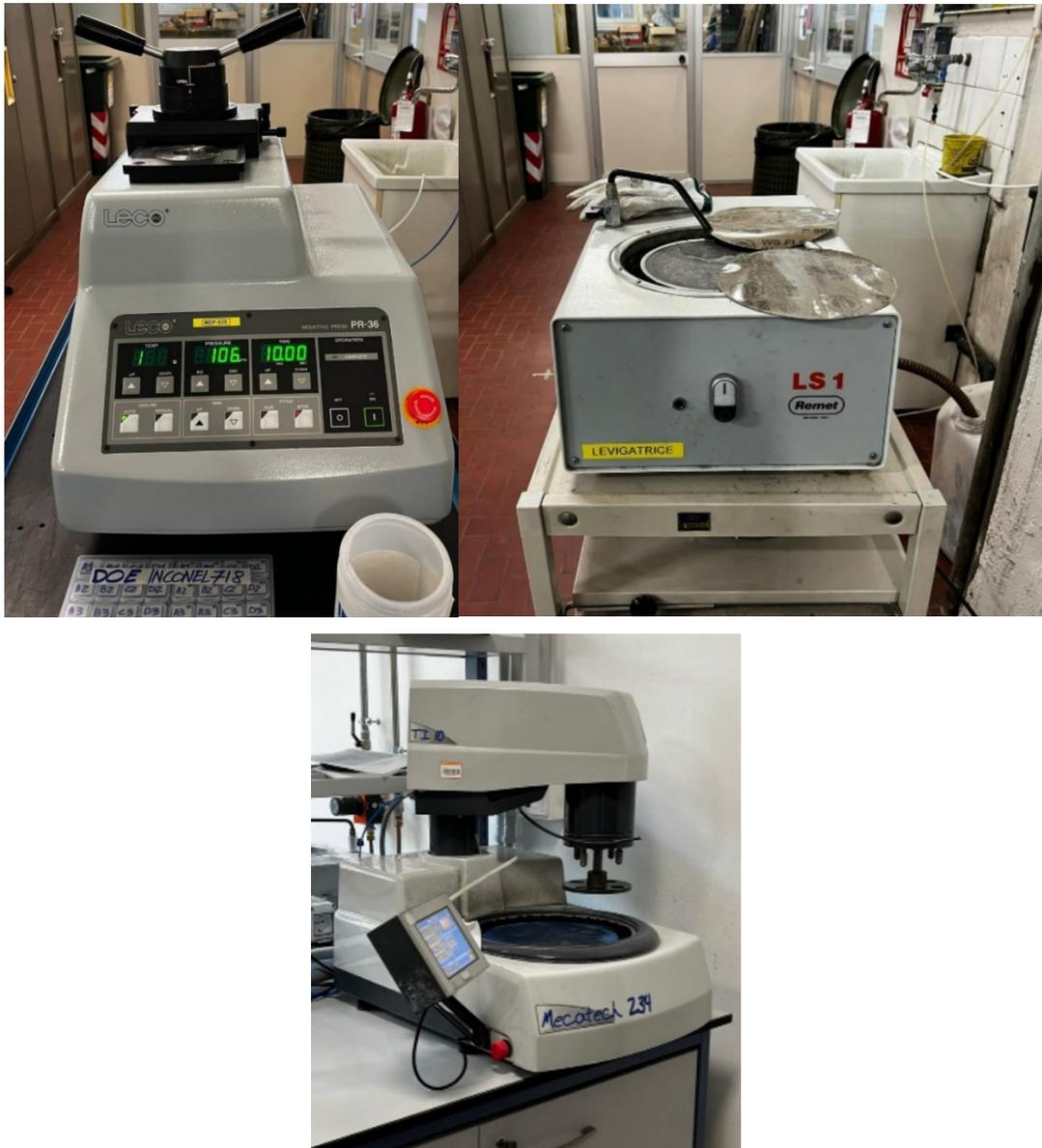
Figure 4-3: Metallographic preparation machines (a) specimen mold machine (b) polishing machine (DIMEAS) (c) Polishing machine (DISAT)
