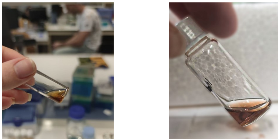
Figure 44 3 % CHP407- SHF68 solution containing PheLig NPs at time 0 (left) and after 1 day (right). No gelation was observed even if the turbidity of the solution changed with time.
