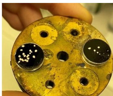
**Figure 12:** Sarcospheres mounted on carbon discs for SEM analysis.
