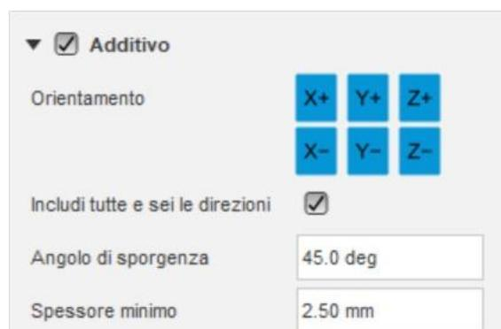
FIG. 62 - MODULO "ADDITIVO" PER LEGHE DI ALLUMINIO
