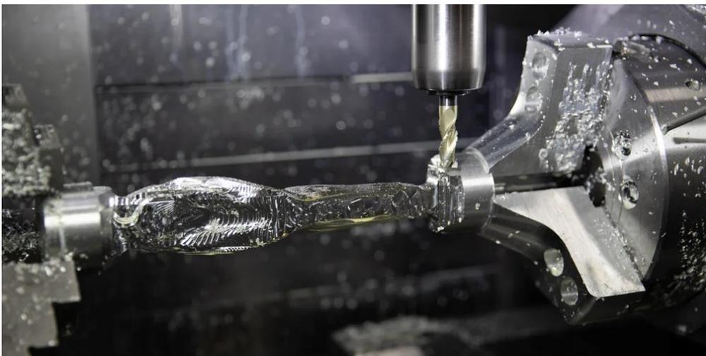
**FIG. 4 - PEDIVELLA REALIZZATA CON MACCHINA UTENSILE 5 ASSI [4]**
