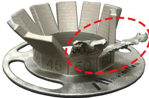
FIG. 18 - COLLASSO DI SUPERFICI A SBALZO INCLINATE [21]
