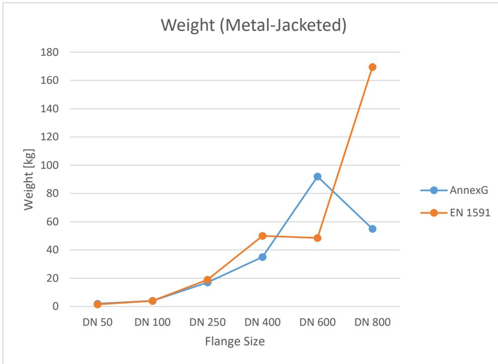
Figure 10. Comparison of weight in EN 1591 and Annex G Metal-Jacketed
