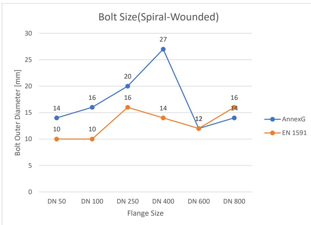
Figure 5. Comparison of bolt size in EN 1591 and Annex G Spiral Wounded
