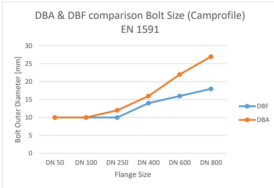
Figure 28. Comparison of Bolt Size for Camprofile gasket designed by DBA and DBF EN 1591
