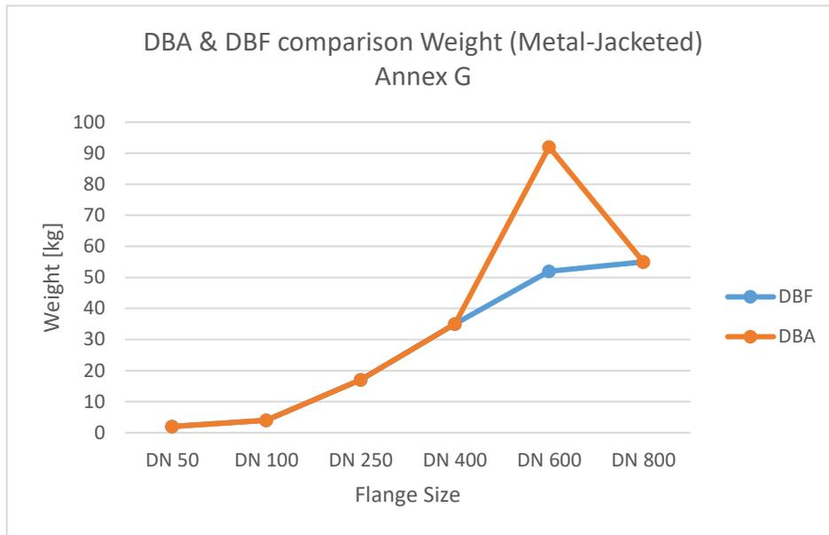
Figure 35. Comparison of weight for Metal Jacketed gasket designed by DBA and DBF
