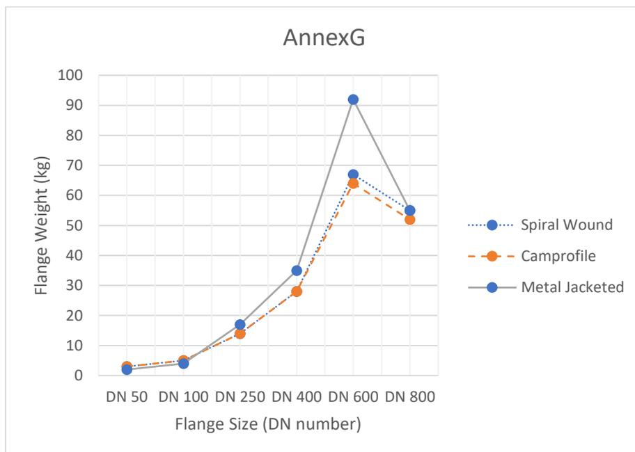
Figure 3. Comparison of flange weight in Annex G
