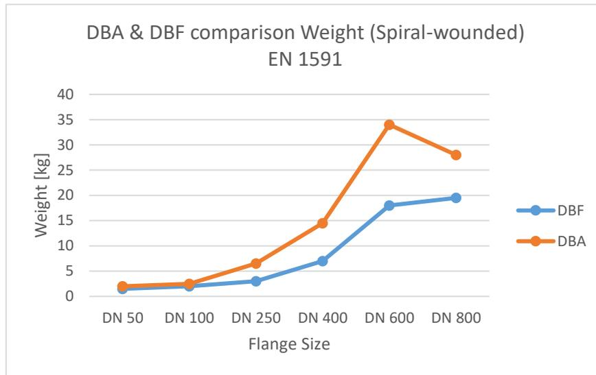
Figure 32. Comparison of weight for Spiral wounded gasket designed by DBA and DBF
