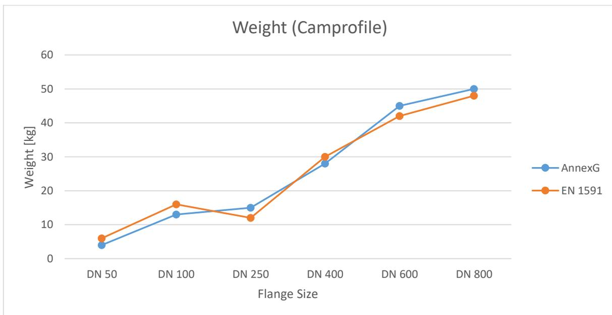
Figure 22. Comparison of weight of Camprofile gasket, designed by Annex G and EN 1591
