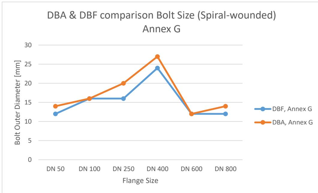
Figure 25. Comparison of Bolt Size for Spiral-wounded gasket designed by DBA and DBF Annex G
