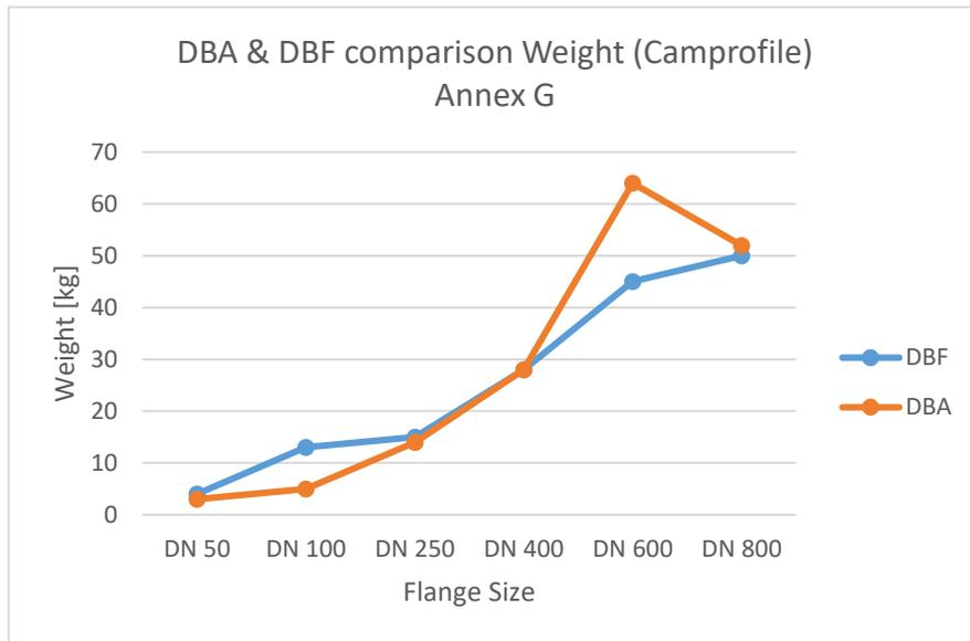
Figure 33. Comparison of weight for Camprofile gasket designed by DBA and DBF
