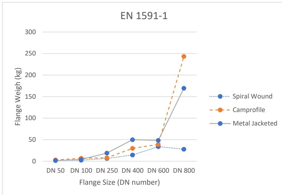
Figure 4. Comparison of flange weight in EN 1591
