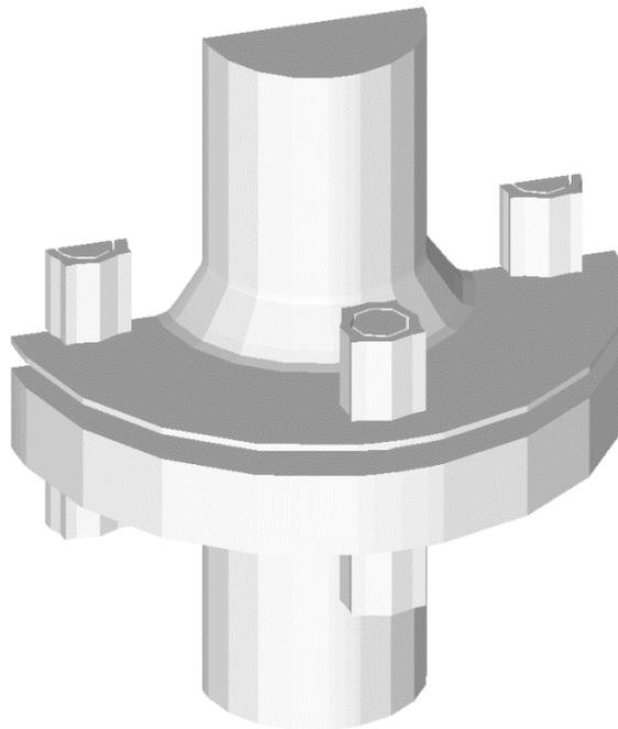
Figure 11. Schematic model of DN 50 Flange in AxiPro
