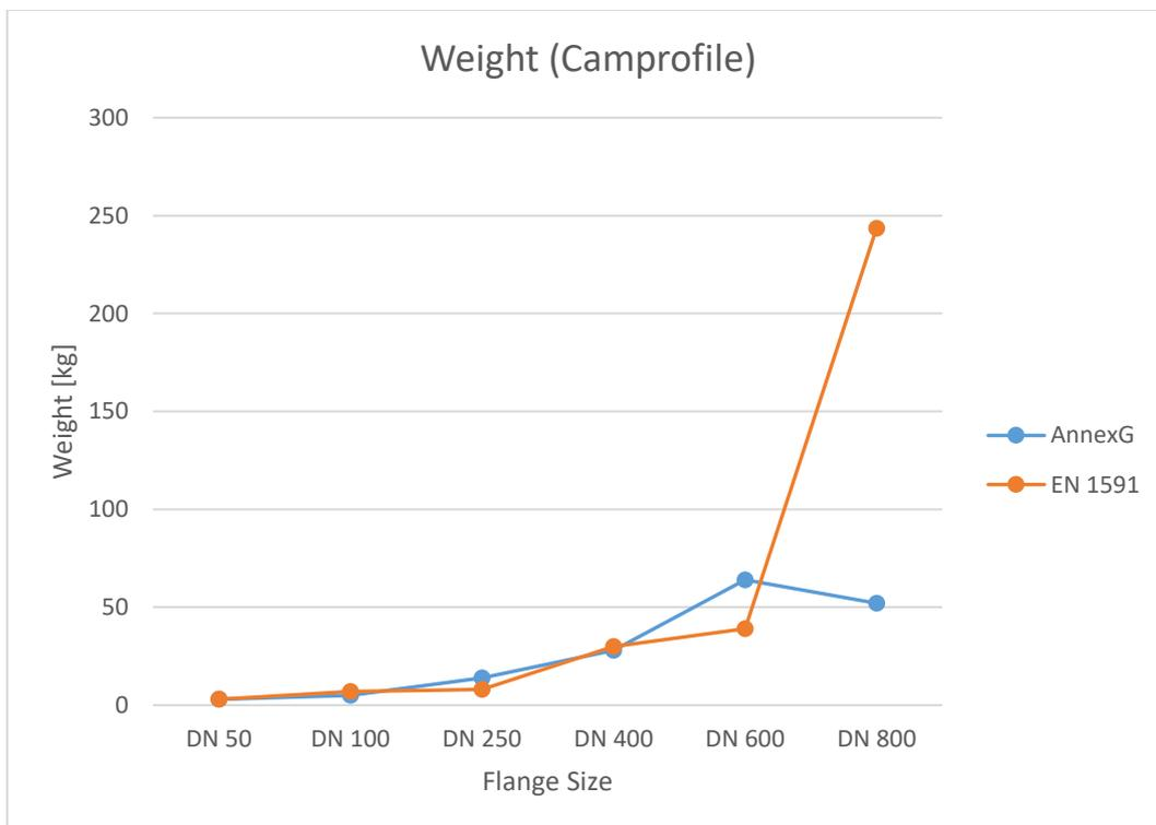
Figure 9. Comparison of weight in EN 1591 and Annex G Kamprofile
