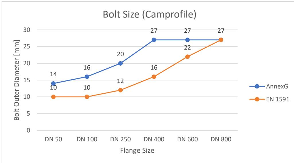
Figure 6. Comparison of bolt size in EN 1591 and Annex G Kamprofile
