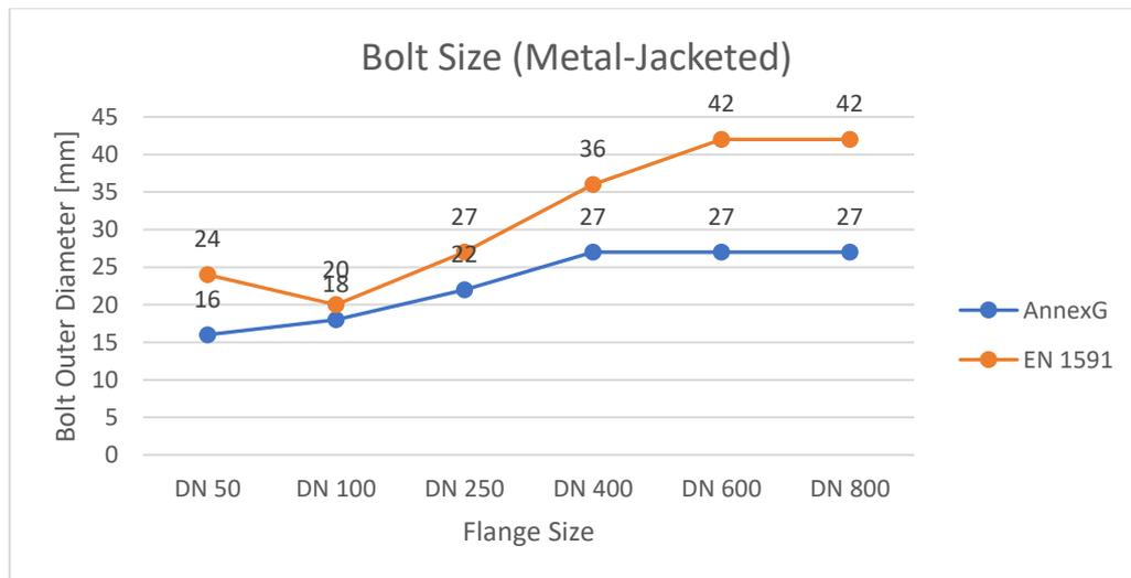
Figure 7. Comparison of bolt size in EN 1591 and Annex G Metal-Jacketed
