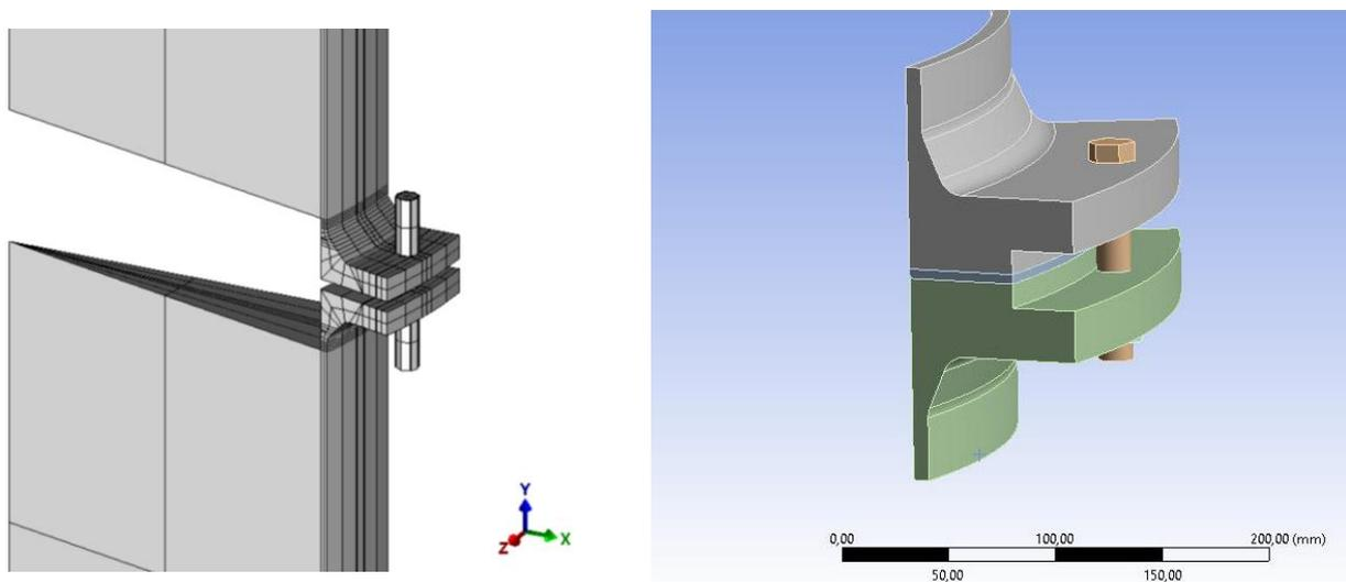
Figure 15. Schematic of Flange in: Right: Ansys left: AxiPro
