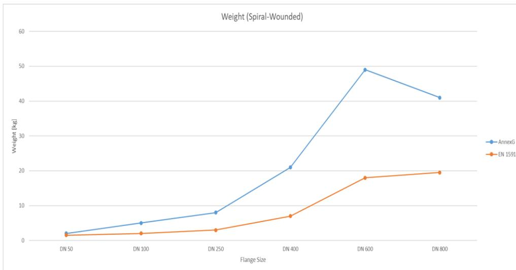
Figure 20. Comparison of weight of Spiral Wounded gasket, designed by Annex G and EN 1591
