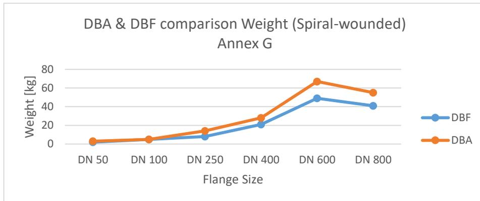
Figure 31. Comparison of weight for Spiral wounded gasket designed by DBA and DBF
