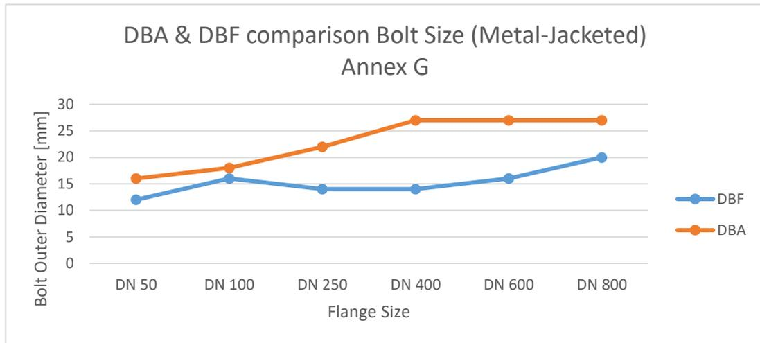
Figure 29. Comparison of Bolt Size for Metal Jacketed gasket designed by DBA and DBF
