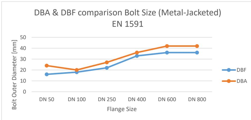
Figure 30. Comparison of Bolt Size for Metal Jacketed gasket designed by DBA and DBF
