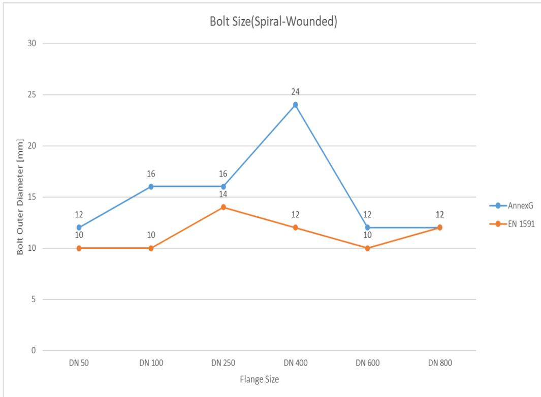
Figure 19. Comparison of bolt size of Spiral Wounded gasket, designed by Annex G and EN 1591
