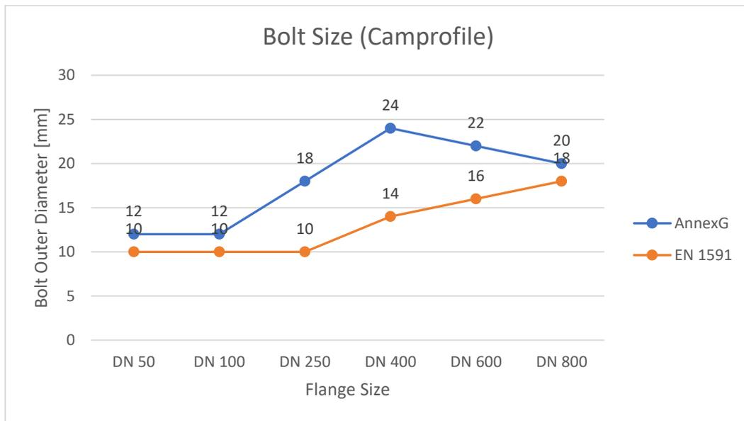
Figure 21. Comparison of bolt size of Camprofile gasket, designed by Annex G and EN 1591
