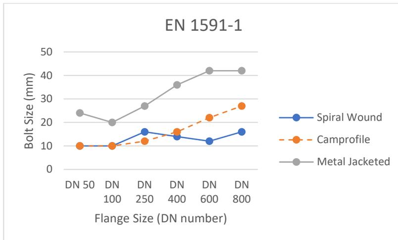
Figure 2. Comparison of bolt size in EN 1591
