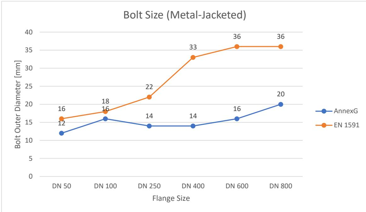
Figure 23. Comparison of bolt size of Metal jacketed gasket, designed by Annex G and EN 1591
