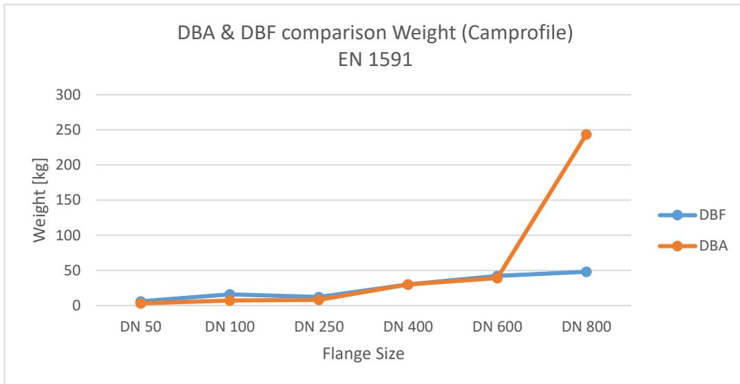
Figure 34. Comparison of weight for Camprofile gasket designed by DBA and DBF
