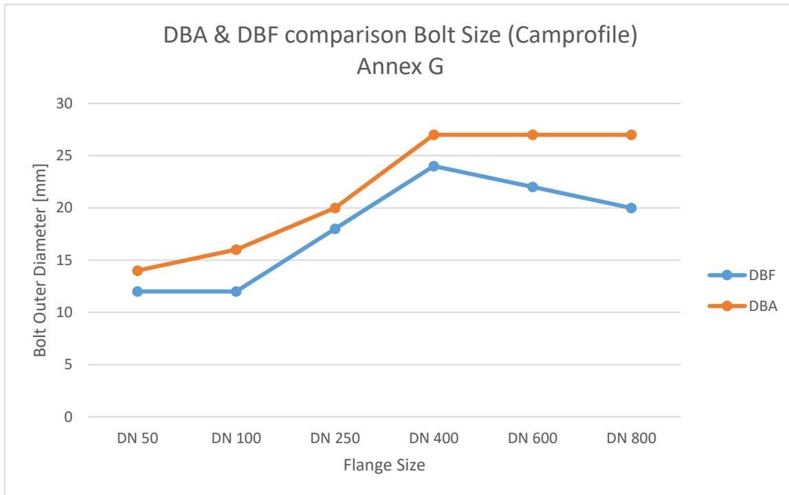
Figure 27. Comparison of Bolt Size for Camprofile gasket designed by DBA and DBF Annex G
