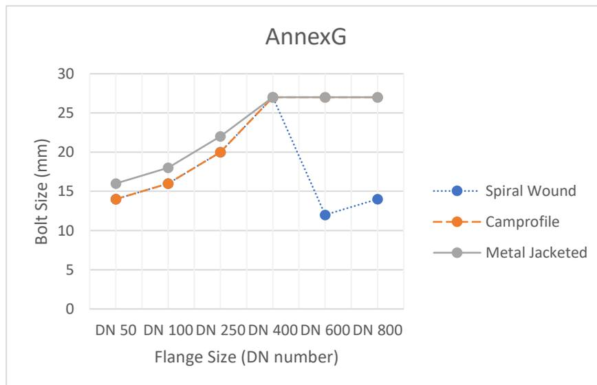
Figure 1. Comparison of bolt size in Annex G
