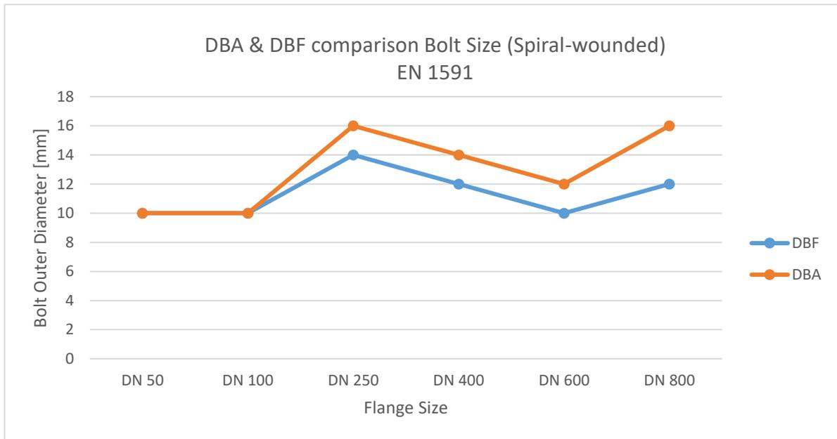
Figure 26. Comparison of Bolt Size for Spiral-wounded gasket designed by DBA and DBF
