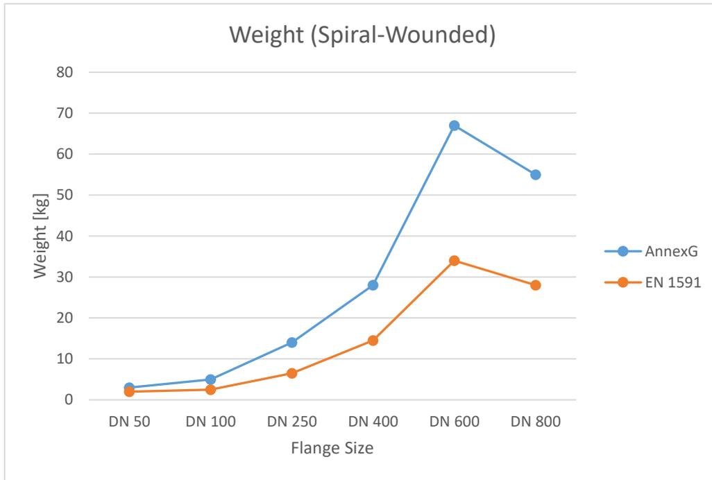
Figure 8. Comparison of weight in EN 1591 and Annex G Spiral Wounded
