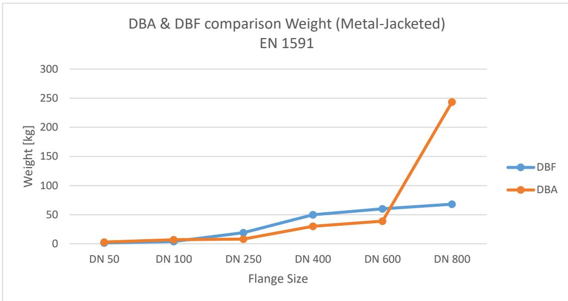
Figure 36. Comparison of weight for Metal Jacketed gasket designed by DBA and DBF
