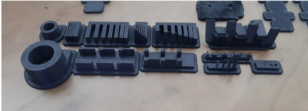
**Figure 3.17:** Carbon PEEK: specimens of the capability assessment
