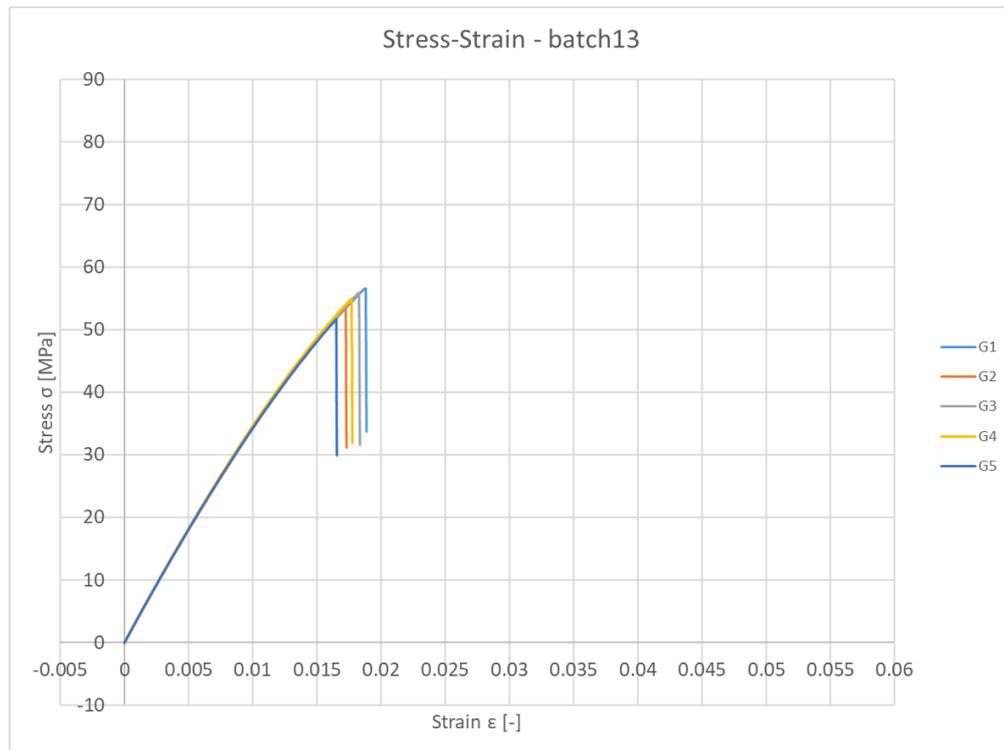
**Figure 4.17:** ULTEM™: stress vs strain diagrams
