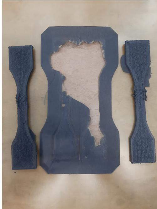
**Figure 4.9:** Carbon PEEK: broken buildsheet and ruined specimens after the artifacts' removal
