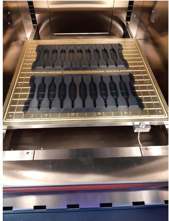
**Figure 4.11:** C-PEEK: four horizontal batches in the printer
