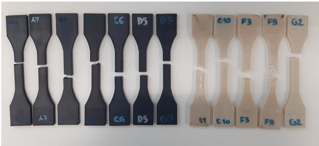
Figure 4.14: Selection of broken specimens
