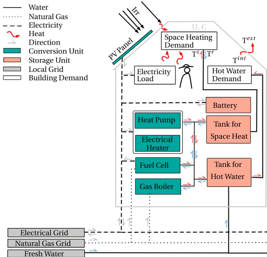
Figure 3.1: Schematic overview of a building energy system, which is also considered as a decentralized energy system [34]
