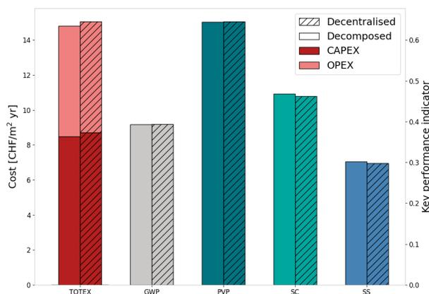
Figure 4.11: Comparison of centralized and decentralized design strategy
