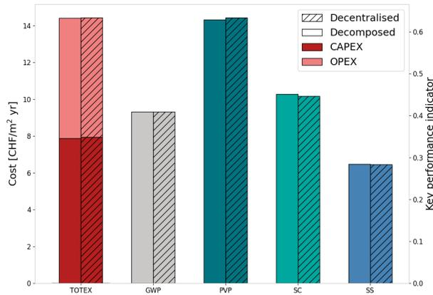
Figure 4.6: Comparison of centralized and decentralized design strategy
