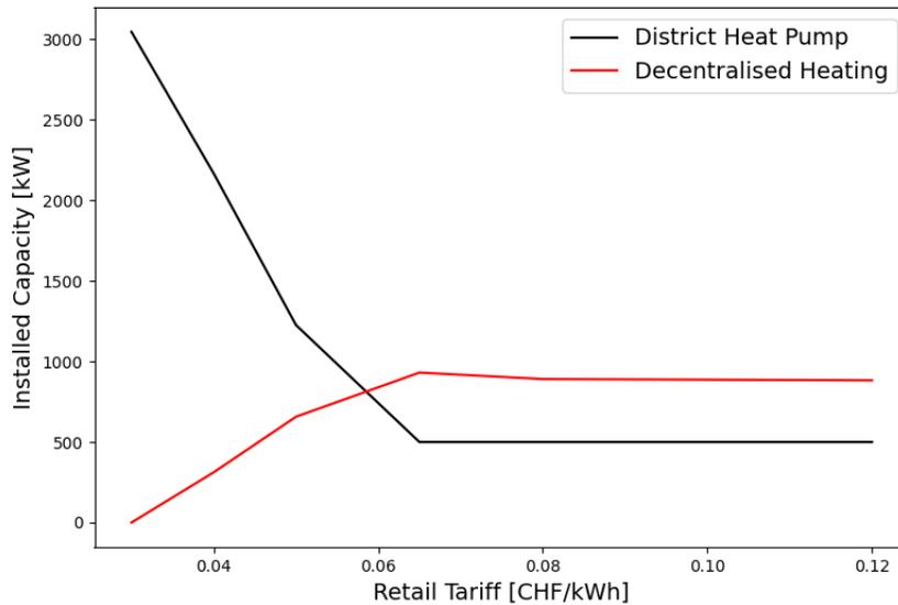
Figure 5.10: Installed capacity of district heat pump and decentralised heating production for increasing retail tariffs.
