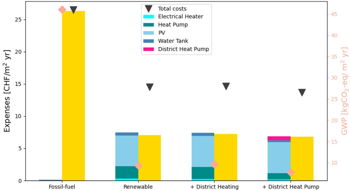
Figure 5.4: Scenario with different energy system configurations comparison
