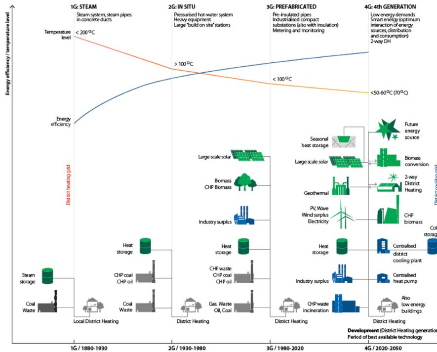
Figure 2.4: Illustration of the concept of 4<sup>th</sup> Generation District Heating in comparison to the previous three generations [31]
