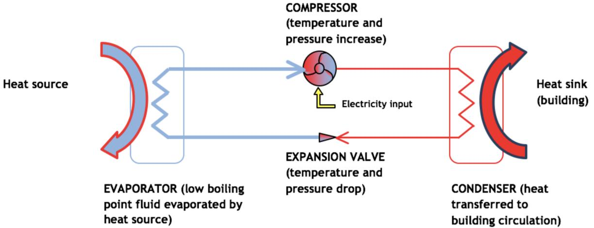
Figure 5.2: Heat pump cycle [44]
