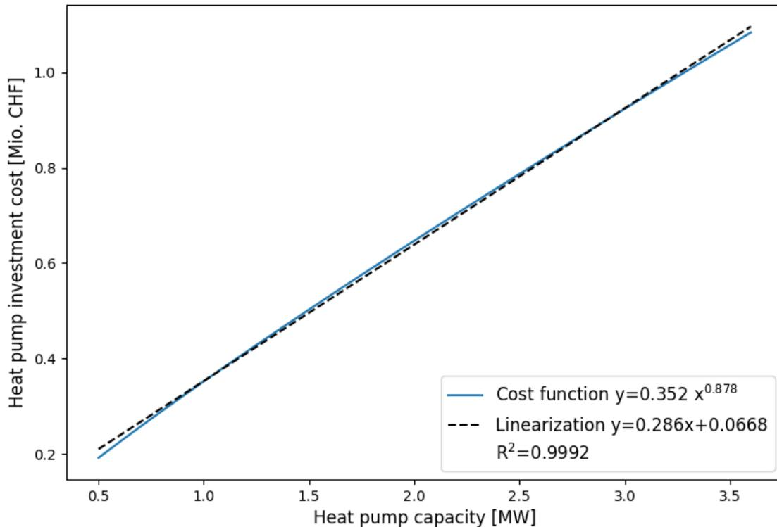
Figure 5.3: Heat pump cost function and linear regression line
