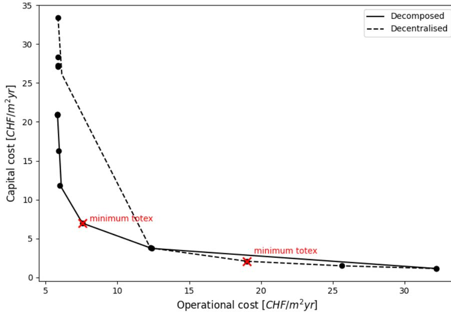
Figure 4.3: Comparison of the CAPEX–OPEX pareto curve resulting from the decentralized and centralized optimization strategies. Minimum total expenses (TOTEX) marked on both curves
