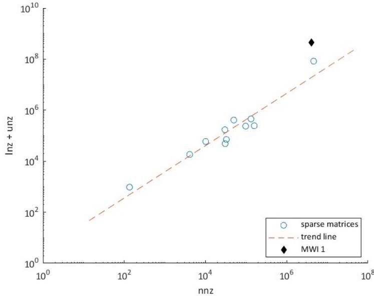
Figure 11 – Number of non-zeros before and after factorization
