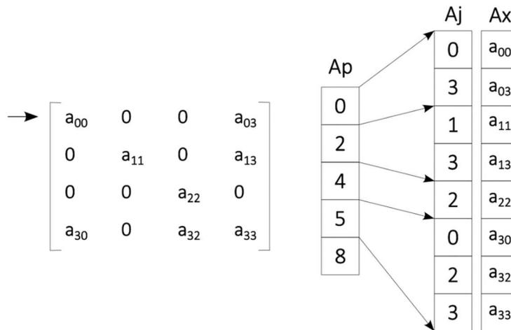
Figure 9 – Row-compressed storage example
