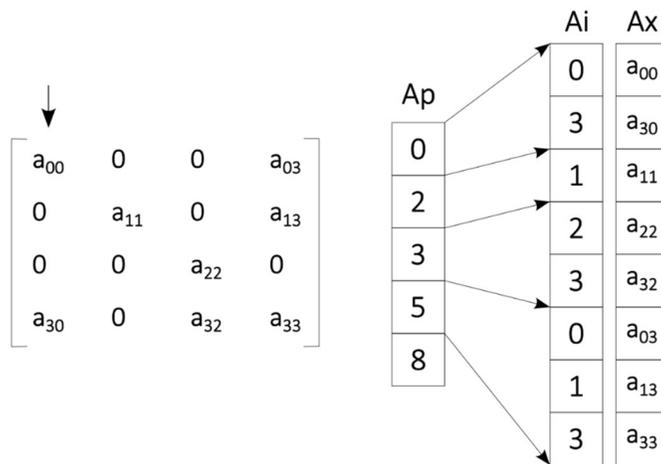
Figure 8 – Column-compressed storage example
