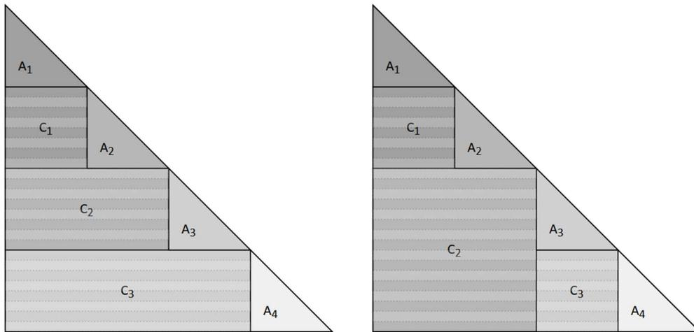
Figure 17 – Row Block and Recursive Block algorithms' graphical representation
