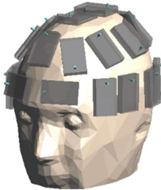
Figure 4 – Illustration of 3D discretization used in the CSI algorithm with the antennae.
