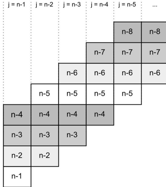
Figure 21 – Ring buffer behaviour for accumulator in Prototype 3
