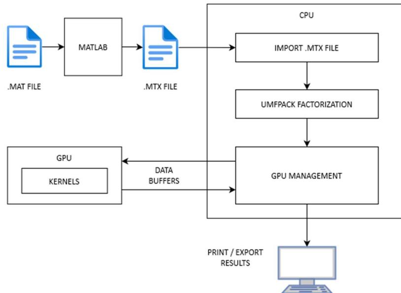
Figure 14 – Block diagram of the programs that use GPU
