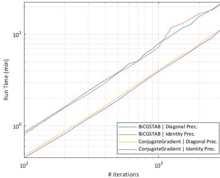
Figure 13 – Run time of iterative solvers
