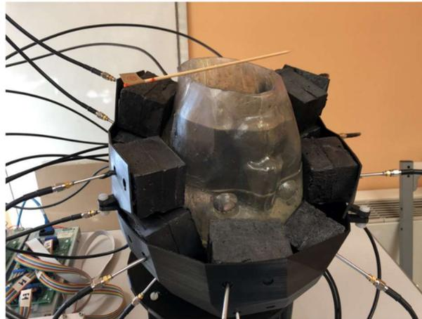
Figure 2 – Photography of the MWI system prototype. Image extracted from [3].
