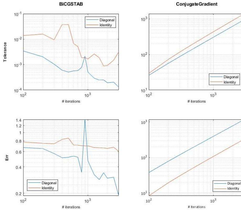
Figure 12 - Err and Tolerance evolution with number of iterations for BiCGSTAB and ConjugateGradient iterative solvers
