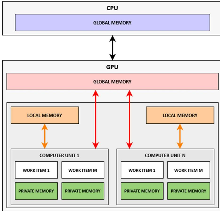
Figure 18 – OpenCL memory architecture
