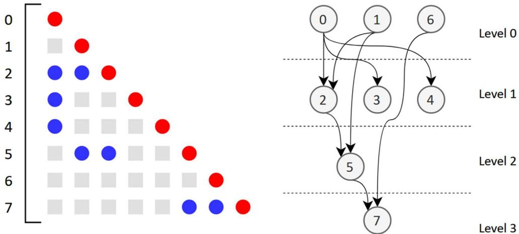
Figure 15 – Parallelization of a sparse matrix based on graphs. Non-zeros are represented by blue and red circles. Red circles for the diagonal elements and blue for non-diagonal elements.
