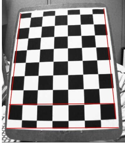
Figure 4.3: Example of Lens Distortion
