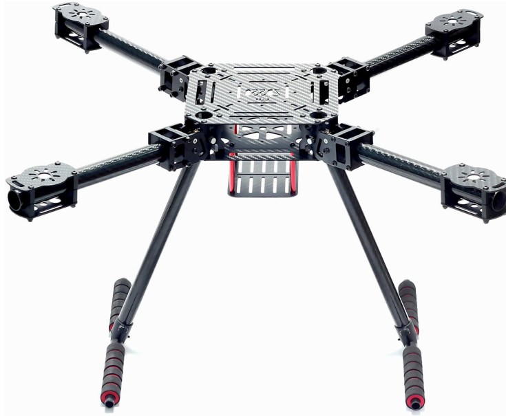
Figure 2.1: Readytosky ZD550 Frame 550mm Folding Carbon Fiber
