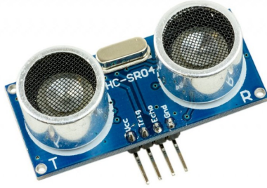
Figure 1.10: Ultrasonic Sensor HC SR-04
