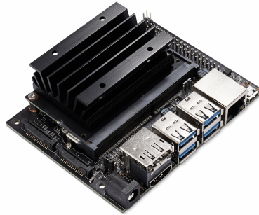
Figure 1.5: Nvidia Jetson Nano
