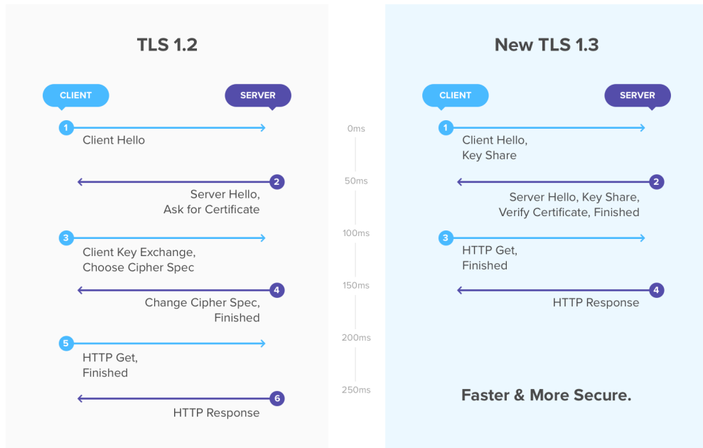
Figure 3.1. TLS handshake. On the left version 1.2 handshake. On the right the version 1.3 handshake (Source: [34]).
