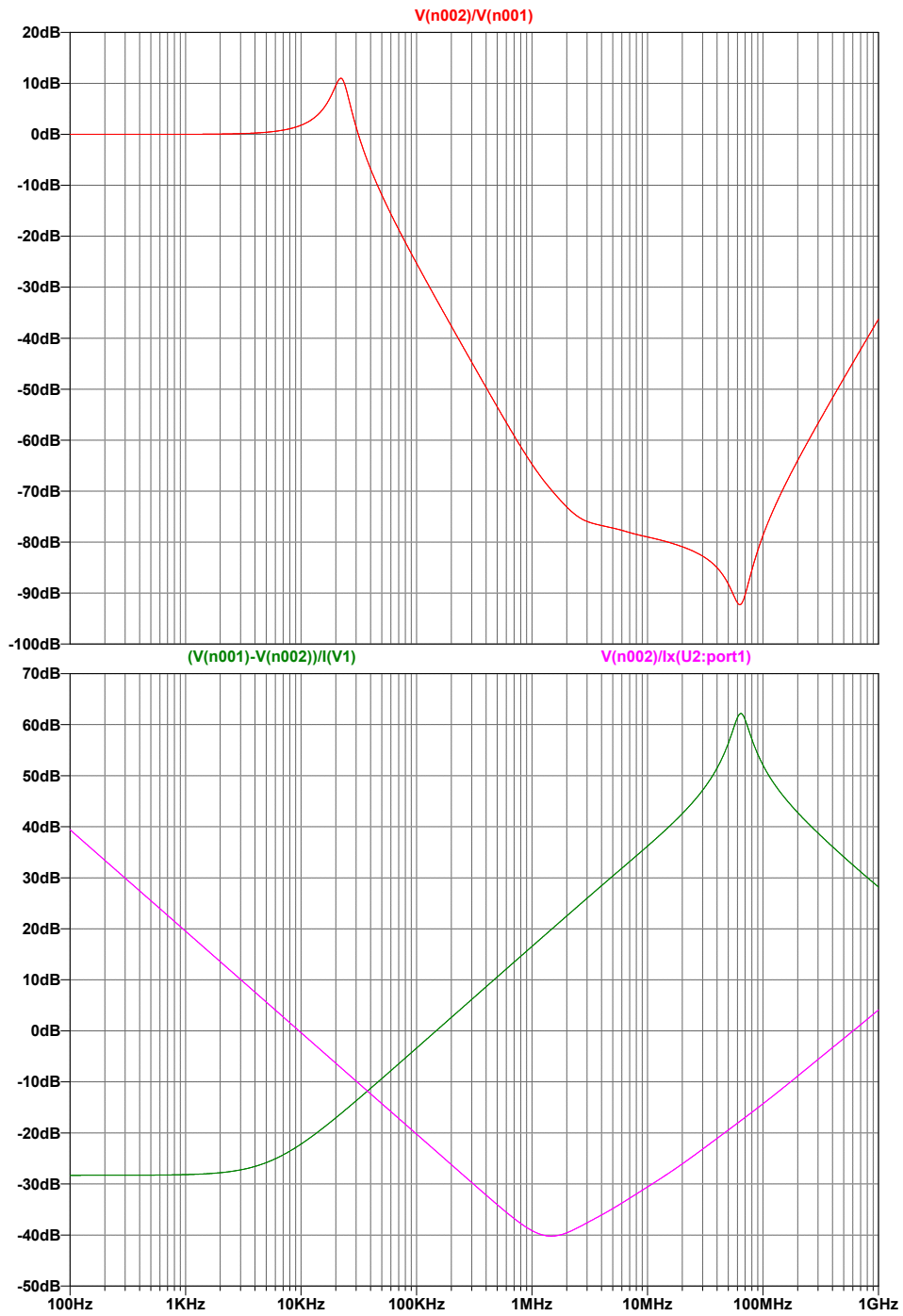
Figure 3.13: 3.3V rail filtering simulation with real components
