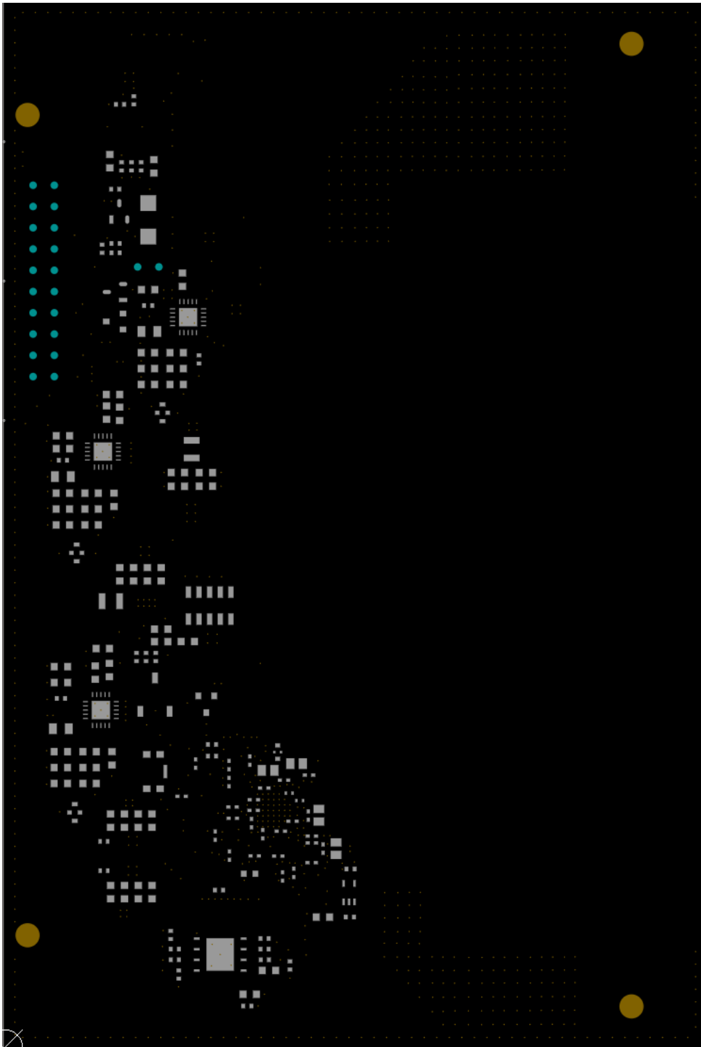
Figure B.10: Bottom paste mask layout
