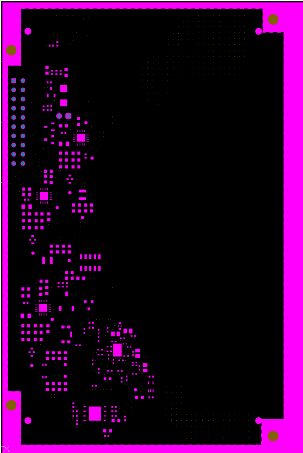
Figure B.8: Bottom solder mask layout
