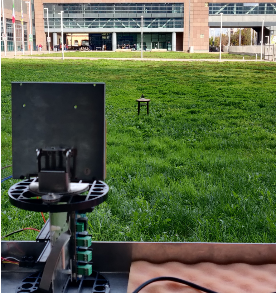
Figure 6.4: Setup used for the measurements, the test target is positioned 12 meters distant from the RADAR setup
