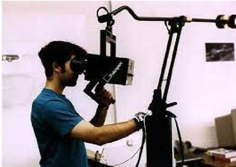
Figura 2.5: *BOOM (Binocular Omni-Orientation Monitor)*
