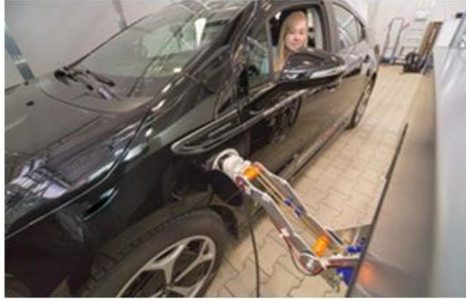
**Figure 1.5:** TU Dortmund solution to autonomous charging
