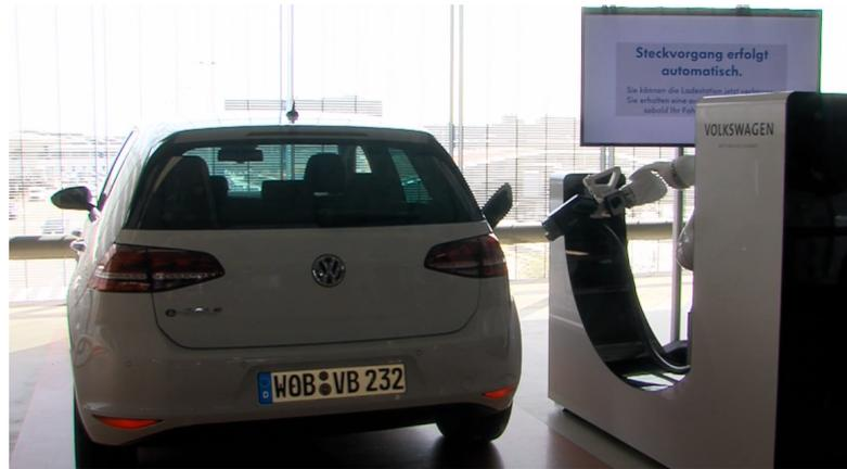
**Figure 1.3:** Volkswagen solution to autonomous charging
