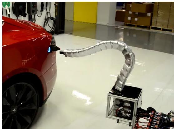
**Figure 1.4:** Tesla solution to autonomous charging
